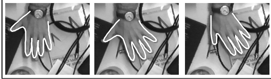
Fig. 7. Tracking a flexing hand across a cluttered desk. Representative stills from a 500 field (10 second) sequence of a hand moving over a highly cluttered desk scene. The fingers and thumb flex independently, and the hand translates and rotates. The distribution consists of N = 500 samples except for the first 4 fields, when it decreases from 1500 samples to aid initialisation. The distribution is initialised automatically by iterating on the motion model in the absence of measurements.
