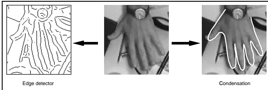
Fig. 8. Localising the hand in a dense edge map. Detail of a field from the hand sequence. The result of running a directional Gaussian edge detector shows that there are many clutter edges present to distract the system. The CONDENSATION algorithm succeeds in tracking the hand through this clutter.
