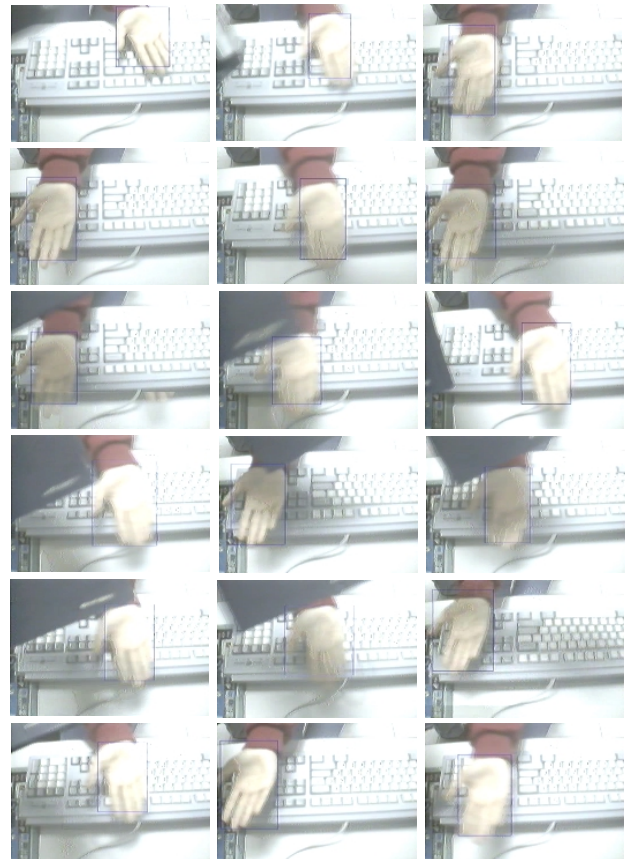
Figure 5: Results of localization with 18 frames taken from image sequences. A moving hand with interfering of a book is localized. The blue boxes are the bounding box of the interested color region.
