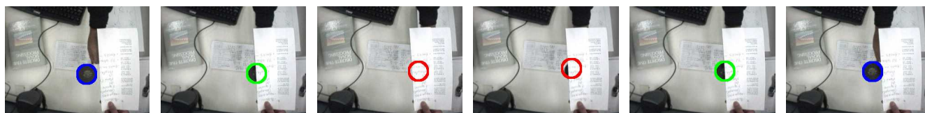
Figure 15: The tracker is able to tell if the target is tracked (in blue), partially occluded (in green), or lost (in red). (See eval.mpg )
