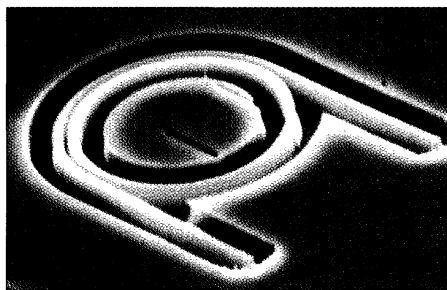
Ring of light. A ring laser just 9 microns across sends light into the surrounding waveguide.
