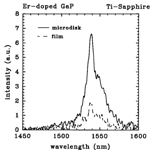
FIG. 3. Photoluminescence of an Er-doped GaP microdisk resonator given by the solid line, and the spectrum of an Er-doped GaP planar thin film sample given by the dashed line. Both measurements were obtained at the same peak pumping power and pumping intensity.
