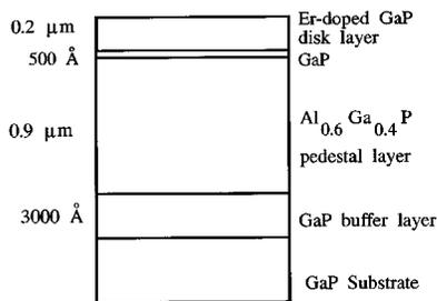
FIG. 1. The schematic of the Er-doped GaP microdisk layer structure, mainly consisting of an AlGaP pedestal layer and an Er-doped GaP disk layer.
