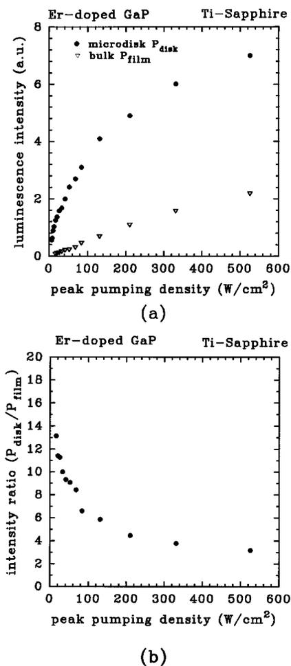
FIG. 4. (a) The emission power of the Er-doped GaP microdisk resonator  $P_{\text{disk}}$  (shown in solid circles) and the thin film sample  $P_{\text{film}}$  (shown in triangles) vs the pumping intensity, respectively. (b) The ratios between emission power of the Er-doped GaP microdisk resonator  $P_{\text{disk}}$  and the planar thin film sample  $P_{\text{film}}$  vs various pumping intensity.
