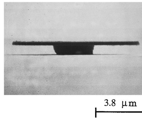
FIG. 2. The scanning electron microscope image of the side view of an Er-doped GaP microdisk resonator with 10 μm diameter.
