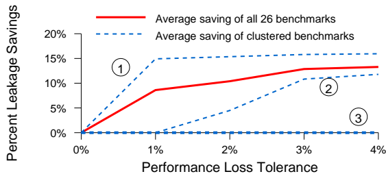
Figure 5: Static L1 Icache power savings versus unaware selective cache sets from the average of all 26 benchmarks and clustered benchmarks under k-means grouping.
