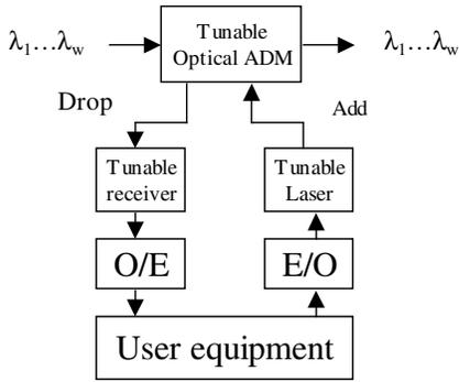
Fig. 1. An example node with tunable transceiver.
