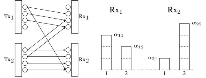
Fig. 2. At left is a deterministic interference channel. The more compact figure at right shows only the signals as observed at the receivers.
