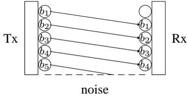
Fig. 1. The deterministic model for the point-to-point Gaussian channel. Each bit of the input occupies a signal level. Bits of lower significance are lost due to noise.
