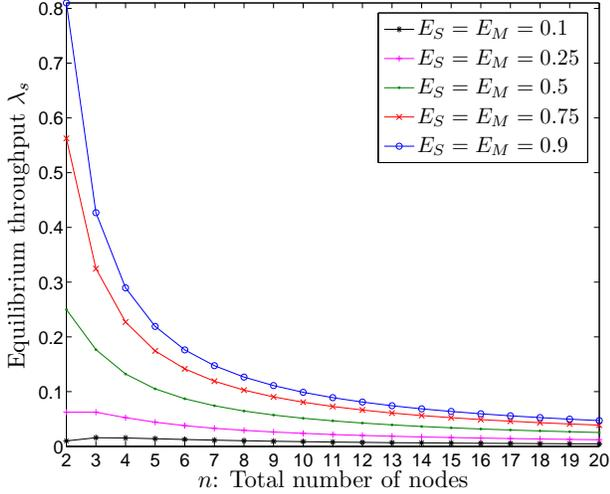
Fig. 7. The throughput  $\lambda_S$  achievable by one selfish node in Nash equilibrium as function of  $n$  for  $n_s = 1$ .
