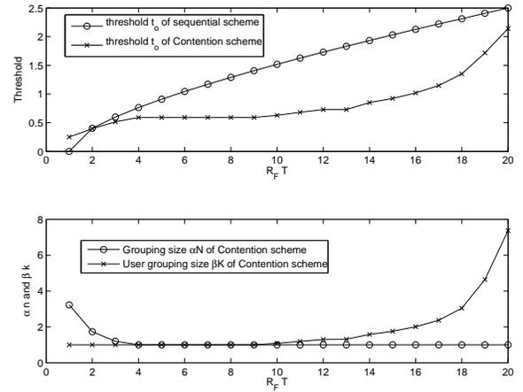
Fig. 4. Optimized parameters for each feedback scheme versus  $R_F T$ .
