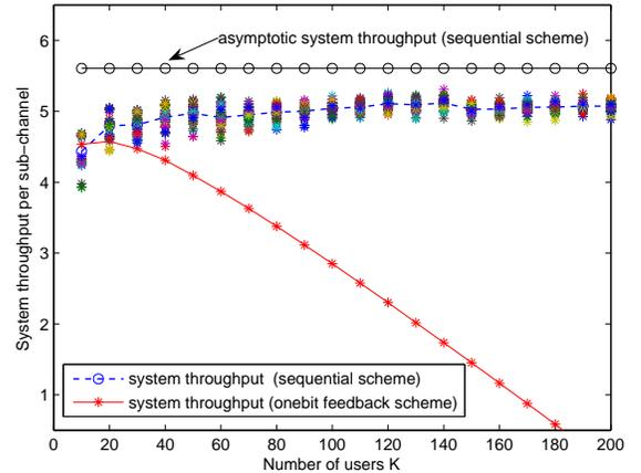
Fig. 6. Achievable rate per sub-channel for the sequential scheme as a function of  $K$  for  $\rho = 1$ . Also shown is the achievable rate for the one-bit feedback scheme presented in [6].
