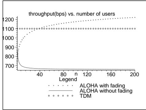
Figure 1: Comparison of throughput versus number of users with peak power constraint ( $P_m = 5W$ ,  $N_0W = 1$ ,  $W = 1000$  and  $h_0 = 1$ ).
