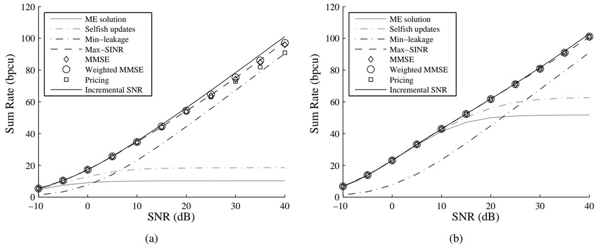
Fig. 3. Comparison of sum rate vs SNR for an interference network with  $K = 7$  users and  $N = M = 4$  antennas at each transmitter and receiver. The left and right plots correspond to strong and weak cross-channels, respectively. Results are averaged over 100 channel realizations.
