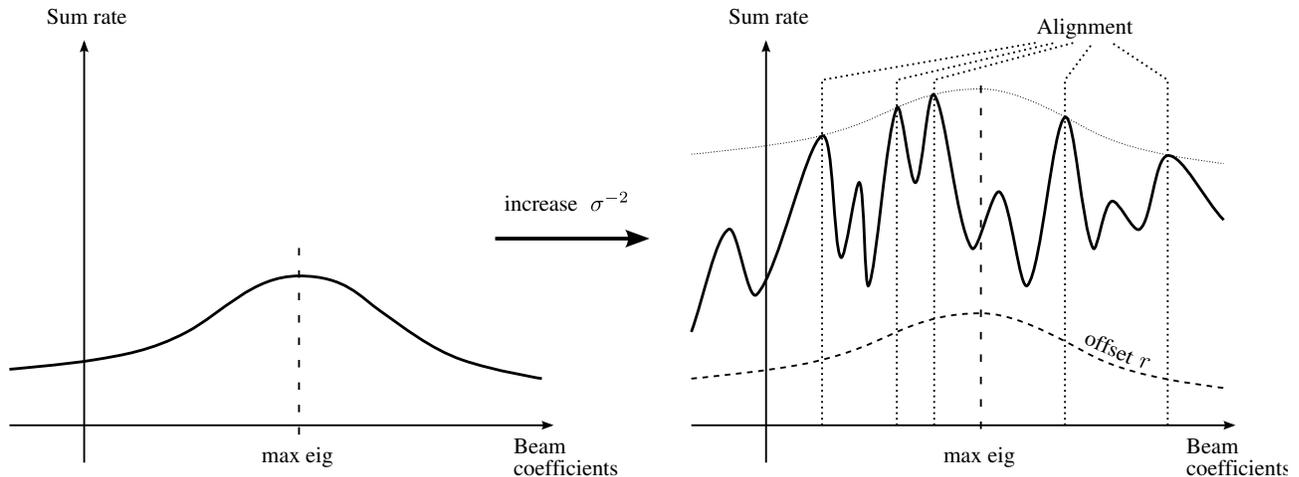
Fig. 2. For low SNR (left) the optimal beamformers are the principal eigenvectors of the Gramians of the direct channels. At high SNR (right), there are many local optimizers corresponding to ZF (aligned) solutions, which depend only on the cross channels.
