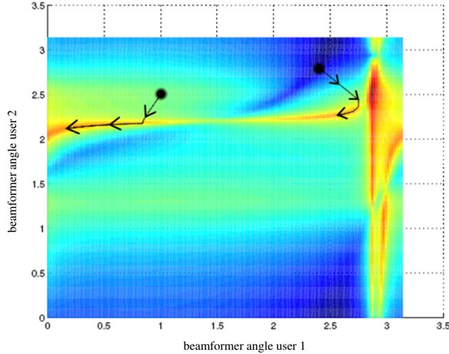
Fig. 1. Contour plot of sum rate for an example with three users,  $2 \times 2$  channels, and SNR 40 dB. The contours are in a two-dimensional subspace of the beam coefficients that contains the optimal (nearly aligned) solution shown in the upper right. Also shown are trajectories of a gradient algorithm from two different initial starting points. The end point corresponds to shutting off one of the users (determined by examining the resulting beamformers).
