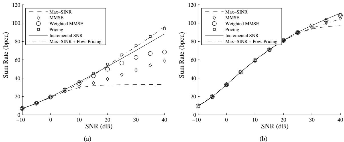
Fig. 4. Comparison of sum rate vs SNR for an interference network with  $K = 10$  users and  $N = M = 4$  antennas at each transmitter and receiver. The left and right plots correspond to strong and weak cross-channels, respectively. Results are averaged over 100 channel realizations.
