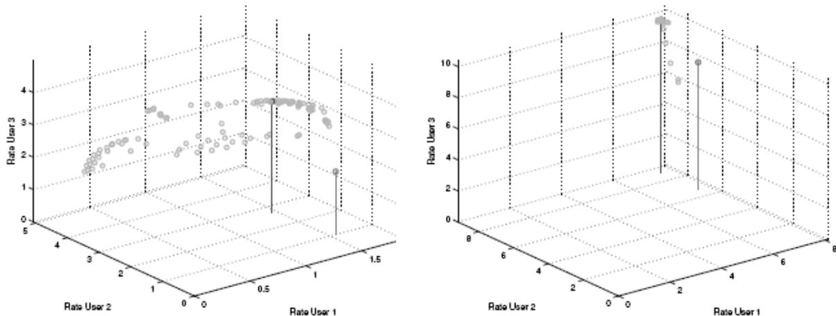
Fig. 6. Points in achievable rate region obtained by minimizing weighted sum MSE. Parameters are  $K = 3$ ,  $N = M = 2$ , and SNR equal to 10 dB (left) and 30 dB (right).
