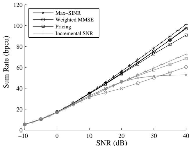
Fig. 5. Comparison of sum rates vs SNR with  $K = 7$  users,  $N = M = 4$  antennas, and strong cross-channels. Two sets of curves are shown corresponding to 100 iterations (shown as dark) and 20 iterations (shown as light). Results are averaged over 100 channel realizations.
