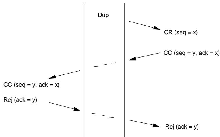
The client knows that it has already given up on starting a connection with seq=x. It may tell the server, so that the server does not hold on to false connection (or the server may simply time-out and close the connection.)
