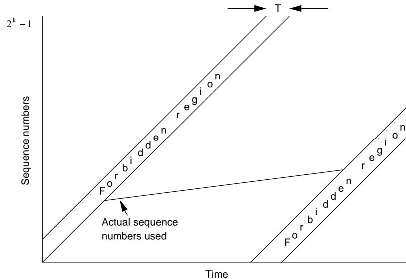
To avoid this, one solution is to resynchronize sequence numbers after a certain time. In TCP, 32 bit sequence numbers are used, and the clock increments every 4  $\mu$ sec. So wrap-around takes over 4 hours. Thus, this is not a major problem.
