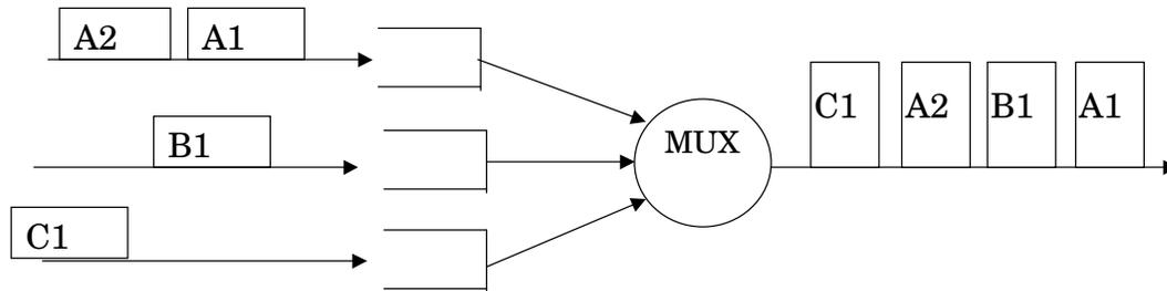
Statistical multiplexing is usually implemented at the packet level. Packets may have variable sizes or may all be a fixed size depending on the network. For example the Internet allows for variable packet sizes, while in ATM networks all packets have a fixed size of 53 bytes. The outgoing link may be synchronous and require each packet to be in a fixed slot, or it may be asynchronous allowing a packet to be sent at any time.
