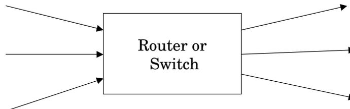
The transmission links in subnet usually carry traffic from several users. How this traffic is combined onto a link is referred to as **Multiplexing**. The reason for this is again primarily economic. In particular, transmission lines exhibit an **economy of scale**, what this means is that the cost per unit bandwidth for installing a transmission line is decreasing with the bandwidth.
