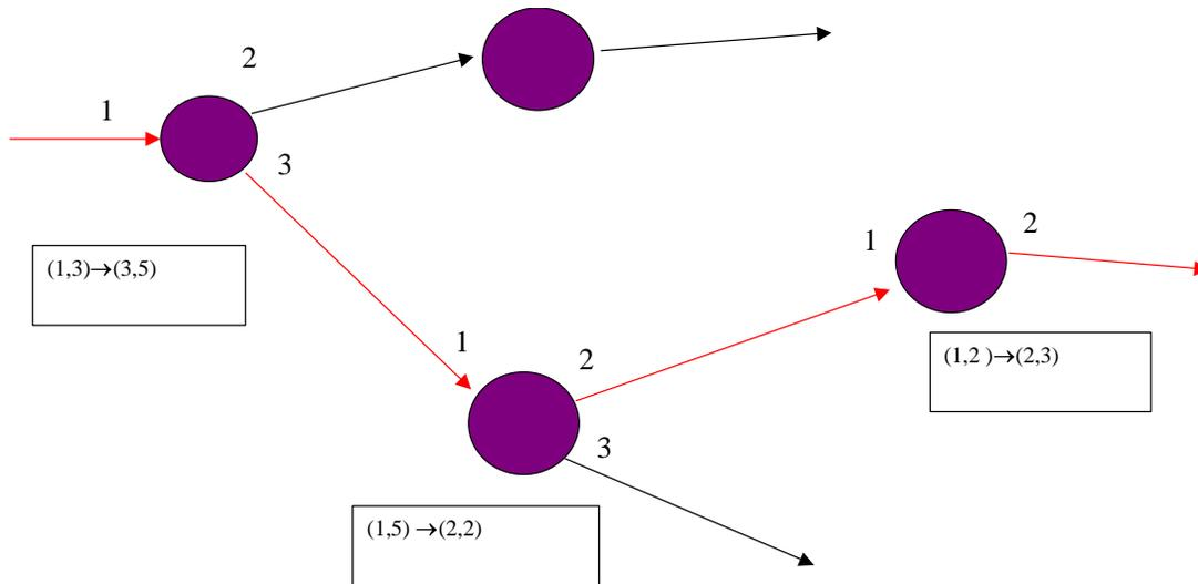
Each box shows the forwarding table entry for a connection along the path shown in red. The notation used is (incoming port, VCI)  $\rightarrow$  (outgoing port, VCI). Thus at the first switch, packets arriving with VCI 1, will be forwarded to port 3 and their VCI will be set to 5.
