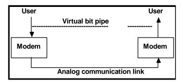
The modem/link/modem is **lower layer**; it provides a *service* to **higher layer** users.
