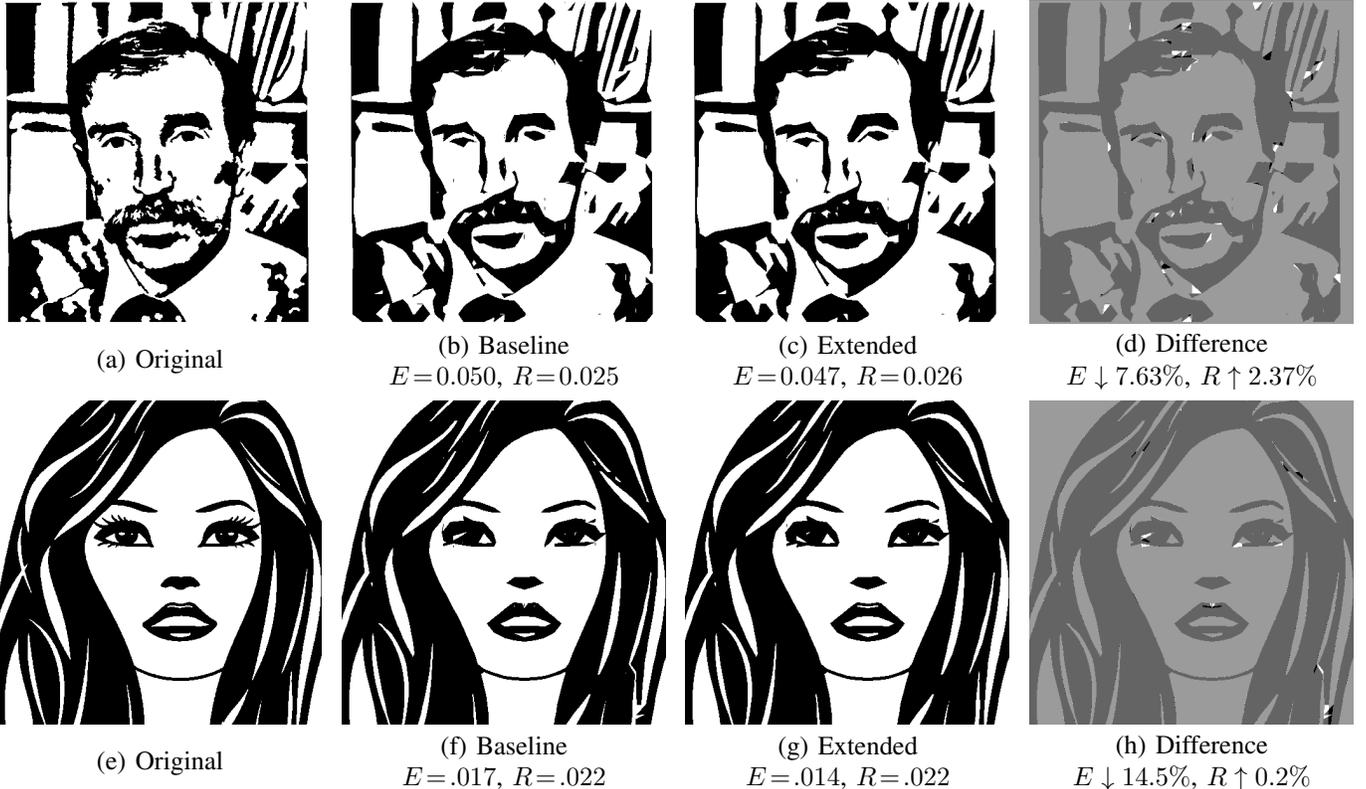
Fig. 13: Fixed-grid LCC with baseline and extended connection bits ( $N = 16$ ) and reconstruction difference
