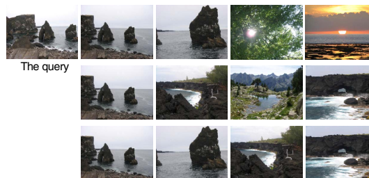
Figure 1. A sample query from the Holidays dataset: retrieval using a vocabulary tree of local features (first row); retrieval using 1000 semantic attributes (second row); retrieval based on co-indexing of both local features and semantic attributes (third row).
