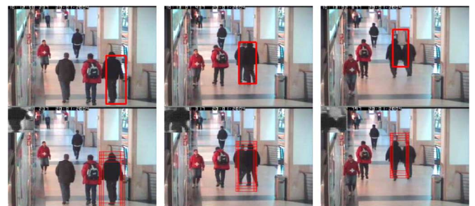
Fig. 13. Tracking a person with a camouflage object nearby [corridor]. (Top) our method; (bottom) the positive cluster.
