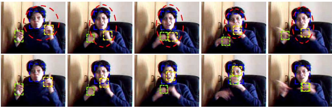
Figure 6.7. Tracking [sign language] for frame #1, 171, 172, 305, and 325, (1st row) game-theoretic MTT trackers and (2nd row) multiple independent trackers.
