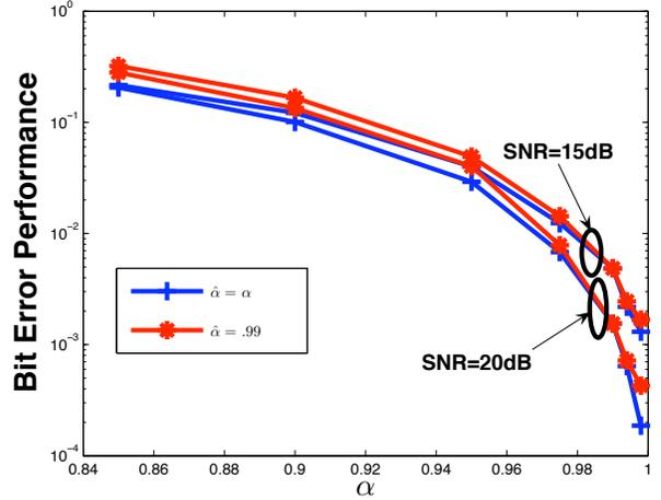
Fig. 5. Performance v.s. different values of  $\alpha$  with 3 dB weaker interference. For curves marked with “+”, the receiver uses the true value of correlation coefficient *i.e.*,  $\hat{\alpha} = \alpha$ . For curves marked with “\*”, receiver uses  $\hat{\alpha} = .99$  regardless of the value of  $\alpha$ .
