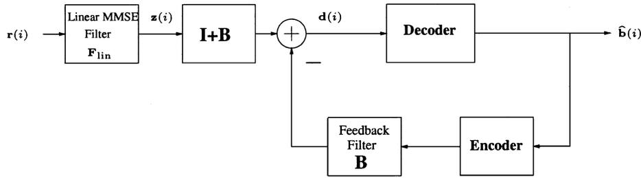
Fig. 8. Combined DFD with Viterbi algorithm for soft decoding.
