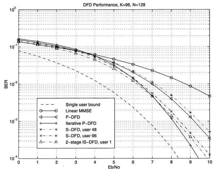
Fig. 6. Performance comparison of different receivers for synchronous CDMA with 96 users and  $N = 128$ .
