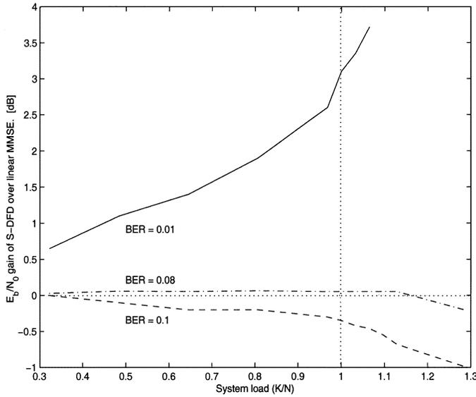
Fig. 7. Gain of the last detected S-DFD user relative to linear MMSE user with target BER as a parameter.
