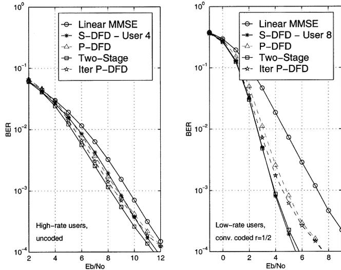
Fig. 10. Receiver performance with low- and high-rate users.
