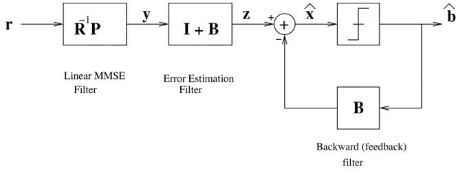
Fig. 2. Block diagram of optimal MMSE multiuser decision-feedback receiver.
