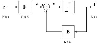
Fig. 1. Block diagram of multiuser decision-feedback receiver.
