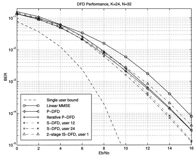
Fig. 5. Performance comparison of different receivers for synchronous CDMA with 24 users and  $N = 32$ .
