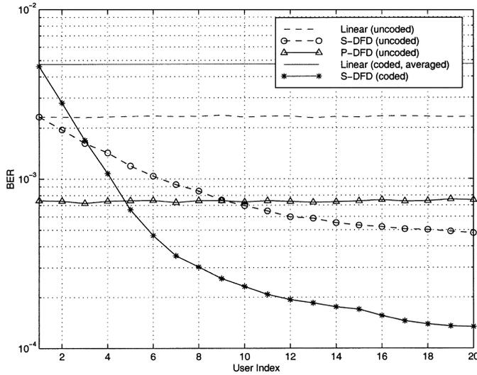
Fig. 9. Receiver performance with rate 3/4 convolutional code.
