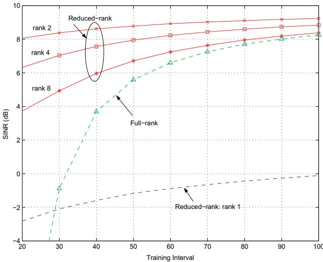
Fig. 3. Average SINR vs training with simultaneous group adaptation.
