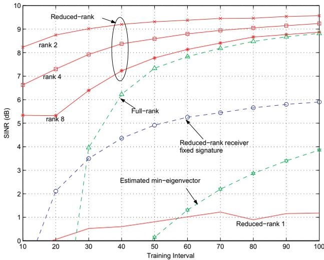
Fig. 1. SINR vs training interval for single-user joint signature-receiver adaptation.
