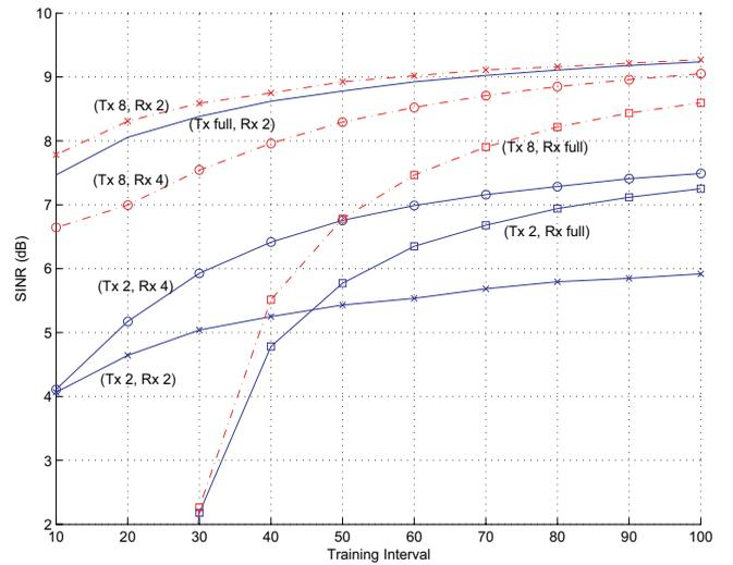
Fig. 4. Average SINR vs training for simultaneous group adaptation with reduced-rank signatures and reduced-rank receivers. (Tx  $a$ , Rx  $b$ ) indicates that the transmitter signature has rank  $a$  and the receiver has rank  $b$ .
