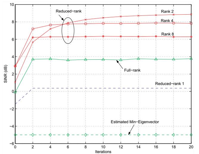
Fig. 2. SINR vs number of iterations with 30 training symbols.
