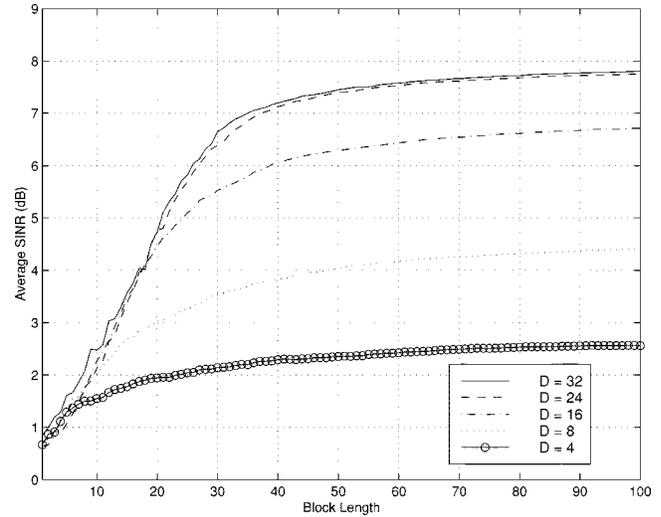
Fig. 5. Average SINR versus blocklength for single-user adaptation with nonadaptive, random interferers, and ideal channels.  $N = 32$ ,  $K = 24$ , and SNR = 8 dB.
