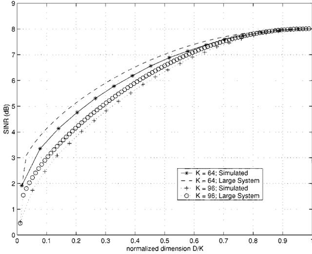
Fig. 3. Average SINR (dB) versus normalized dimension  $\bar{D}$  assuming only one user adapts.  $N = 128$  and SNR = 8 dB.
