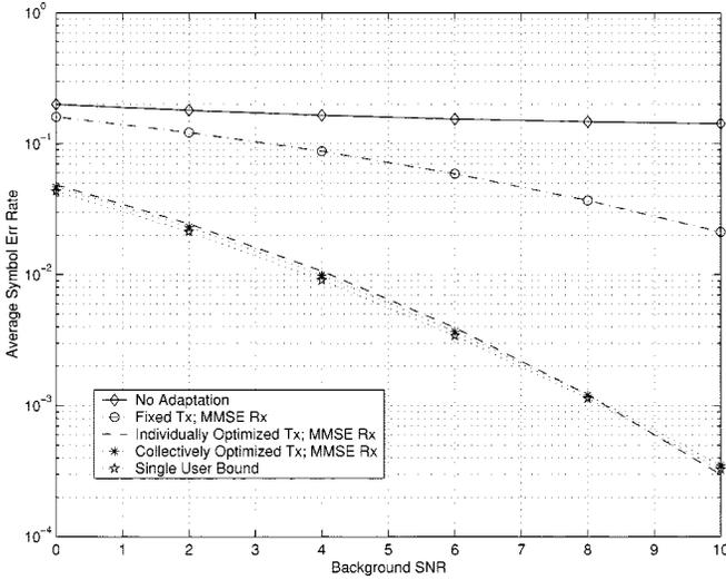
Fig. 9. Average symbol error rate versus background SNR with group optimization of signatures.  $N = 16$  and  $K = 12$ .
