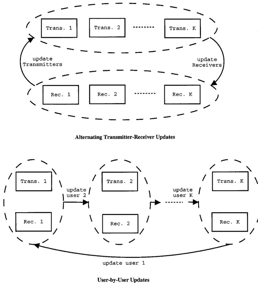
Fig. 2. Alternating transmitter-receiver versus user-by-user adaptation.
