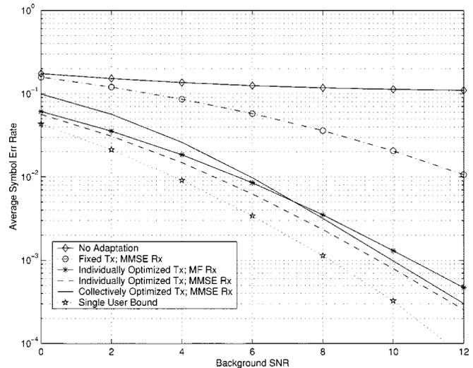
Fig. 8. Average symbol error rate versus background SNR for a single user with optimized signature in the presence of nonadaptive interference.  $N = 16$  and  $K = 12$ .
