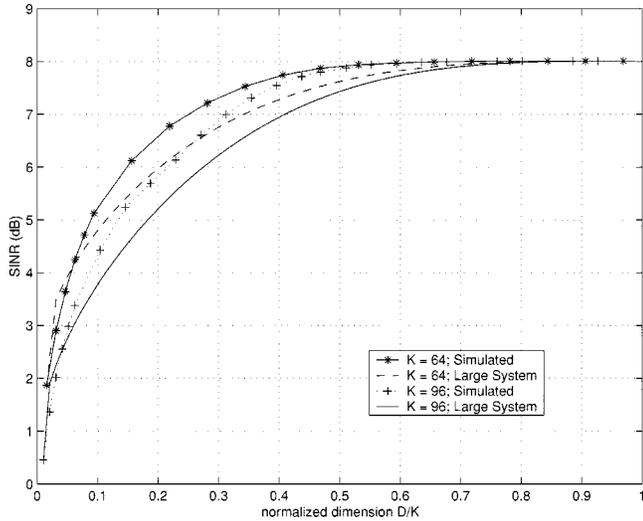
Fig. 4. Average SINR (dB) versus normalized dimension  $\bar{D}$  assuming all users adapt.  $N = 128$  and SNR = 8 dB.
