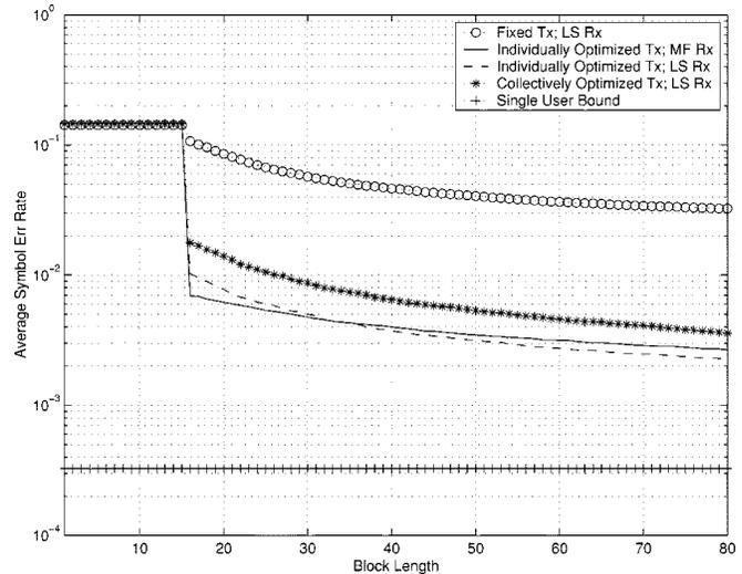
Fig. 7. Average symbol error rate versus blocklength (number of training samples) for single-user adaptation with nonadaptive interference.  $N = 16$ ,  $K = 12$ , and  $\text{SNR} = 10\text{dB}$ .
