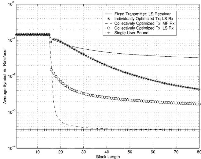
Fig. 6. Average symbol error rate versus blocklength (number of training samples) with group adaptation.  $N = 16$ ,  $K = 12$ , and  $\text{SNR} = 10\text{dB}$ .
