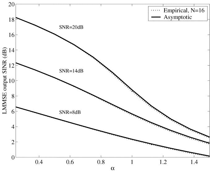
Fig. 7. Asymptotic and empirical SINR versus  $\alpha$  for multiuser multi-signature MC-CDMA.
