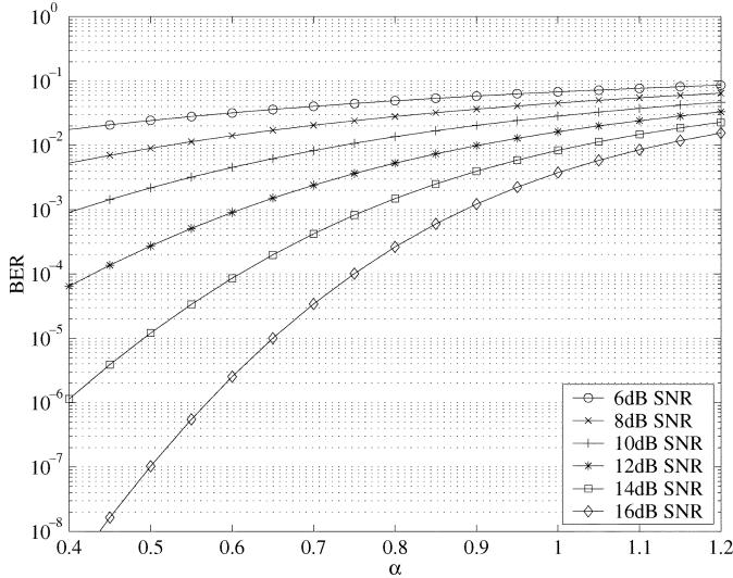
Fig. 3. Asymptotic and empirical BPSK BER for single-user multiple-signature MC-CDMA.
