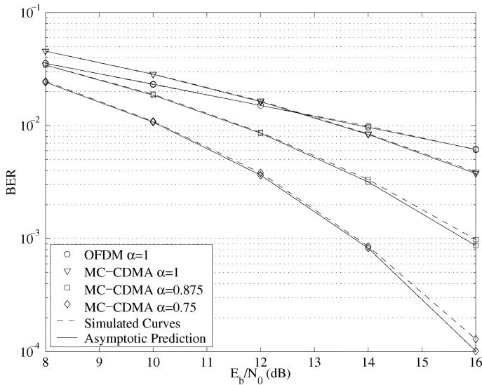
Fig. 2. Asymptotic and empirical BPSK BER for single-user multiple-signature MC-CDMA and OFDM with  $N = 16$ .
