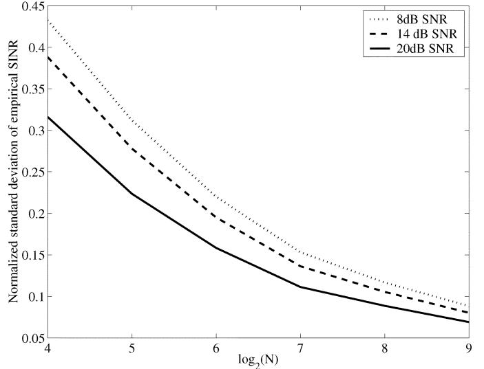
Fig. 1. Normalized standard deviation of single-user multiple-signature MC-CDMA empirical SINR for  $\alpha = 0.5$ .
