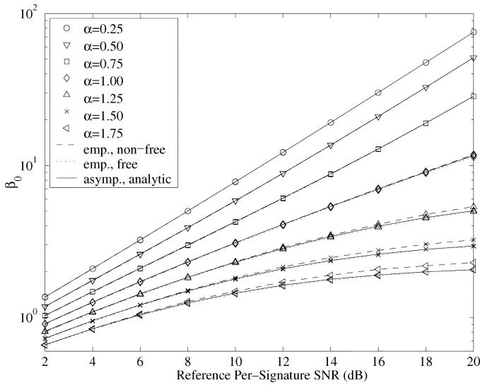
Fig. 6. Empirical and asymptotic values of  $\beta_0$ , and empirical values of  $\text{Tr}[\mathbf{R}^{-1}]$  versus per-signature SNR for a range of  $\alpha$  for two equal-power, equal-rate users.
