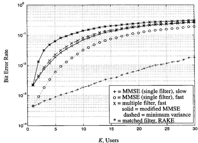
Fig. 4. Bit-error rate of the various MMSE receivers and the matched filter receiver with equal gain combining on a frequency-selective fading channel;  $E_b/N_0 = 15$  dB,  $N = 31$  (Gold codes), four-path (equal strength) Rayleigh fading channel, log-normally distributed interference power with 1.5-dB standard deviation.
