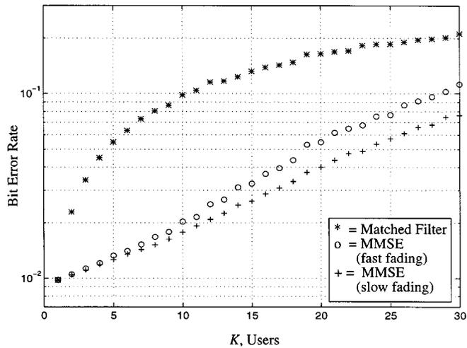
Fig. 2. Bit-error rate of the MMSE and MF on a flat fading channel;  $E_b/N_0 = 17$  dB,  $N = 31$  (Gold codes), Rayleigh fading channel, log-normally distributed interference power with 1.5-dB standard deviation.
