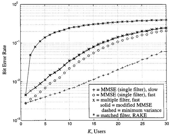
Fig. 5. Bit-error rate of the various MMSE receivers and the matched filter receiver with equal gain combining on a frequency-selective fading channel;  $E_b/N_0 = 15$  dB,  $N = 31$  (Gold codes), two-path (equal strength) Rayleigh fading channel, log-normally distributed interference power with 8-dB standard deviation.
