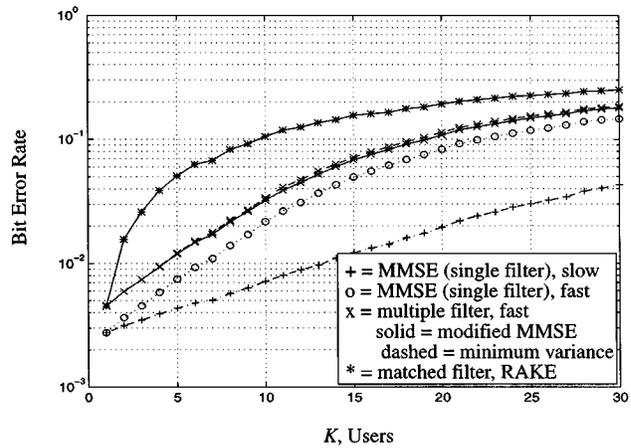
Fig. 3. Bit-error rate of the various MMSE receivers and the matched filter receiver with equal gain combining on a frequency-selective fading channel;  $E_b/N_0 = 15$  dB,  $N = 31$  (Gold codes), two-path (equal strength) Rayleigh fading channel, log-normally distributed interference power with 1.5-dB standard deviation.
