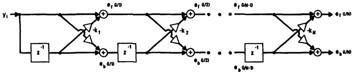
Fig. 1. Lattice structure.
