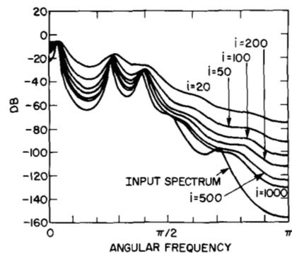
Fig. 7. Autoregressive spectral estimates versus time obtained from the LS lattice algorithm ( $w = 1.0$ ).
