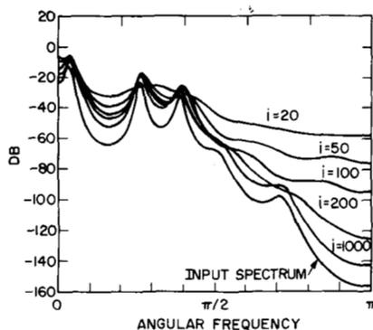
Fig. 5. Autoregressive spectral estimates versus time obtained from the SG lattice algorithm ( $w = 0.97$ ).
