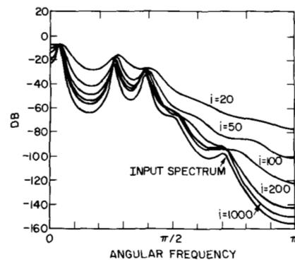
Fig. 6. Autoregressive spectral estimates versus time obtained from LS lattice algorithm ( $w = 0.97$ ).
