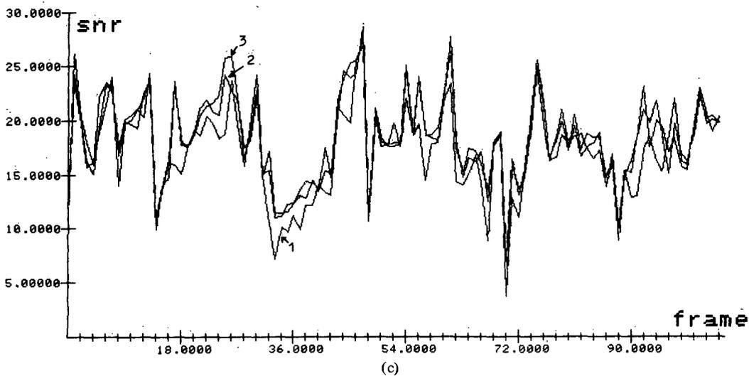
Fig. 7. (a) SNR obtained from using (curve 1) an LS lattice predictor and (curve 2) an LS lattice predictor plus pitch predictor for the phrase "Peter Pan peanut butter." (b) SNR obtained from using (curve 1) a fixed predictor and (curve 2) an LS lattice predictor for the phrase "Peter Pan peanut butter." (c) SNR obtained from using (curve 1) an LMS transversal predictor, (curve 2) an LMS lattice predictor, and (curve 3) an LS lattice predictor for the phrase "Peter Pan peanut butter."
