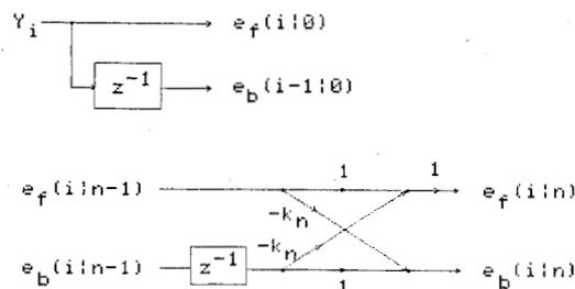
Fig. 1. Lattice filter structure.
