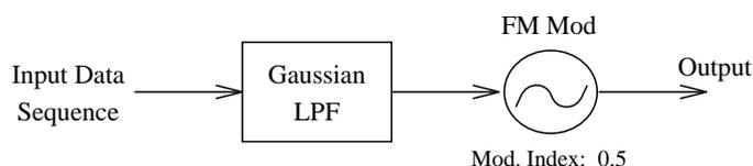
**Figure 13.** Generation of GMSK signal (LPF is Low-Pass Filter).
