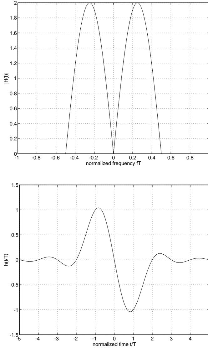
**Figure 10.** Modified duobinary frequency response and minimum bandwidth pulse.
