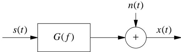
**Figure 1b.** Channel model consisting of a linear, time-invariant system (transfer function) followed by additive noise.
