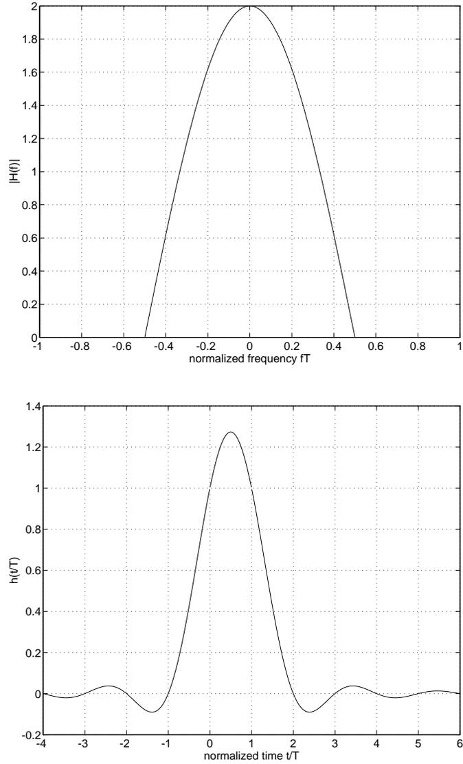
**Figure 9.** Duobinary frequency response and minimum bandwidth pulse.
