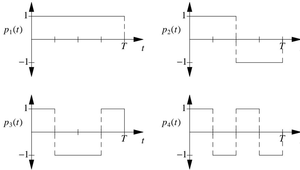
**Figure 2.** Four orthogonal spread-spectrum pulse shapes.
