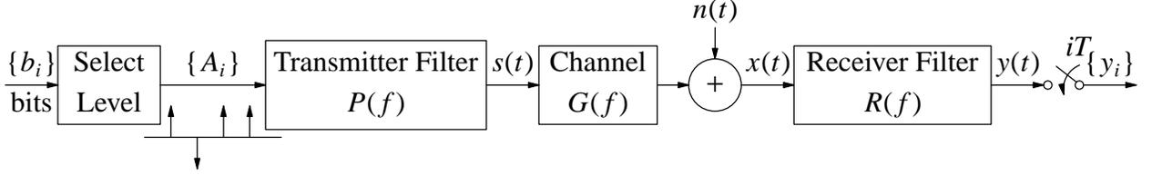
**Figure 3.** Baseband model of a Pulse Amplitude Modulation system.
