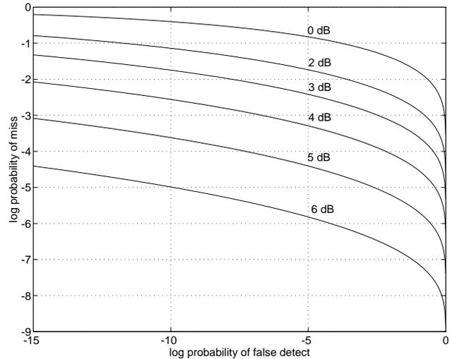
**Figure 2.**  $\log_{10} P_m$  vs.  $\log_{10} P_{fd}$  for the decision rule (5) assuming  $K = 1$ ,  $N = 10$ , and  $\text{SNR} = 15$  dB. Each plot corresponds to a different power level for the new interferer.
