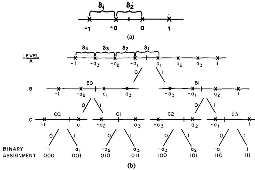
Fig. 2. (a) 4-AM constellation. (b) 8-AM constellation showing mapping of coded bits to levels by set-partitioning.
