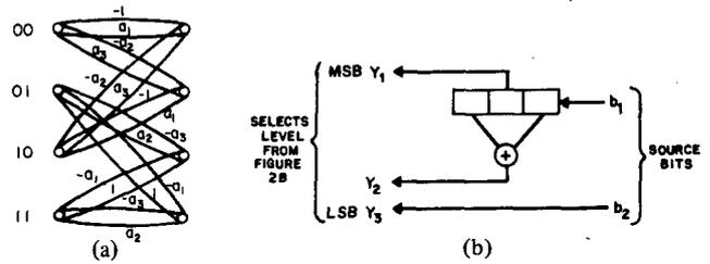
Fig. 1. Four-state, 8-AM trellis code. (a) Trellis diagram. (b) Convolutional code.
