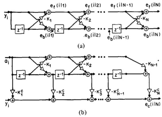
Fig. 4. (a) Lattice structure. (b) Echo canceller using the lattice structure.
