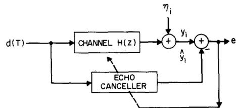
Fig. 2. Illustration of the channel estimation problem.
