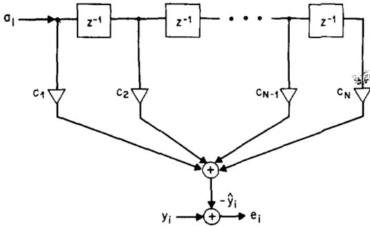
Fig. 3. Echo canceller using the transversal filter structure.
