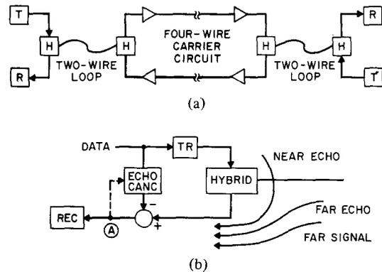
Fig. 1. (a) Typical dialed connection. (b) Use of data-driven echo canceller at station location. (Copied from [4].)
