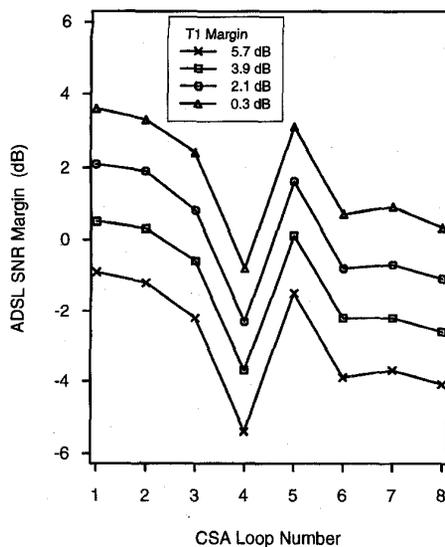
Fig. 4. ADSL performance margins on all 8 CSA loops with the optimized ADSL transmit spectrum. The T1 margins of 5.7, 3.9, 2.1, and 0.3 dB, correspond to those obtained when the proposed PSD mask (above 200 kHz) in [9] is set at  $-40$ ,  $-38$ ,  $-36$ , and  $-34$  dBm/Hz, respectively. The corresponding HDSL and ISDN BRA performance margins are the same as for Fig. 3. Data rate is 6.536 Mb/s.
