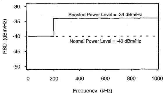
Fig. 1. The proposed ADSL transmit power PSD mask taken from [9].
