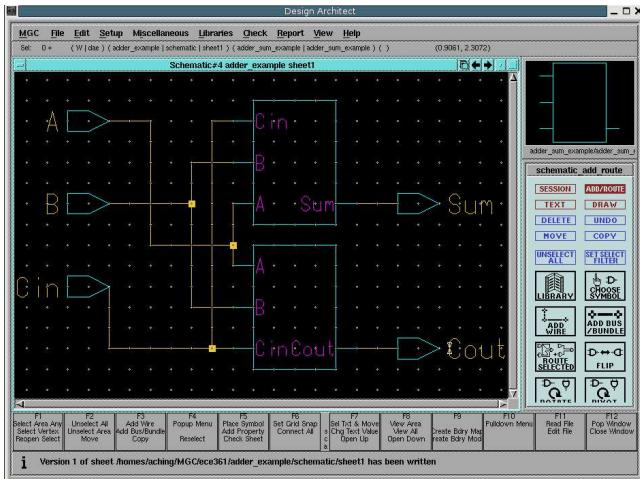
12. Now Check->Sheet and Check->Schematic before saving. Generate a symbol as we did in the past. Make sure to do all the proper checks after generating and saving a symbol and also after creating the symbol for the schematic. Close everything in design architect and then close design architect.
