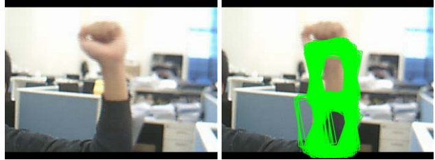
Figure 7. The left figure is the input frame, and the right figure shows the modes of two part-trackers. Two part-trackers handle the upper and lower arms, respectively. Each part-tracker generates 20~200 modes (shown in green rectangles) in one frame.
