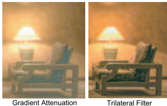
Figure 10: Nonuniform gradient compression 12 can sometimes lead to brightness anomalies. Image courtesy of Shree Nayar, Columbia University.
