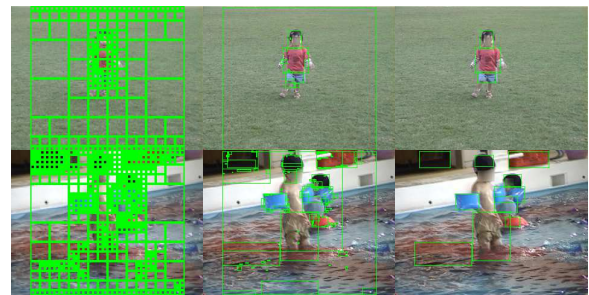
Fig. 3. Illustration of the quad-tree color segmentation. (left) input frame, (middle) over-segmentation, (right) pruned segmentation.
