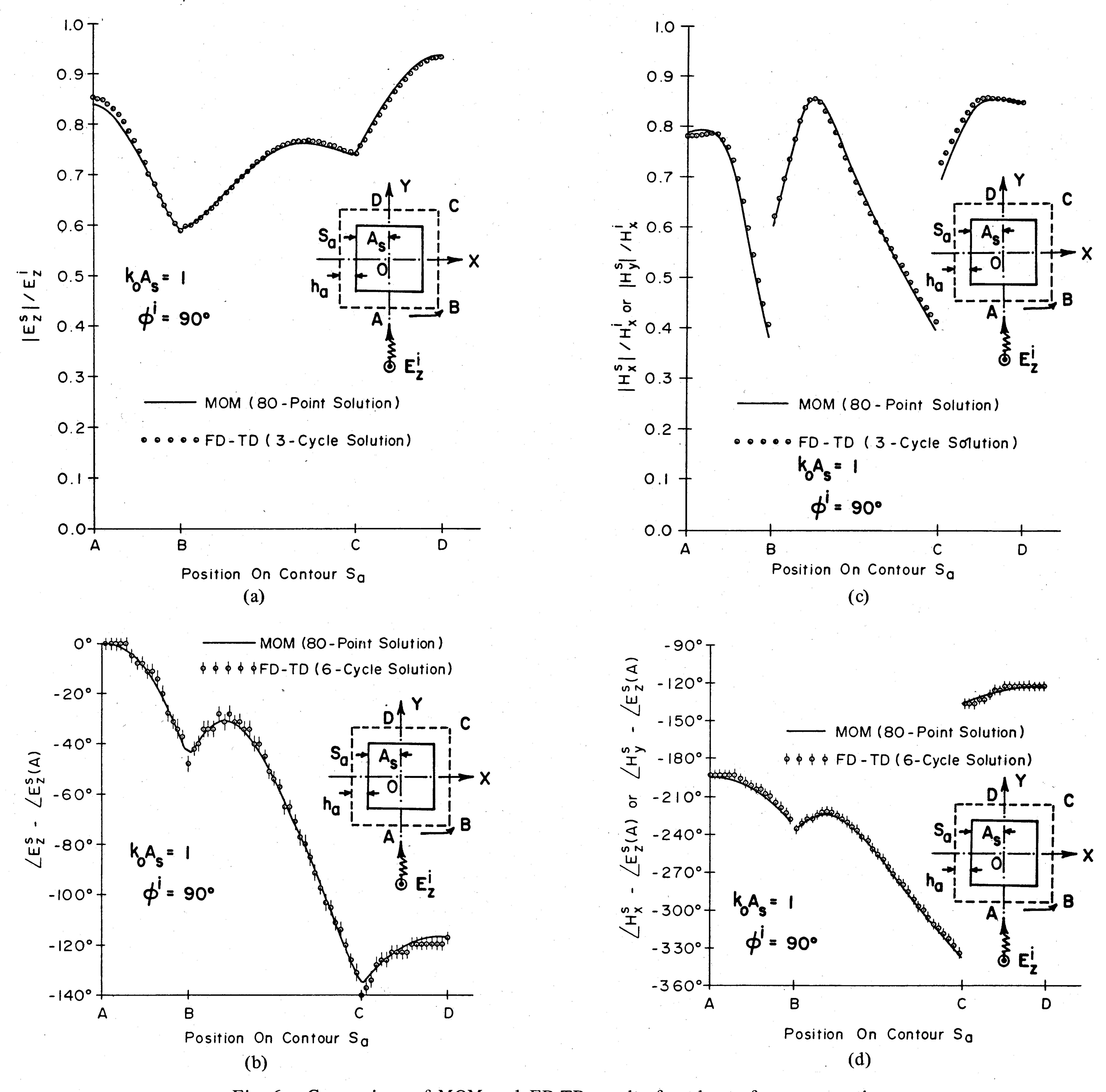
Fig. 6. Comparison of MOM and FD-TD results for phase of near magnetic tangential to contour  $S_a$ .
