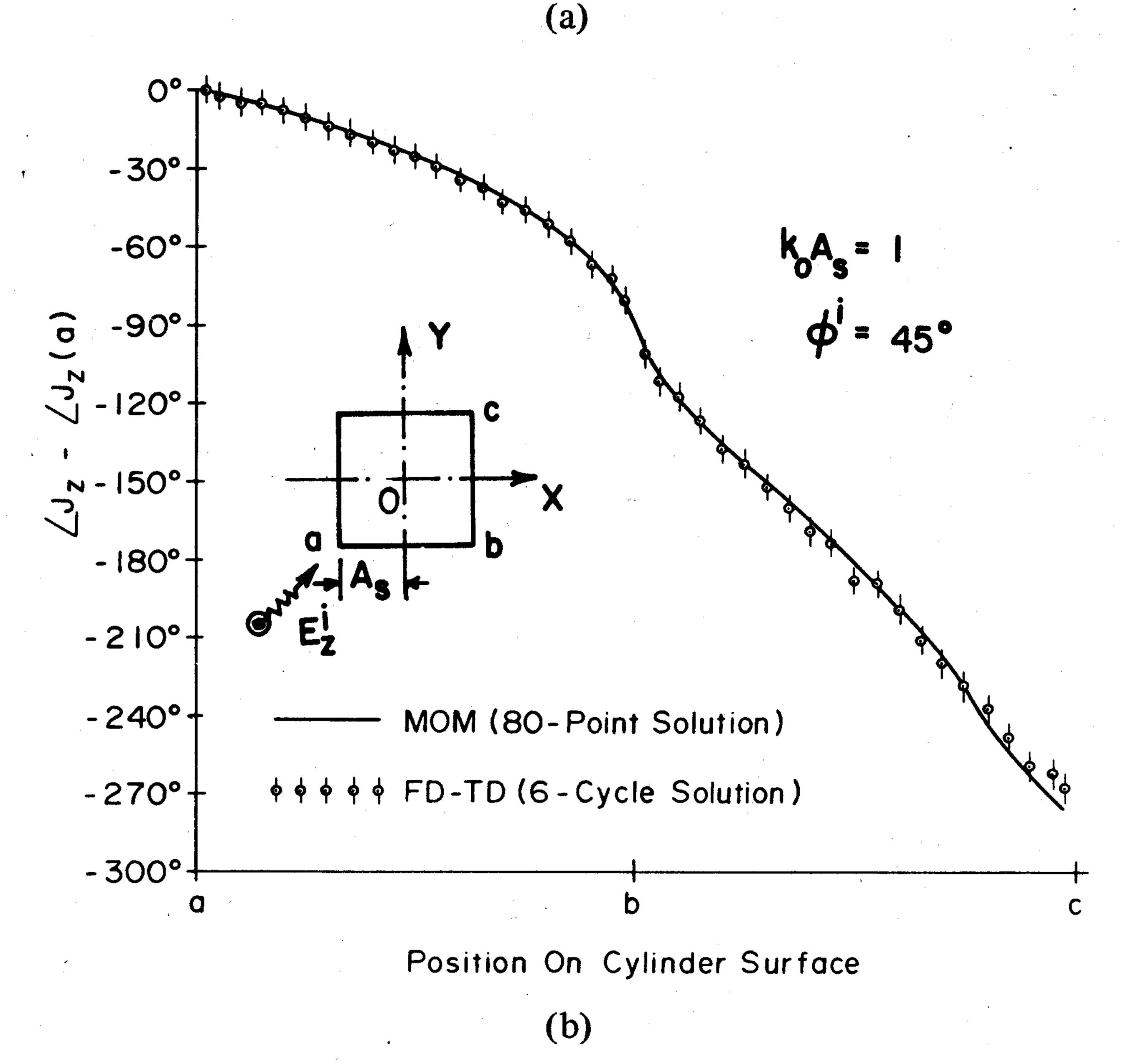
Fig. 8. Comparison of MOM and FD-TD results for (a) magnitude of electric currents on surface of cylinder oblique-incidence case ( $\phi^i = 45^\circ$ ) and (b) phase of electric currents on surface of cylinder oblique-incidence case ( $\phi^i = 45^\circ$ ).
