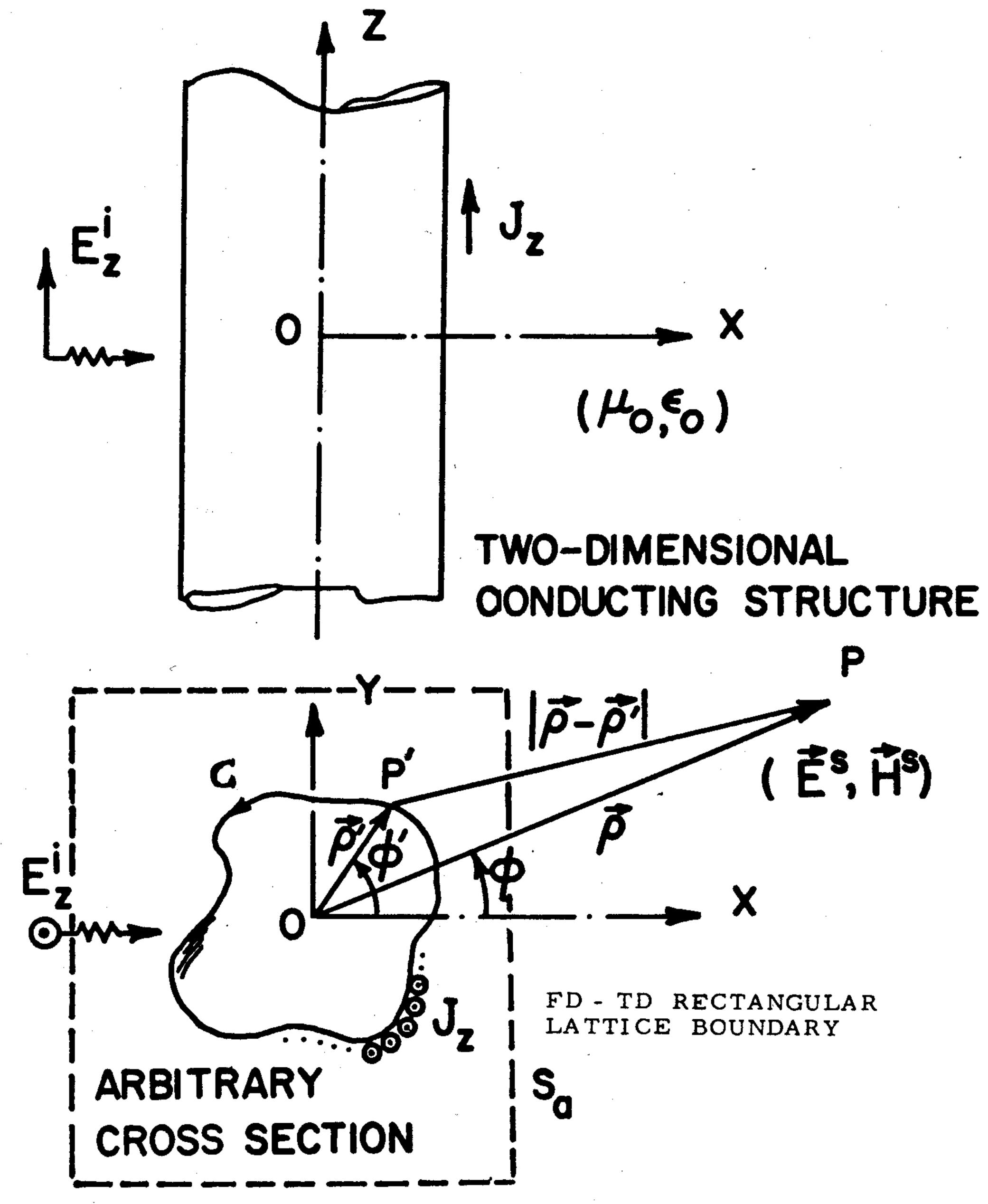
Fig. 4. Geometry of a TM-excited conducting cylinder.
