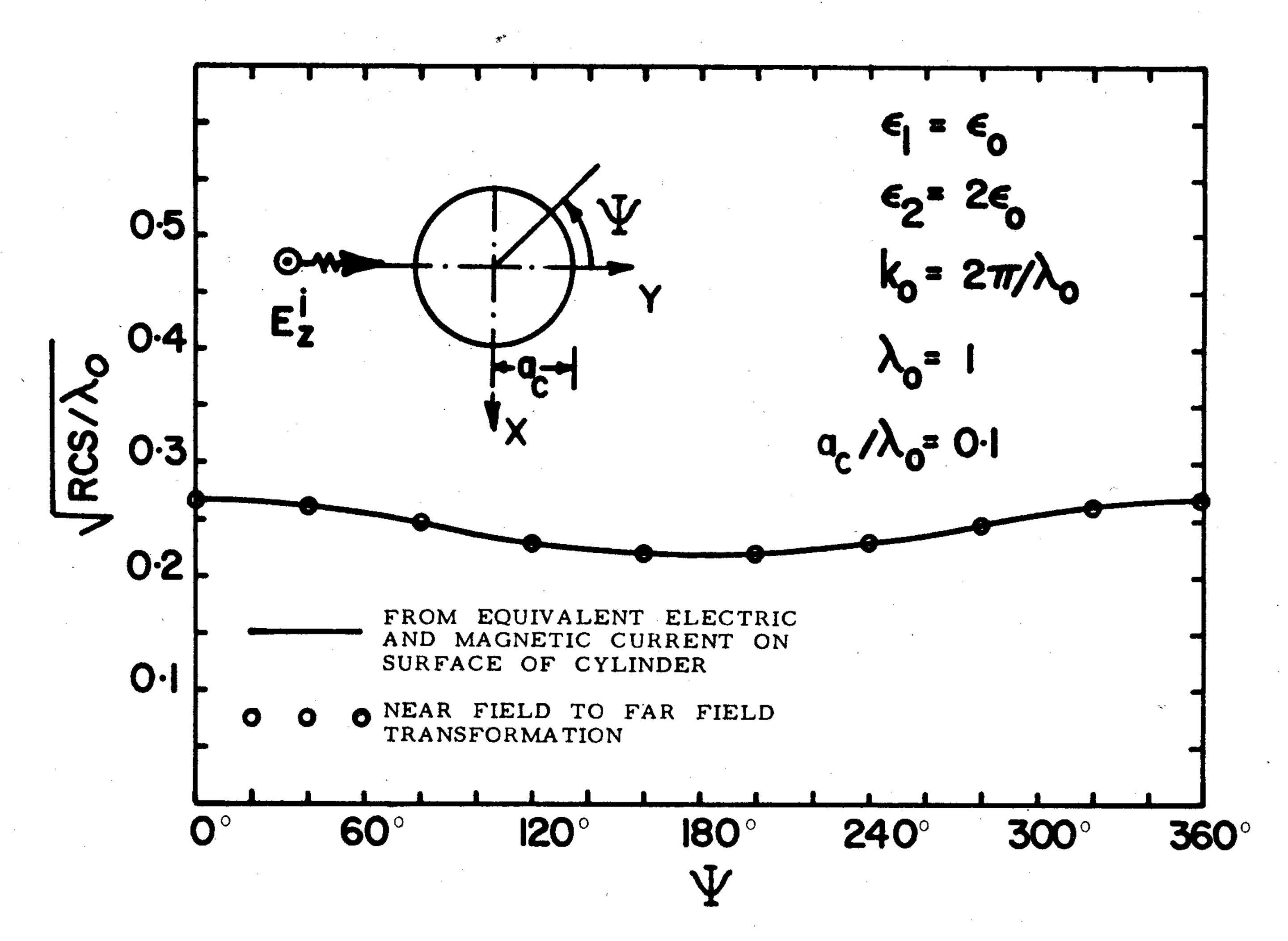
Fig. 10. Scattering cross section of the dielectric circular cylinder.
