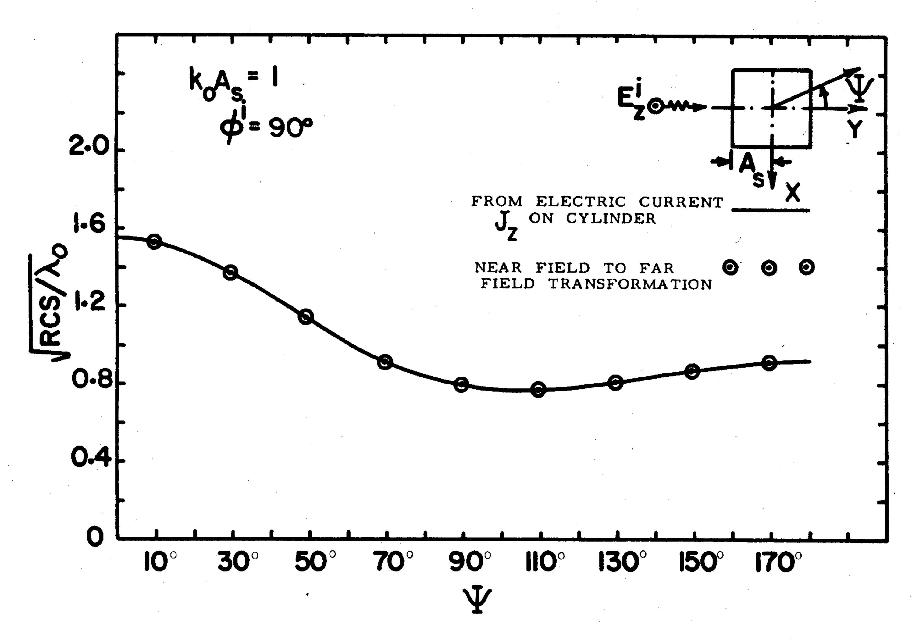
Fig. 7. Scattering cross section of the conducting square cylinder.
