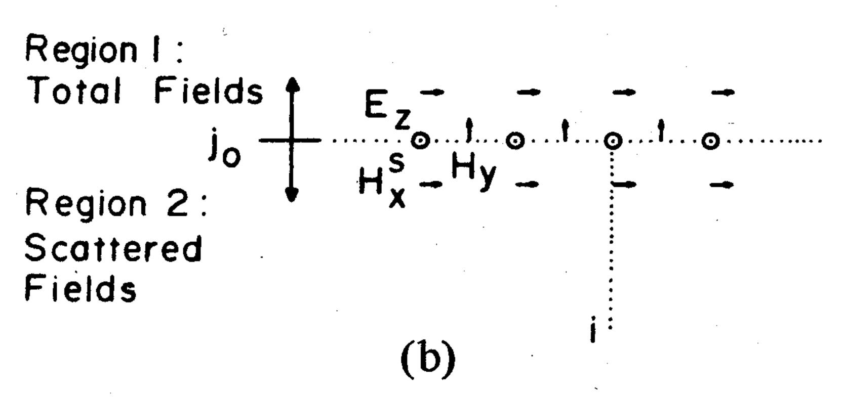
Fig. 2. Division of FD-TD lattice into total-field and scattered-field regions. (a) Lattice division. (b) Typical connecting conditions between regions.
