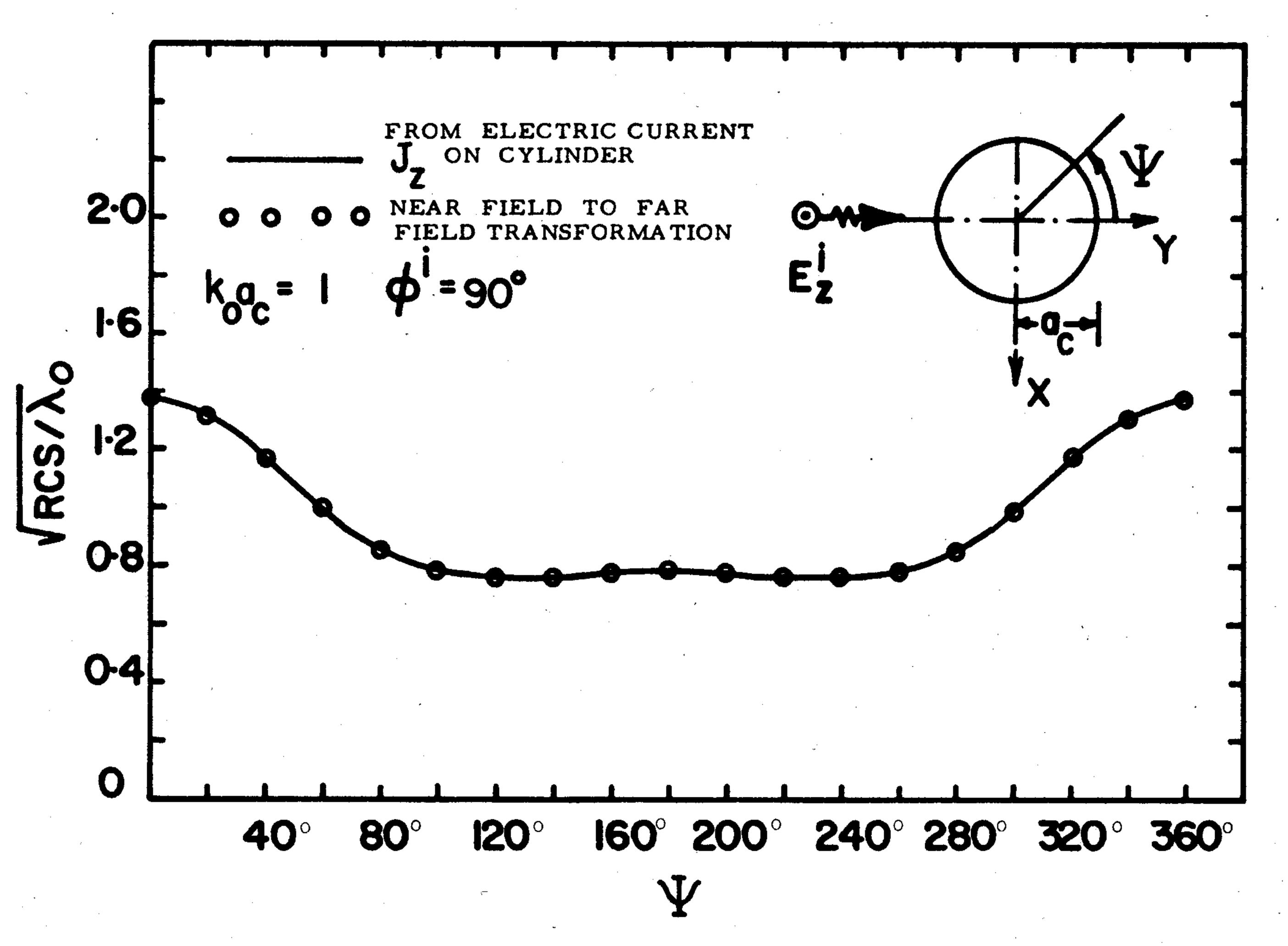
Fig. 9. Scattering cross section of the conducting circular cylinder.
