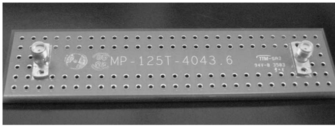
Fig. 3. Test structure comprised of FR4 circuit board (relative permittivity = 4.3 and loss tangent = 0.017) with the transmit and receive probes (50- \Omega nominal source and load impedances) bonded to the opposing ground plane. This structure spans 10 cm between the input and output probes; 3.2 mm between the upper and lower ground planes; and 13.8 mm (center-to-center) between the rows of vias immediately bounding the waveguiding defect. The radius and spacing of the vias are r = 0.83 mm and a = 4.6 mm, respectively.
