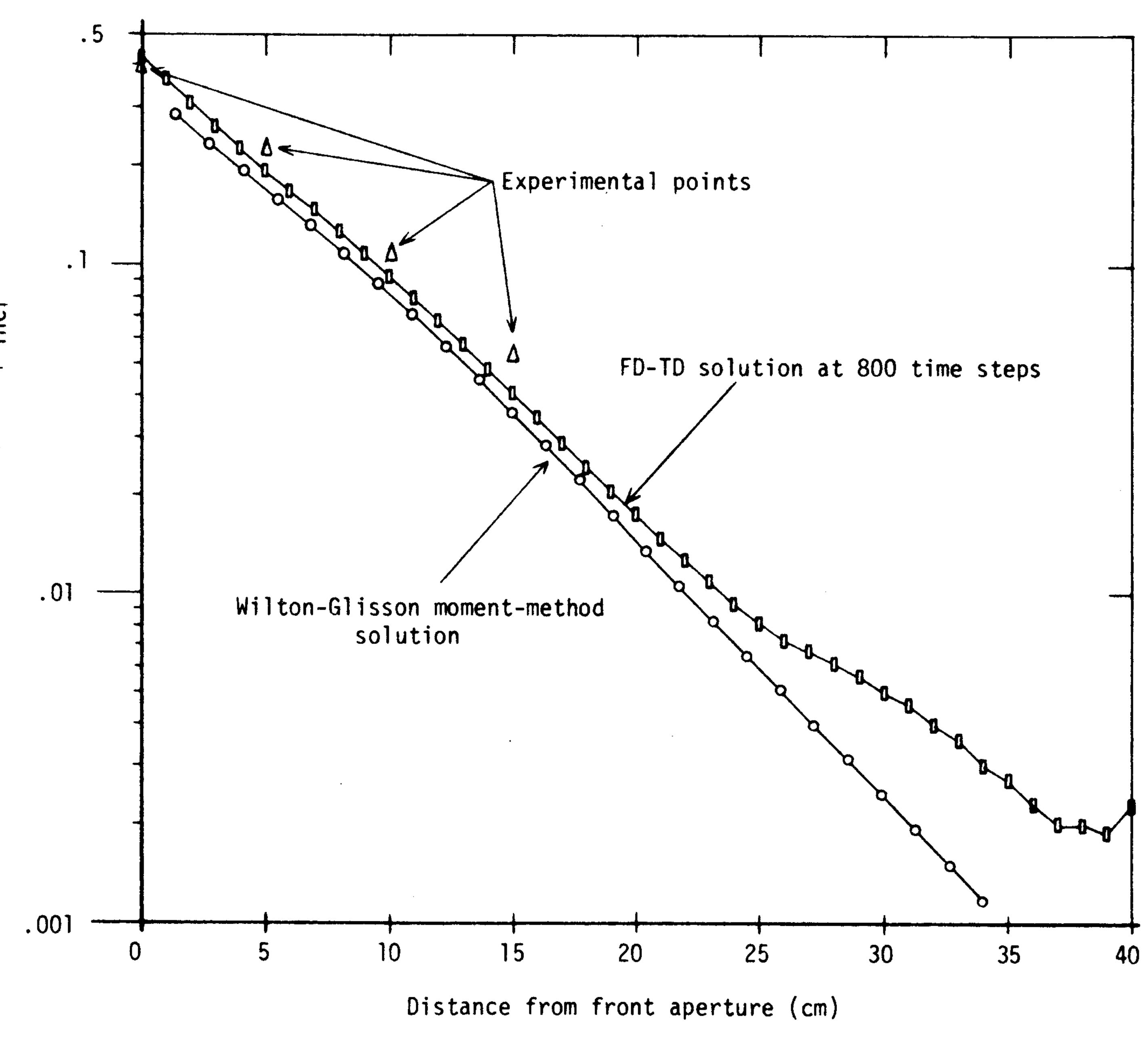
Fig. 7. Comparison of results for the electric field along the cylinder axis.
