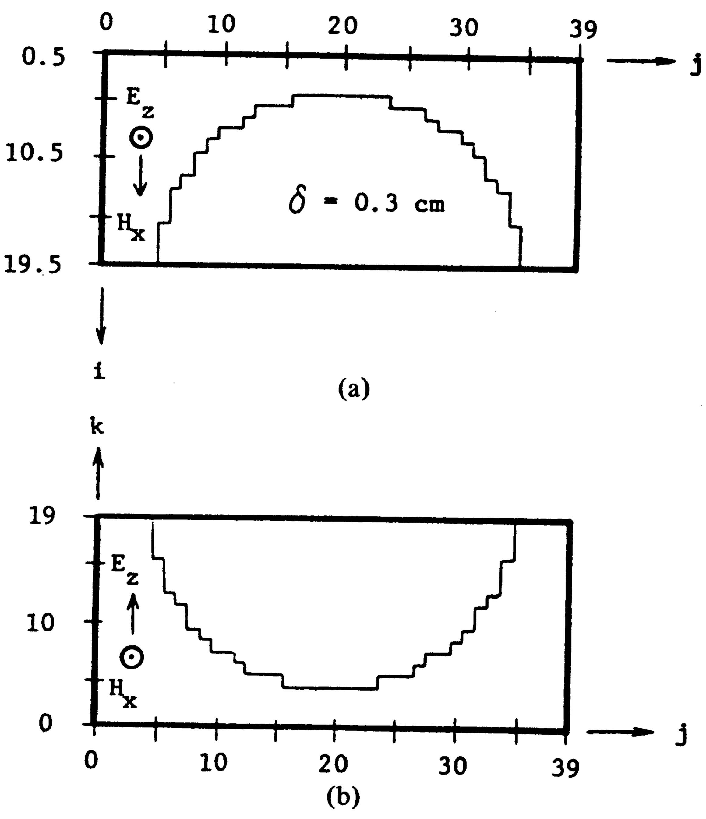
Fig. 2. FD-TD model geometry of a 9.0-cm diameter dielectric sphere. (a) Symmetry plane k = 19. (b) Symmetry plane i = 19.5.
