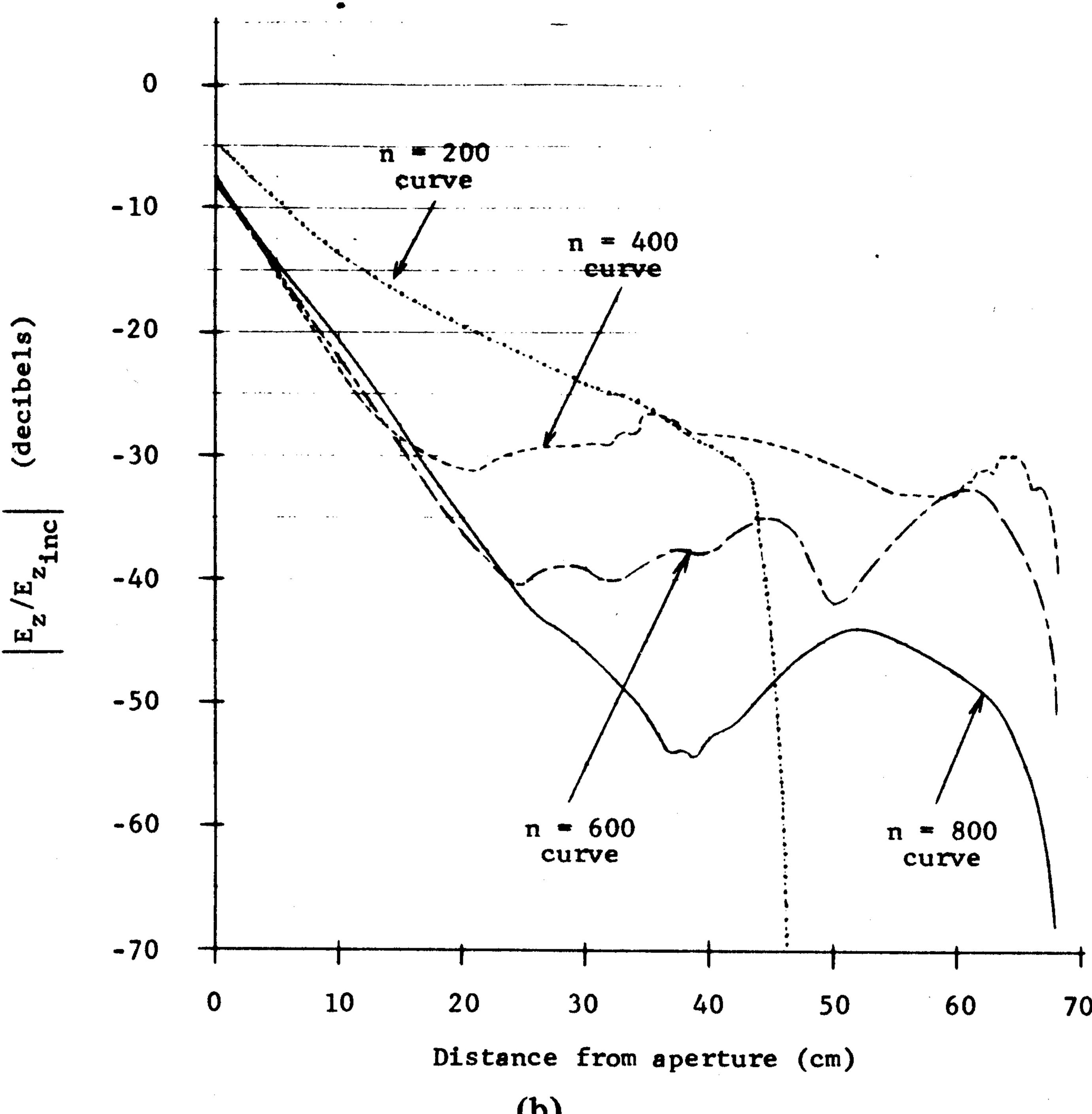
Fig. 6. Convergence of the FD-TD computed electric field along the cylinder axis. (a)  $\sigma_{int} = 0$  case. (b)  $\sigma_{int} = 0.01$ -mho/m case.
