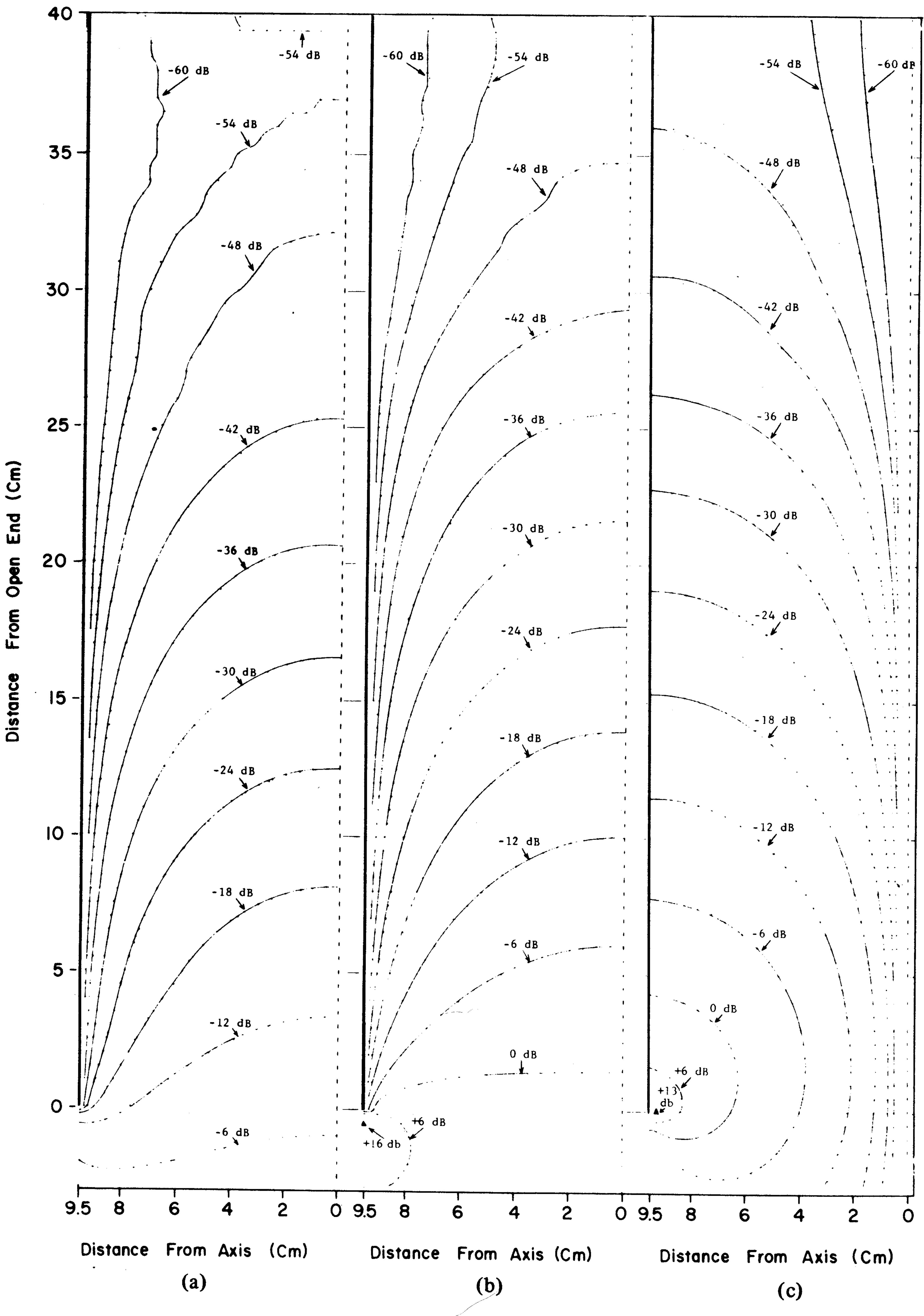
Fig. 9. FD-TD computed field contours in the horizontal symmetry plane of the cylinder. (a)  $E_z$ . (b)  $H_x$ . (c)  $H_y$ .
