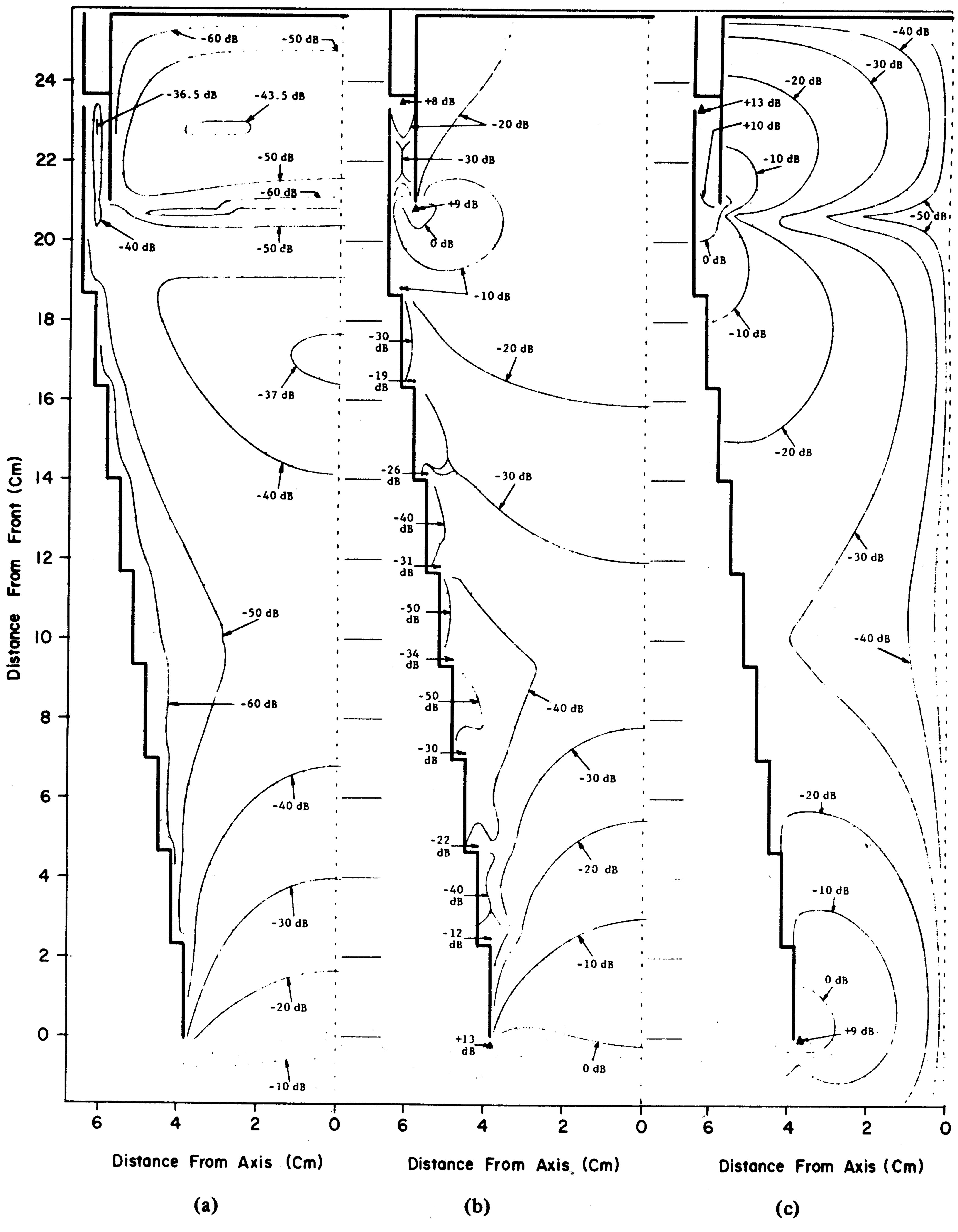
Fig. 13. FD-TD computed field contours in the horizontal symmetry plane of the nose cone. (a)  $E_z$ . (b)  $H_x$ . (c)  $H_y$ .
