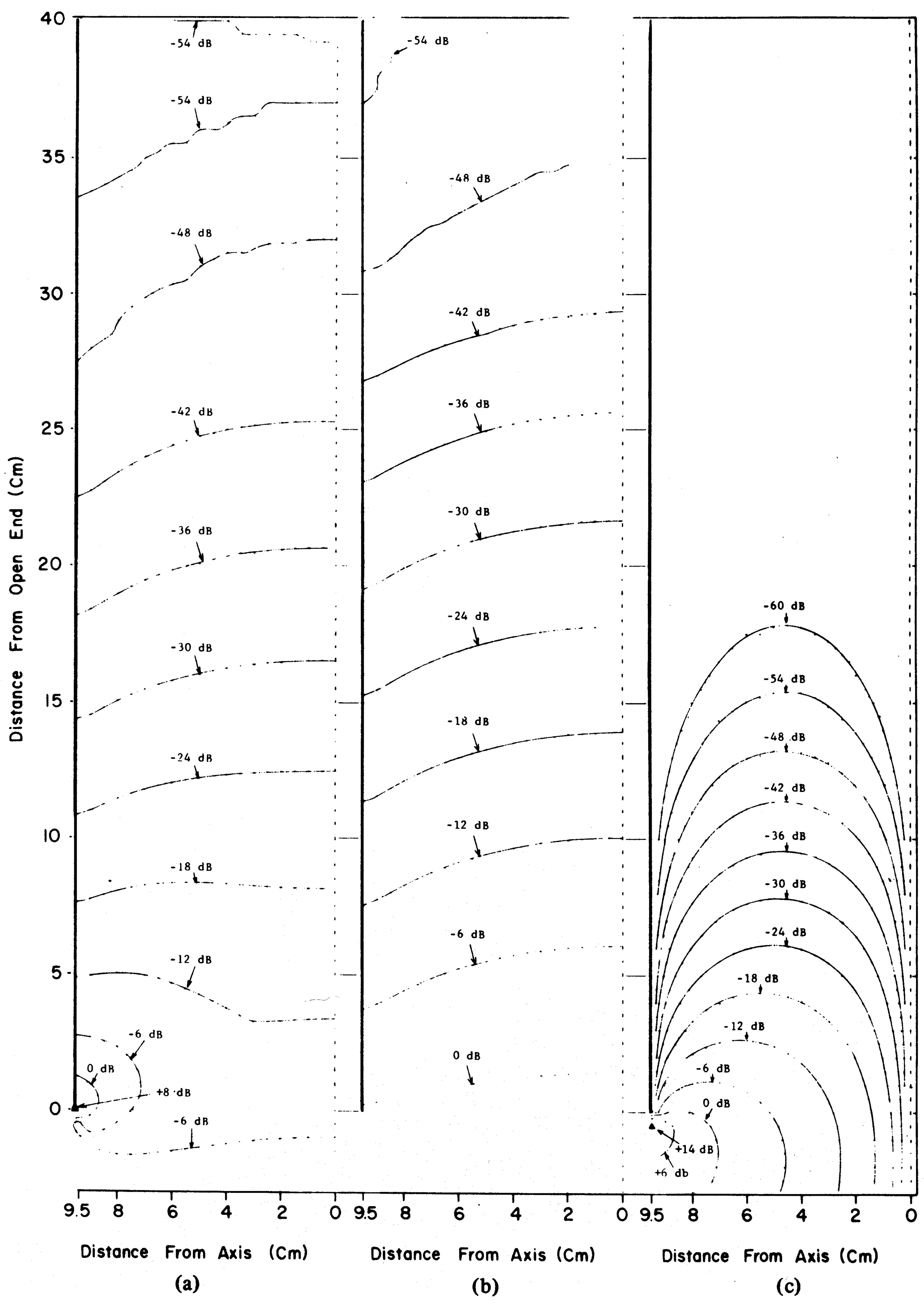
Fig. 8. FD-TD computed field contours in the vertical symmetry plane of the cylinder. (a)  $E_z$ . (b)  $H_x$ . (c)  $E_y$ .
