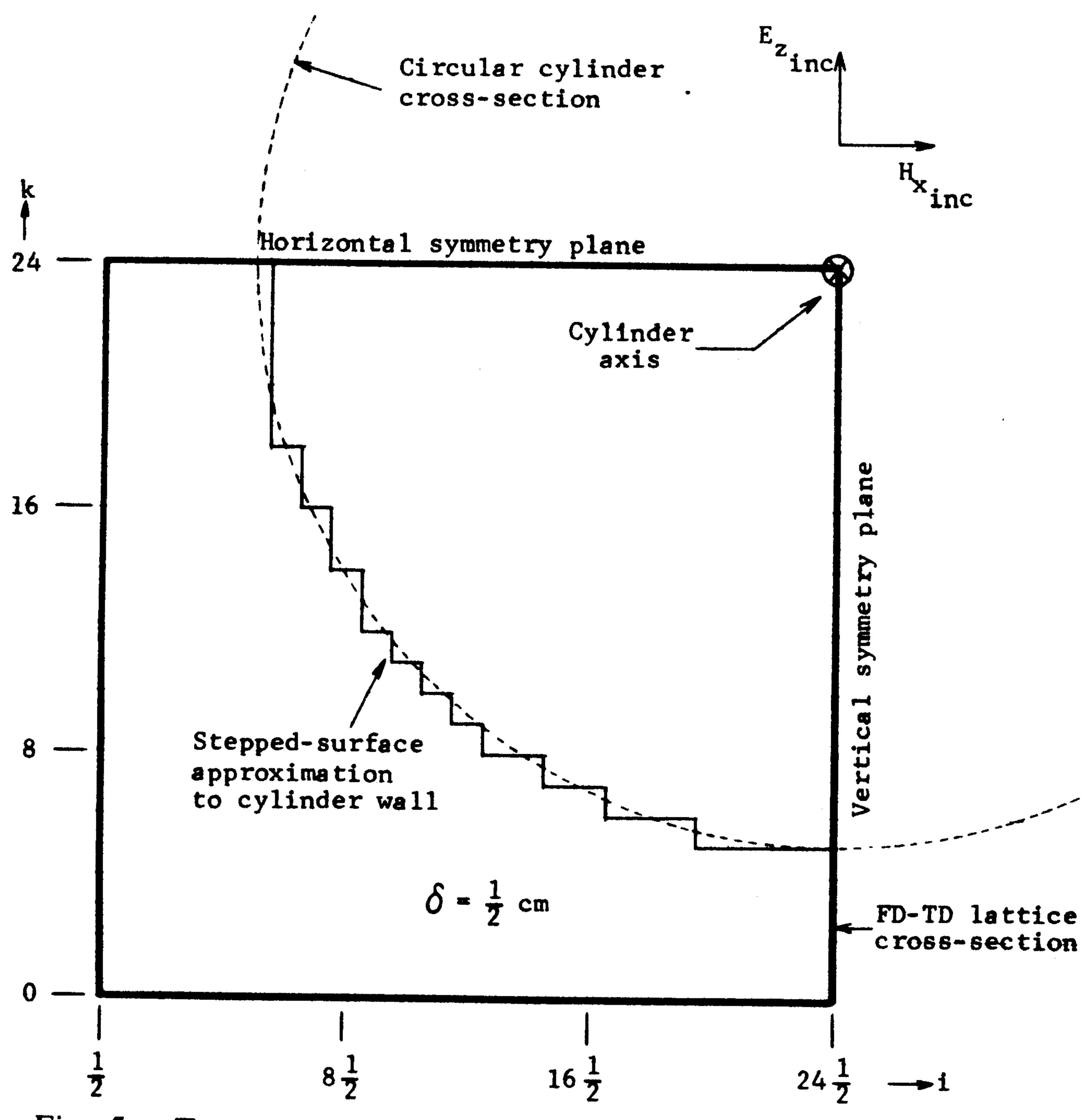
Fig. 5. Transverse cross section of the cylinder model of Fig. 4.
