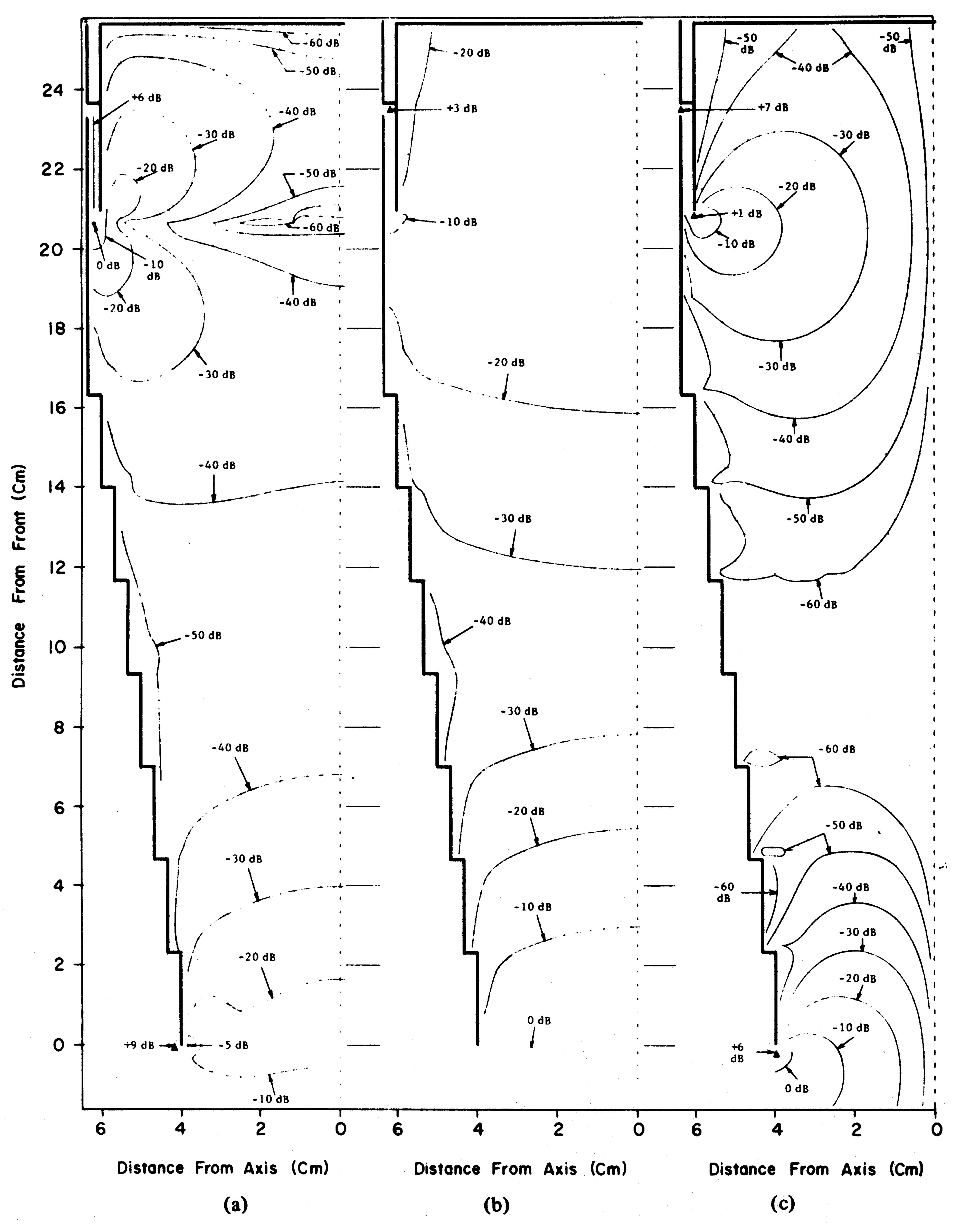
Fig. 12. FD-TD computed field contours in the vertical symmetry plane of the nose cone. (a)  $E_z$ . (b)  $H_x$ . (c)  $E_y$ .
