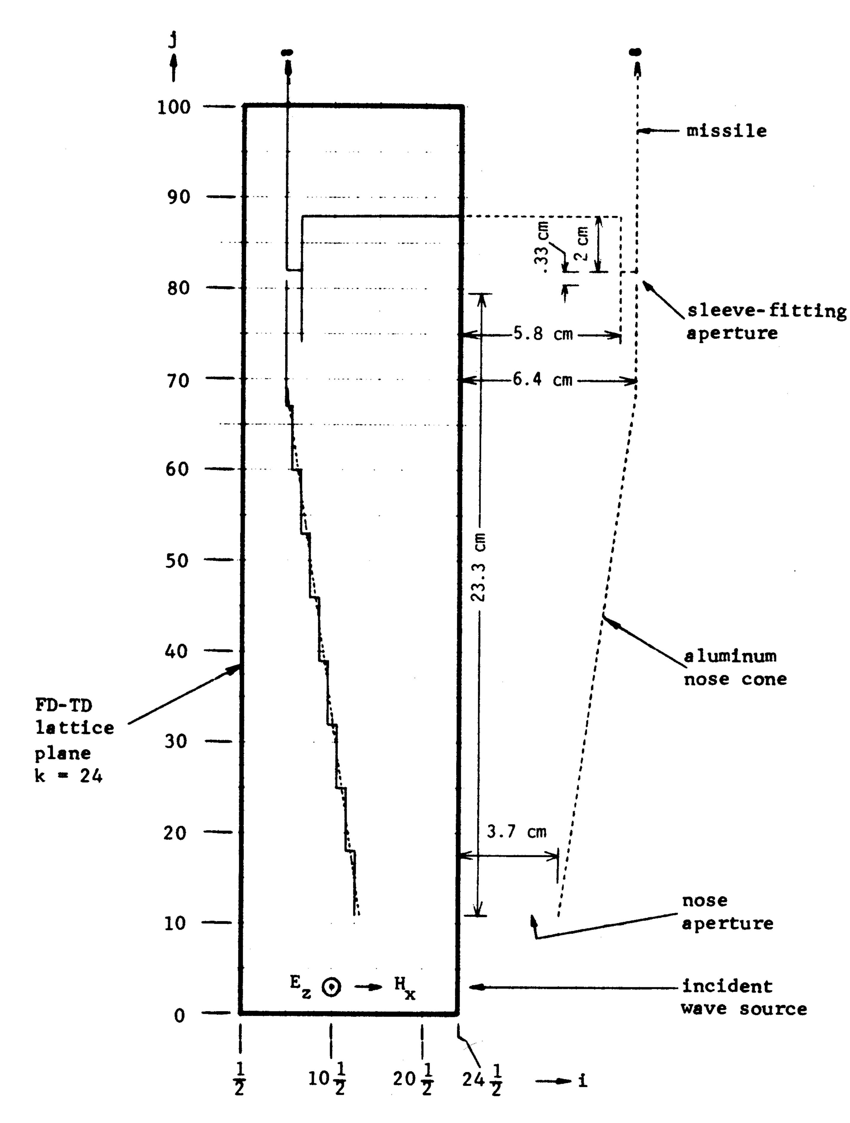
Fig. 10. FD-TD model geometry of an aluminum nose cone with nose aperture and sleeve-fitting aperture, as viewed at lattice plane k = 24 (horizontal symmetry plane).
