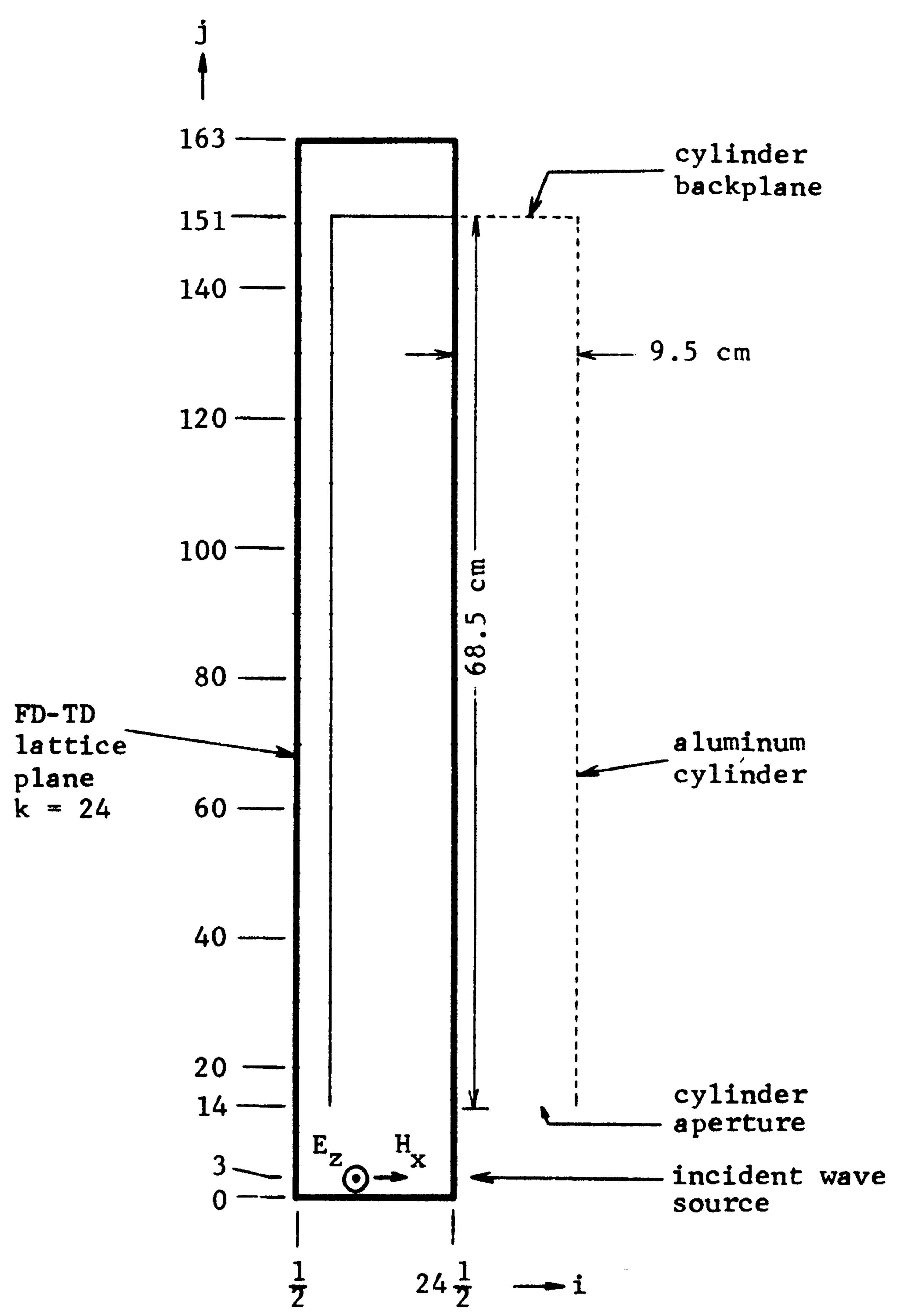
Fig. 4. FD-TD model geometry of a 19.0-cm diameter, 68.5 cm long, open-ended aluminum cylinder, as viewed at lattice plane k = 24 (horizontal symmetry plane).
