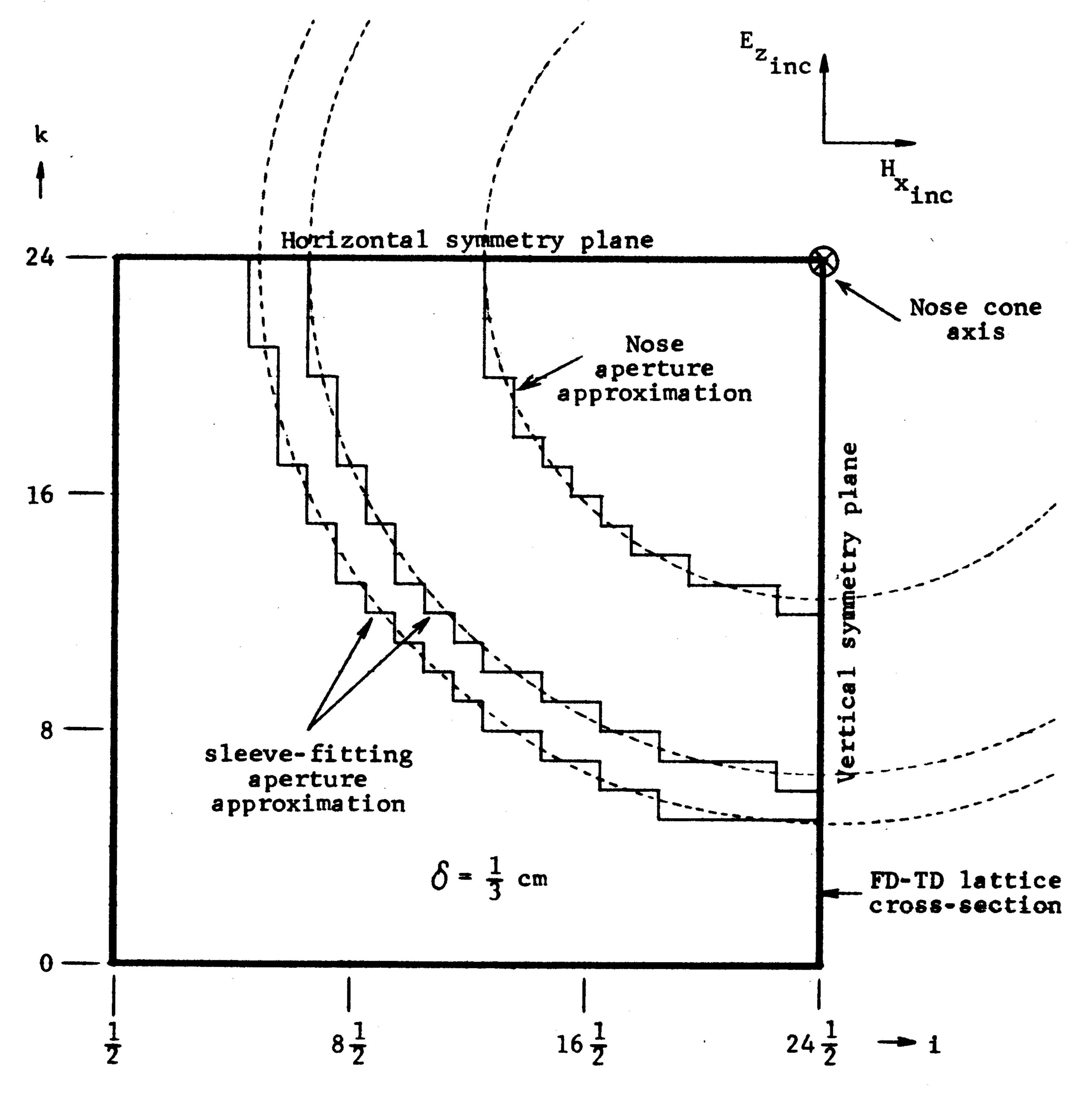
Fig. 11. Transverse cross sections of the nose cone model of Fig. 11.
