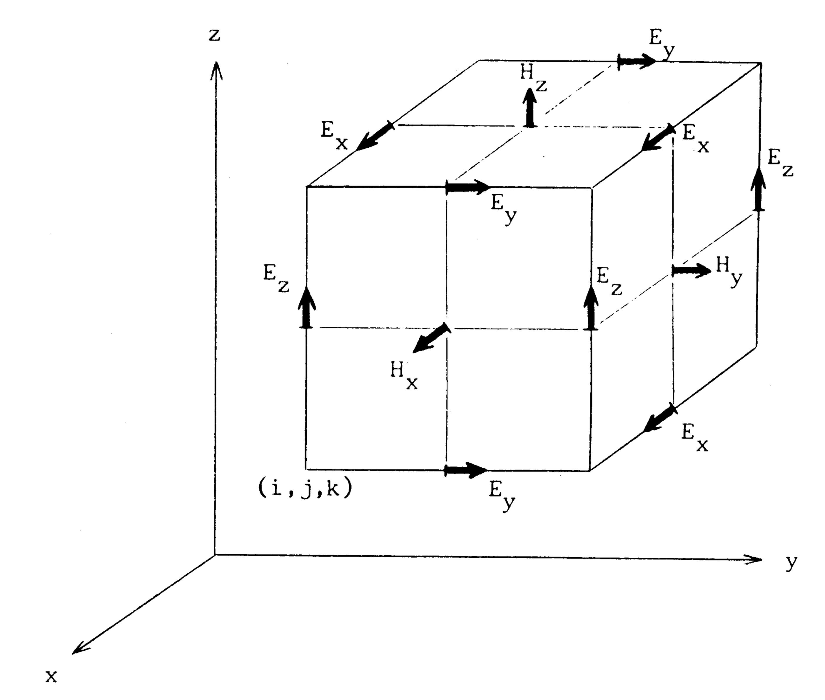
Positions of the field components about a unit cell of the FD\_TD lattice.
