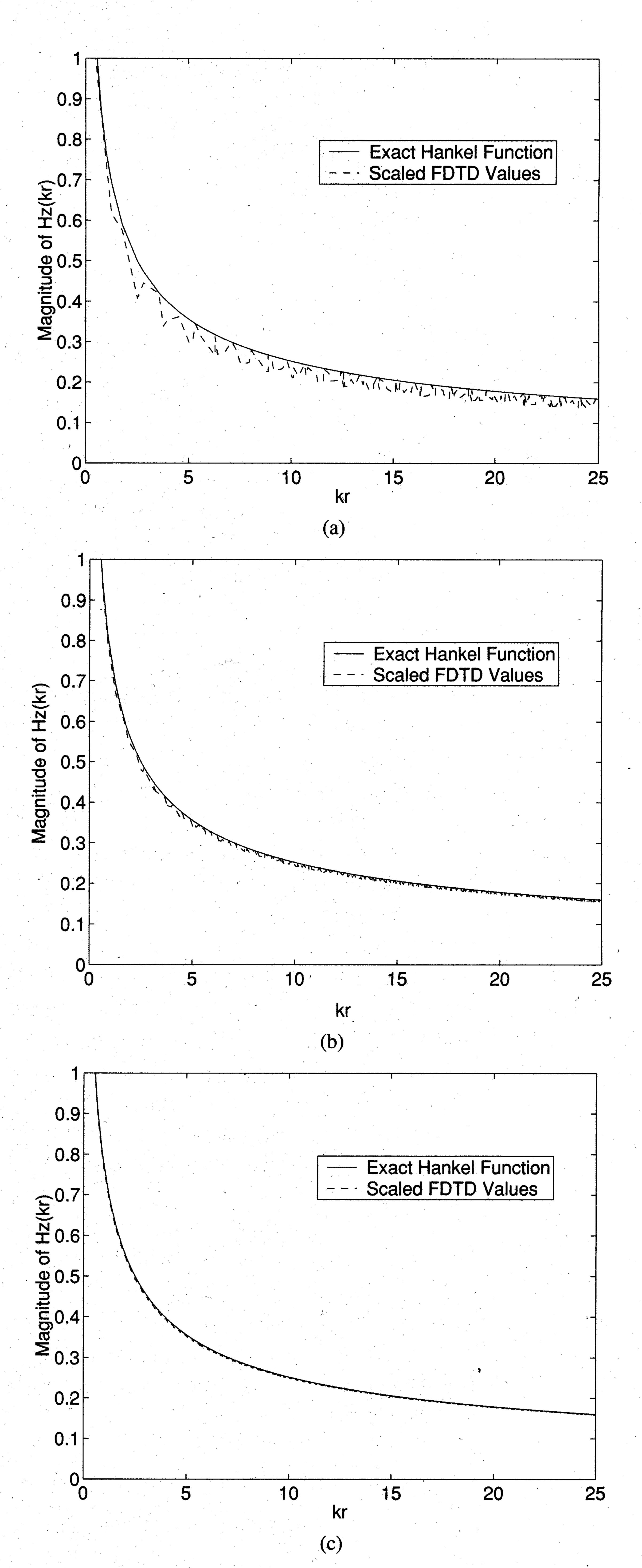
Fig. 2. Scatter diagram of  $|H_z(kr)|$  throughout the entire grid for three grid resolutions: (a)  $\lambda_0/5$ ; (b)  $\lambda_0/10$ ; (c)  $\lambda_0/20$ .
