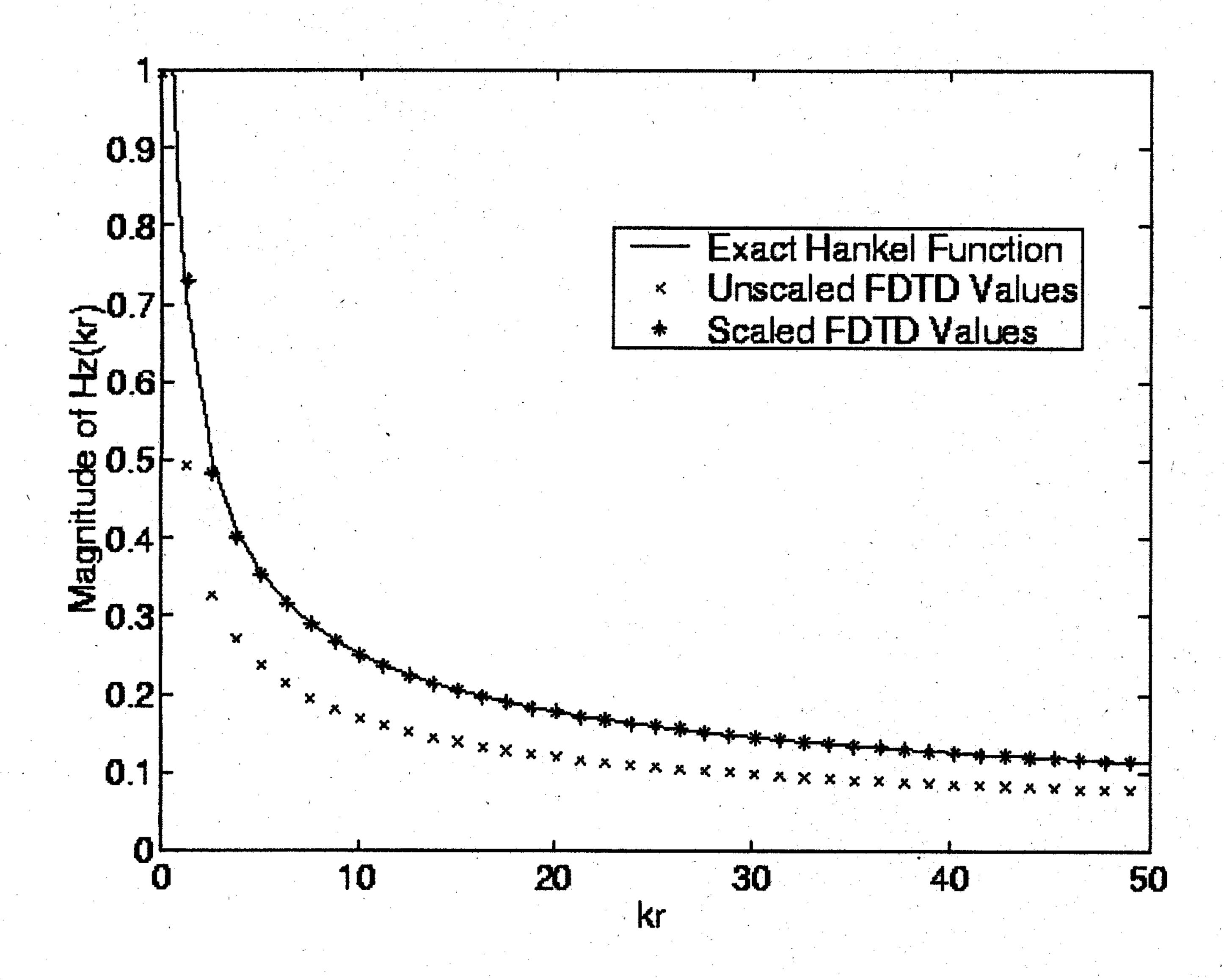
Fig. 1.  $|H_z(kr)|$  with scaled and unscaled FDTD values along the x axis for  $\lambda_0/5$  grid resolution.
