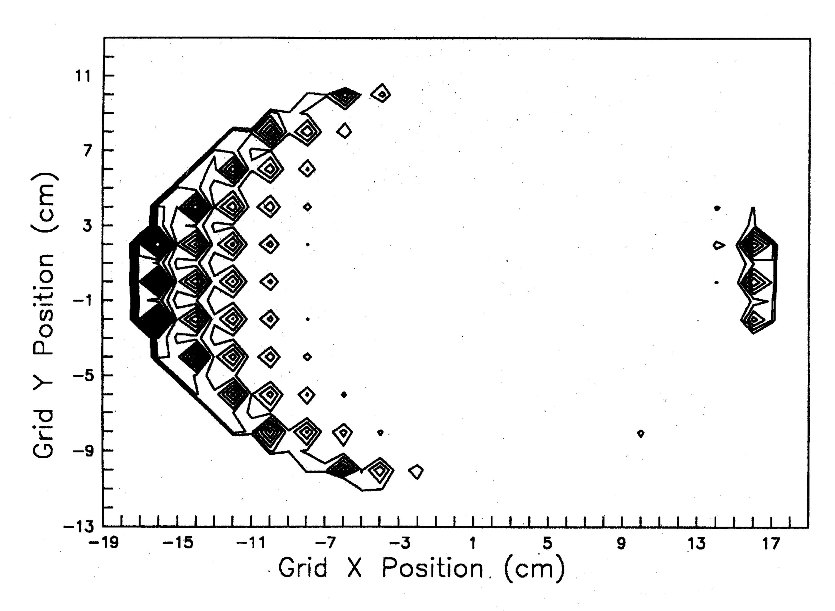
Fig. 7. FDTD predictions for the E-field at the LED sensing matrix under the conditions of Fig. 6. Contours of equal E-field magnitude are shown for LED's having predicted terminal voltages exceeding 1.2-V zero-to-peak. This provides a visualization of both the position and emission intensity of the lit LED's within the phantom, and can be directly compared to Fig. 6.
