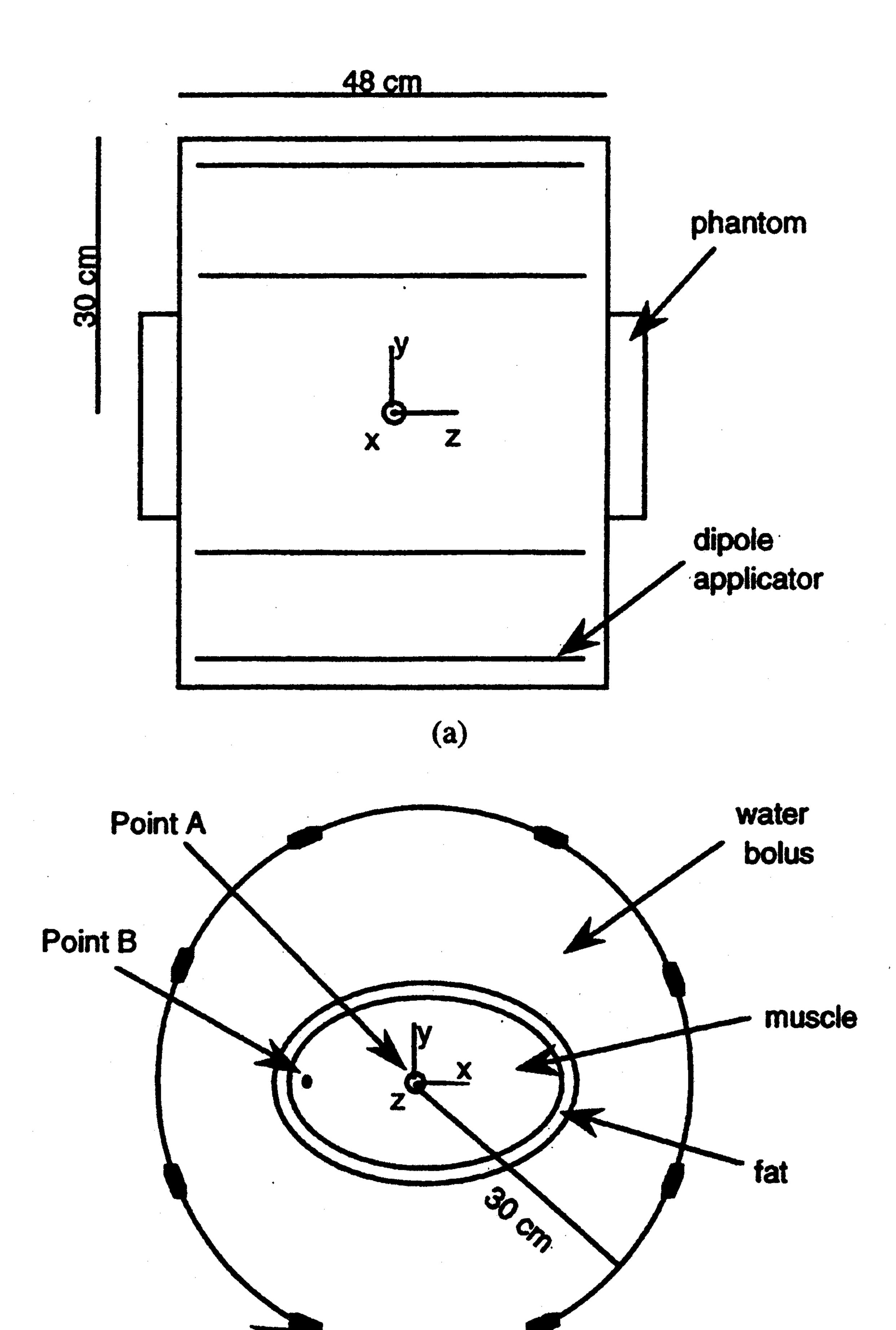
Fig. 1. Schematic representation of the BSD-2000 Sigma-60 applicator and the CDRH phantom. The eight dipole applicators are equally spaced around a 60-cm clear plastic annulus. The phantom has a 1-cm-thick rigid fat-equivalent shell surrounding a muscle-equivalent gel. (a) Longitudinal view. (b) Transverse cross section at z=0.
