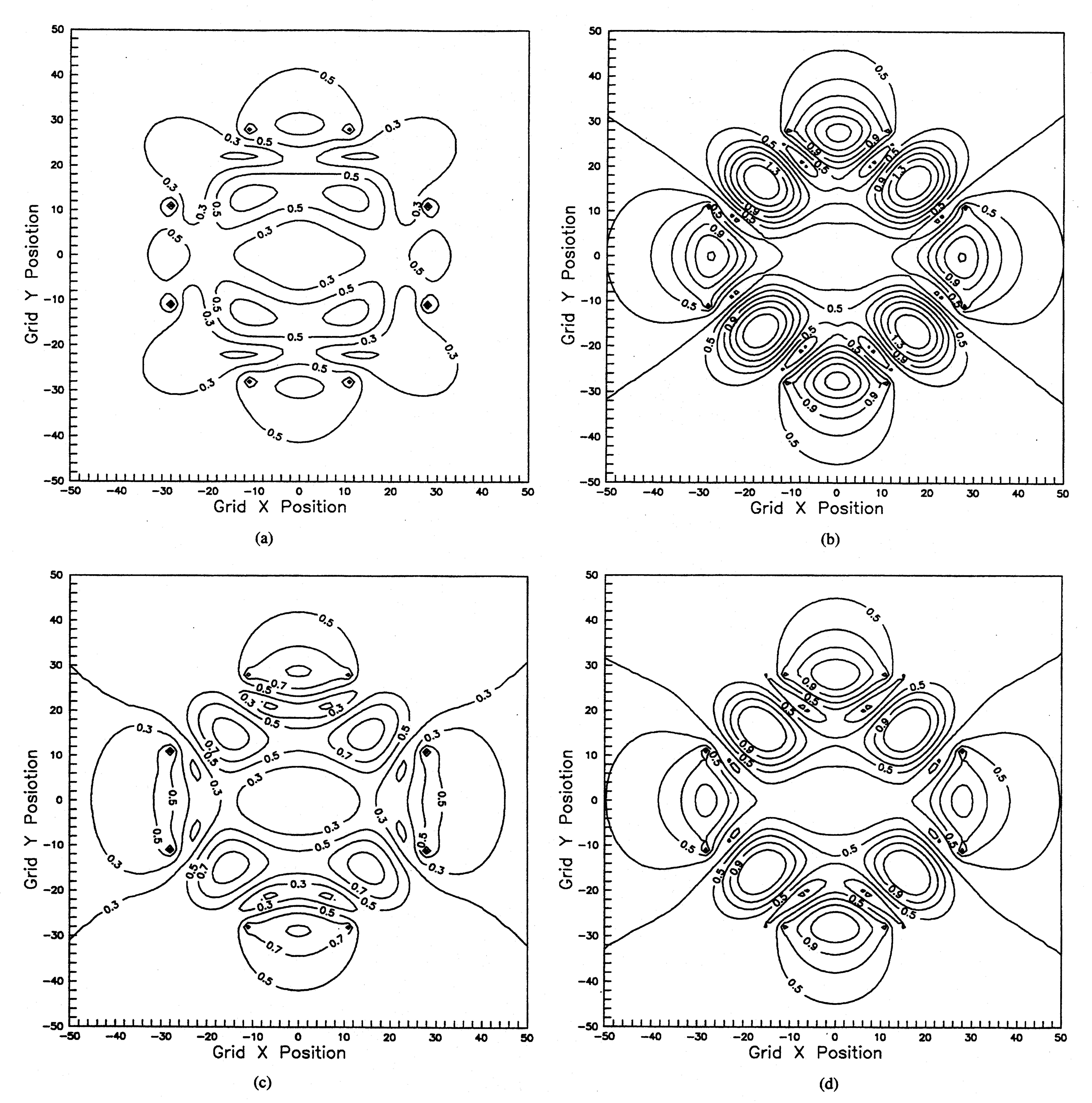
Fig. 5. Distinct modal patterns of the E-field observed within the phantom and water bolus of the 2-D model for 110-MHz equal-magnitude and zero-phase excitation of the annular phased array. (a) After 5 RF cycles, (b) 45 cycles, (c) 85 cycles, and (d) 125 cycles.
