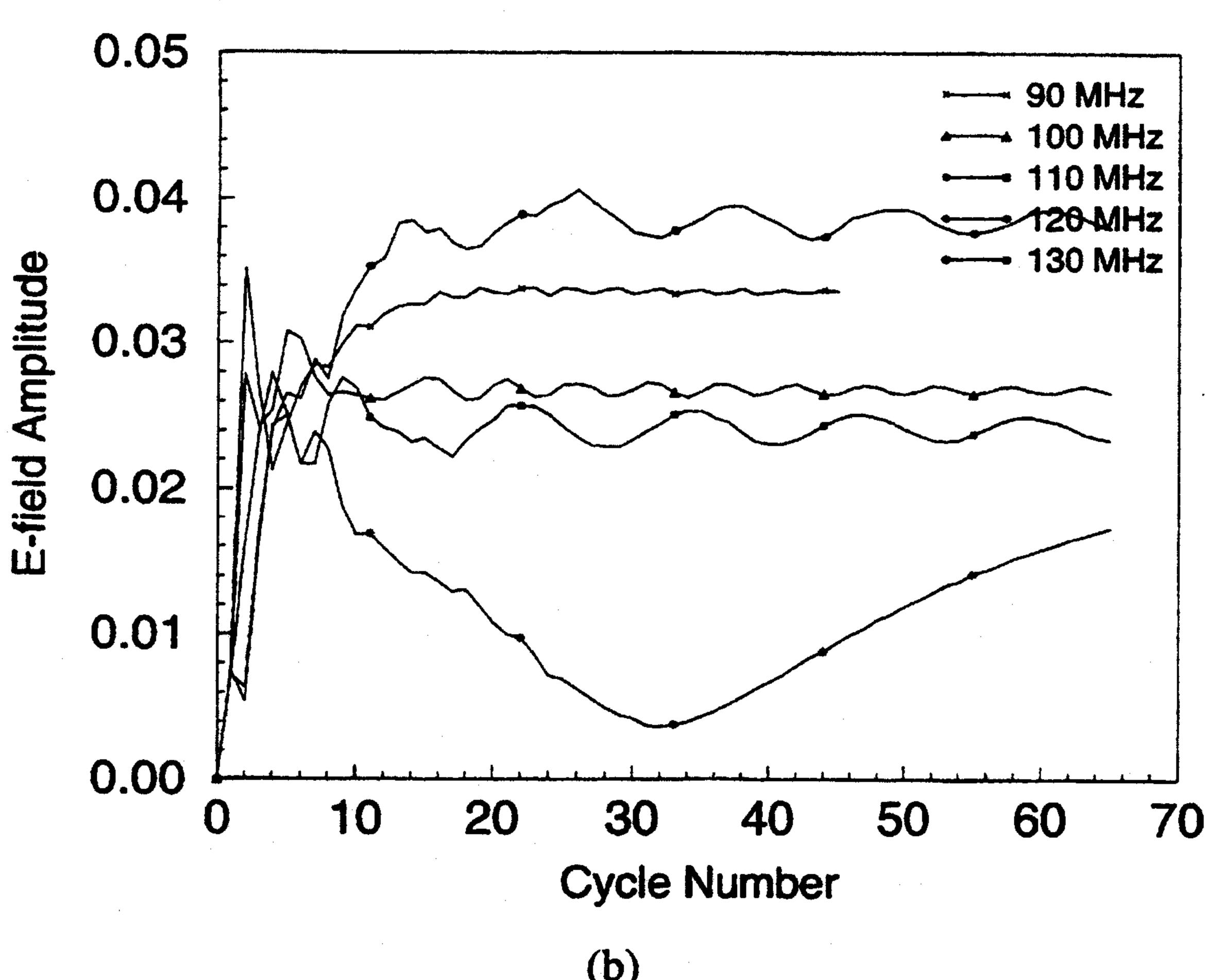
Fig. 4. Electric-field amplitude versus RF cycle number for the 3-D FDTD model for 90-, 100-, 110-, 120-, and 130-MHz equal-magnitude and zero-phase excitation of the annular phased array. (a) Observation Point A(0, 0, 0). (b) Observation Point B(-15 cm, 0, 0), showing pronounced oscillatory behavior at 120 MHz.
