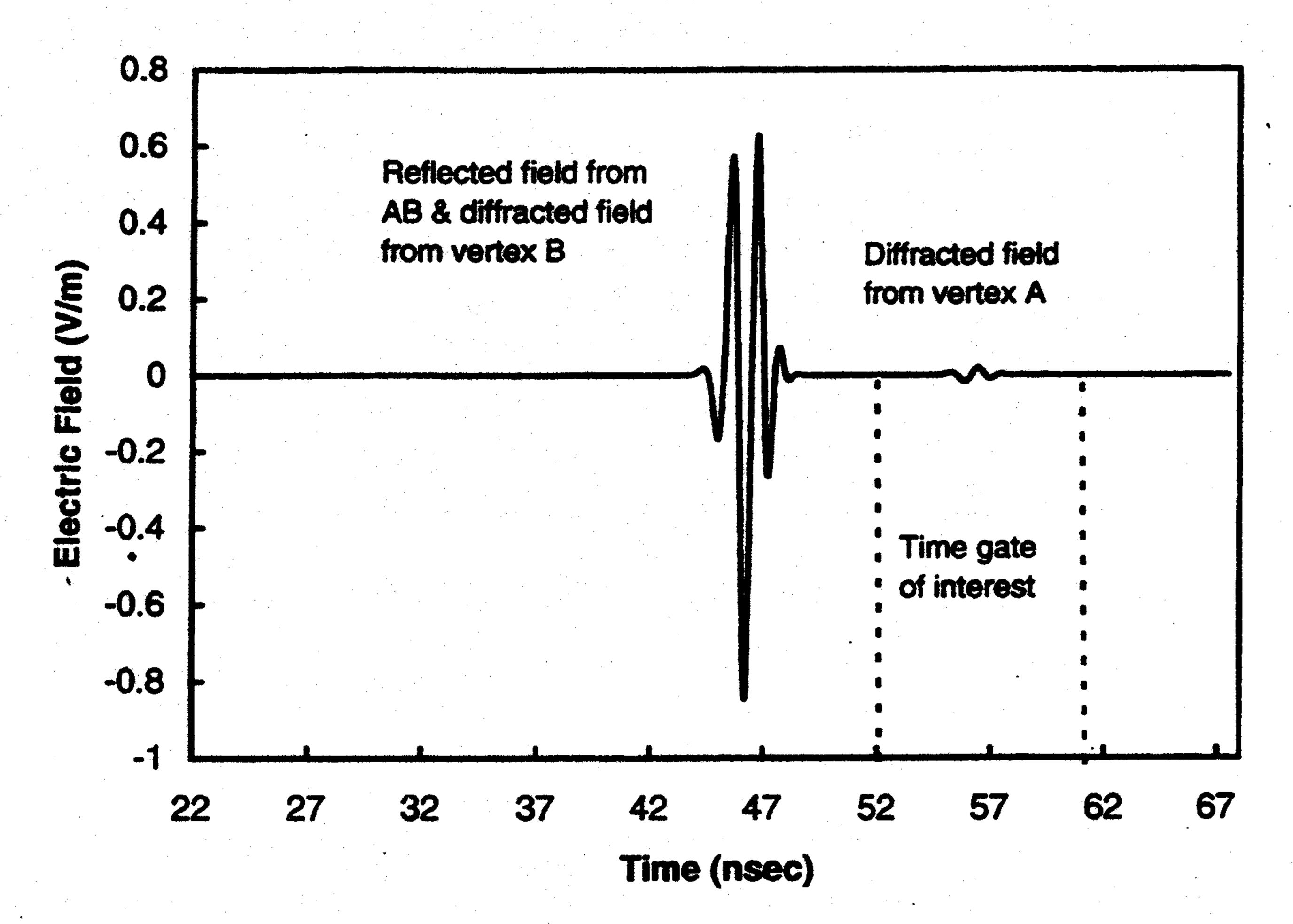
Fig. 3. Time variation of electric field scattered from PEC wedge for the TM polarization case at observation point E ( $\rho = 8.32$  m,  $\phi = 49.56^{\circ}$ ). Diffracted field from vertex A is separated in time from the other fields.
