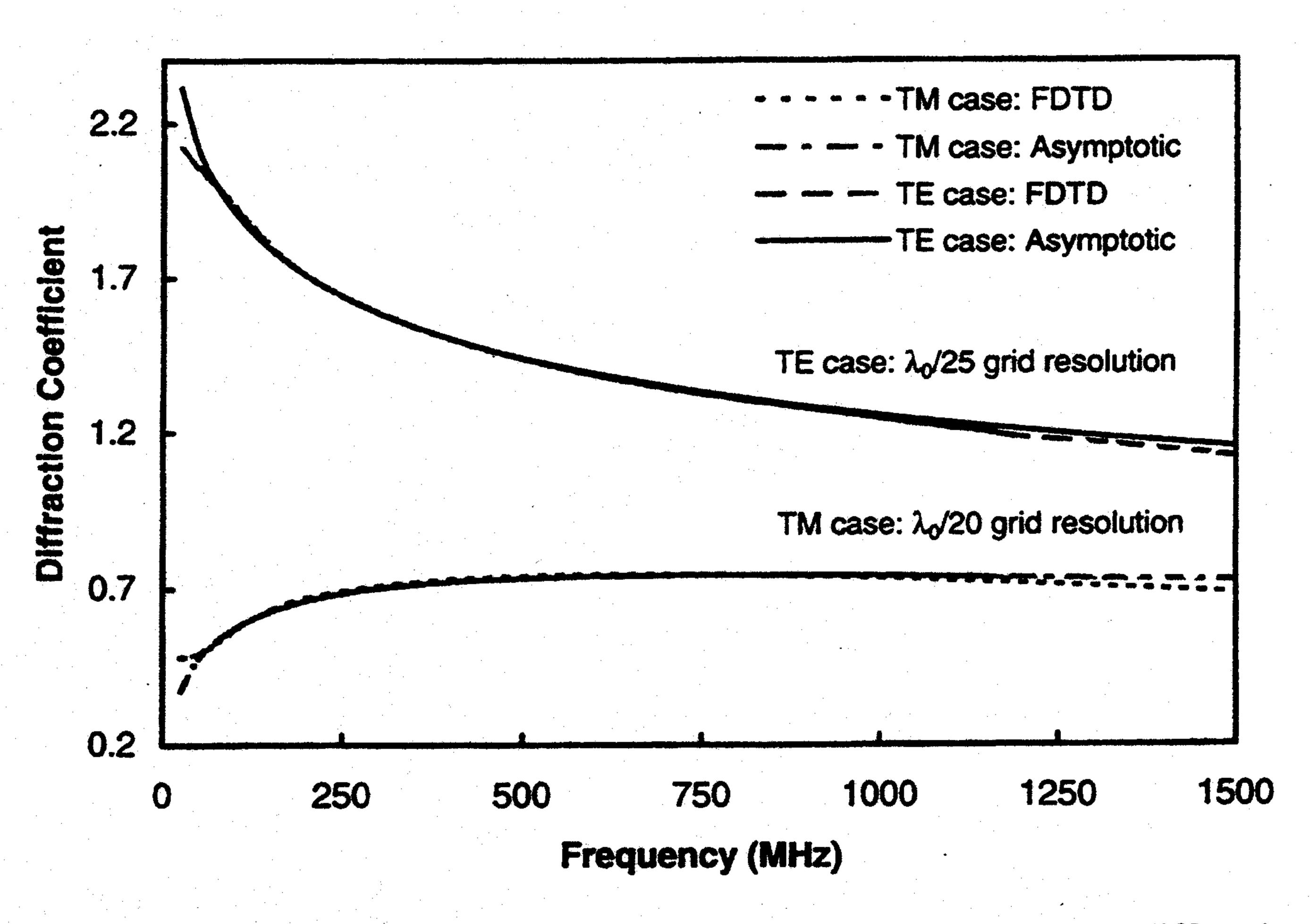
Fig. 5. Comparison of the asymptotic and FDTD results for the diffraction coefficient for PEC wedge at observation point F ( $\rho = 6.30$  m,  $\phi = 262.37^{\circ}$ ) in Region III for TE ( $\lambda_0/25$  grid resolution), and TM ( $\lambda_0/20$  grid resolution) polarizations.
