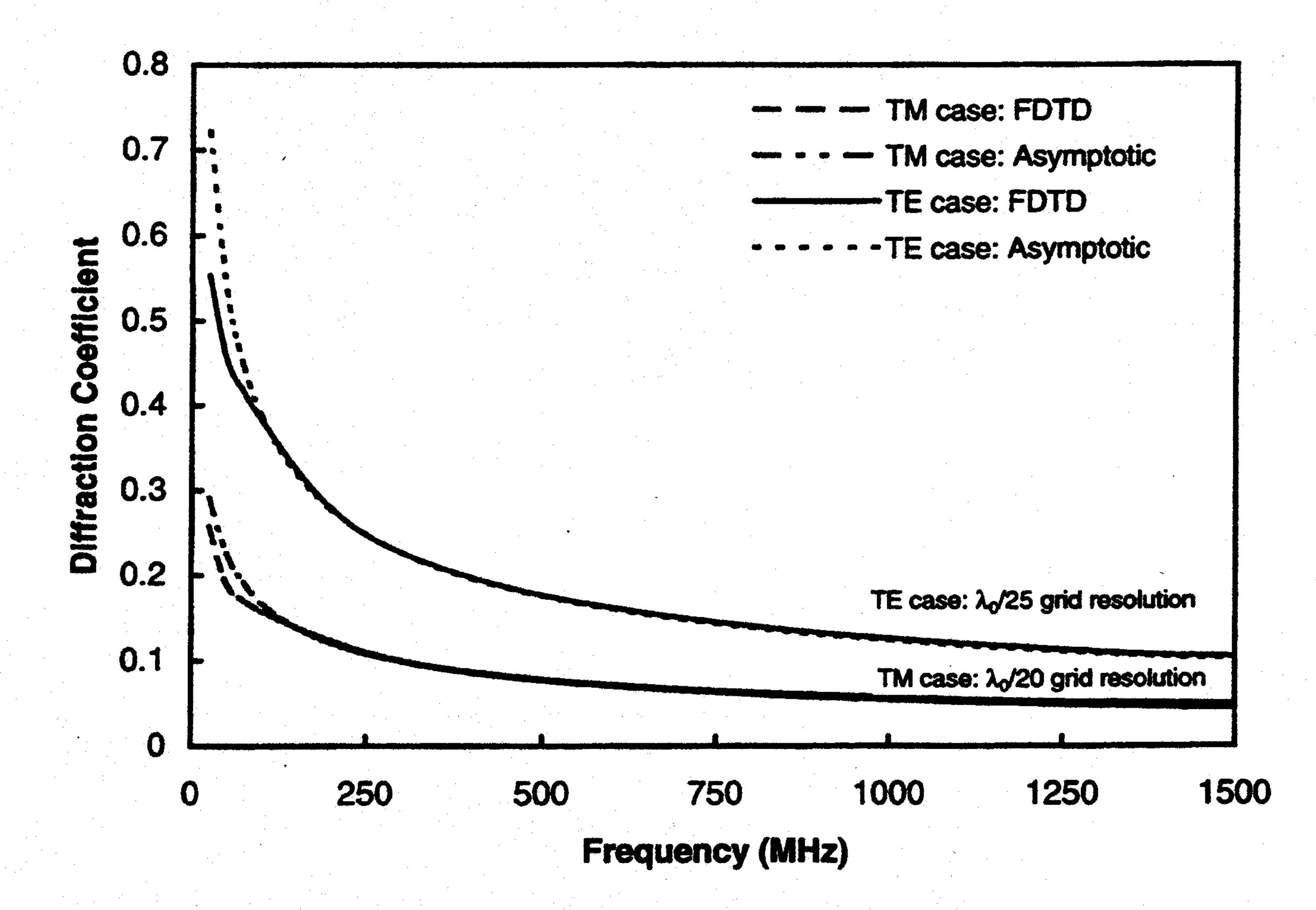
Fig. 4. Comparison of the asymptotic and FDTD results for the diffraction coefficient for PEC wedge at observation point E ( $\rho = 8.32$  m,  $\phi = 49.56^{\circ}$ ) in Region I for TE ( $\lambda_0/25$  grid resolution), and TM ( $\lambda_0/20$  grid resolution) polarizations.
