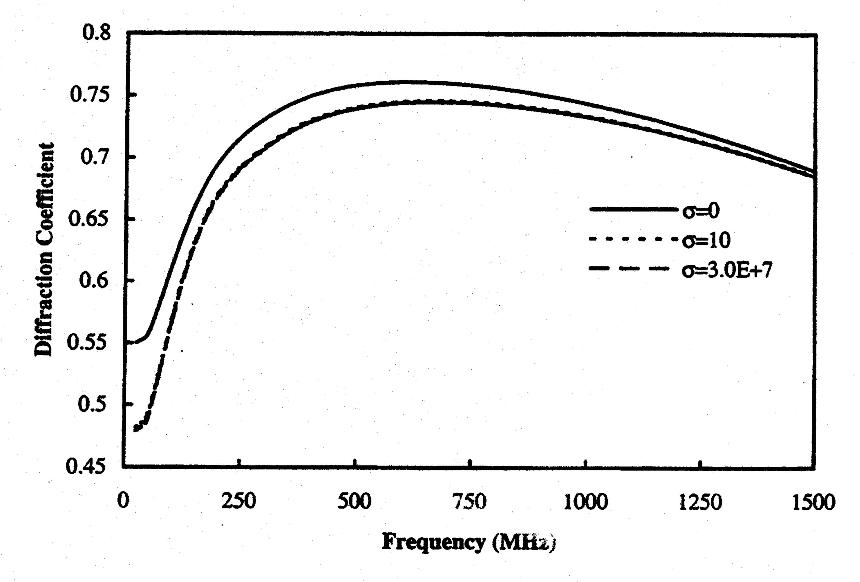
Fig. 8. FDTD computed diffraction coefficient for infinite dielectric wedge at observation point F ( $\rho = 6.30$  m,  $\phi = 262.37^{\circ}$ ) for the TM polarization case. Results are shown for fixed dielectric constant ( $\varepsilon = 7$ ) and varying conductivity for a fixed-grid resolution  $\lambda_0/20$ .
