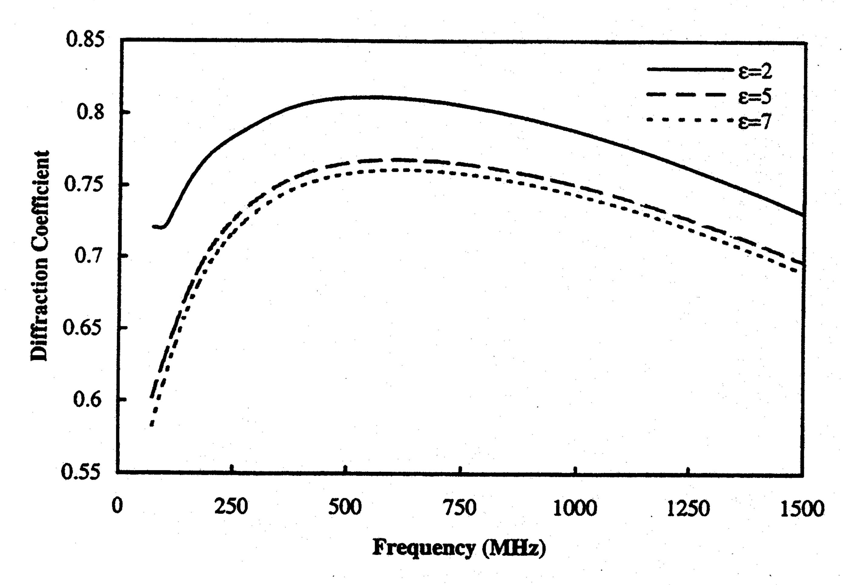
Fig. 6. FDTD computed diffraction coefficient for infinite lossless dielectric wedge at observation point F ( $\rho=6.30$  m,  $\phi=262.37^{\circ}$ ) for the TM polarization case. Results are shown for  $\varepsilon=2$ ,  $\varepsilon=5$ ,  $\varepsilon=7$  for a fixed-grid resolution  $\lambda_0/20$ .
