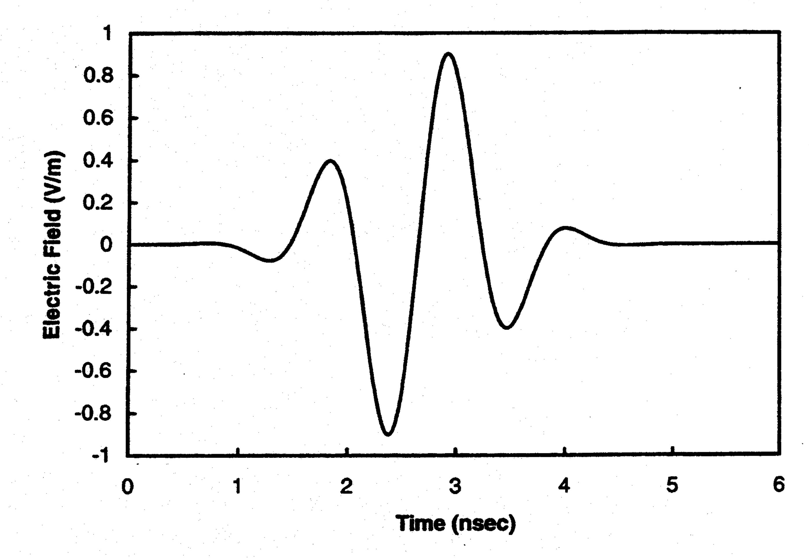
Fig. 2. Electric field source for the TM polarization case. Pulsed plane wave with a Gaussian envelope of 1.3-ns duration full width at half maximum (FWHM).
