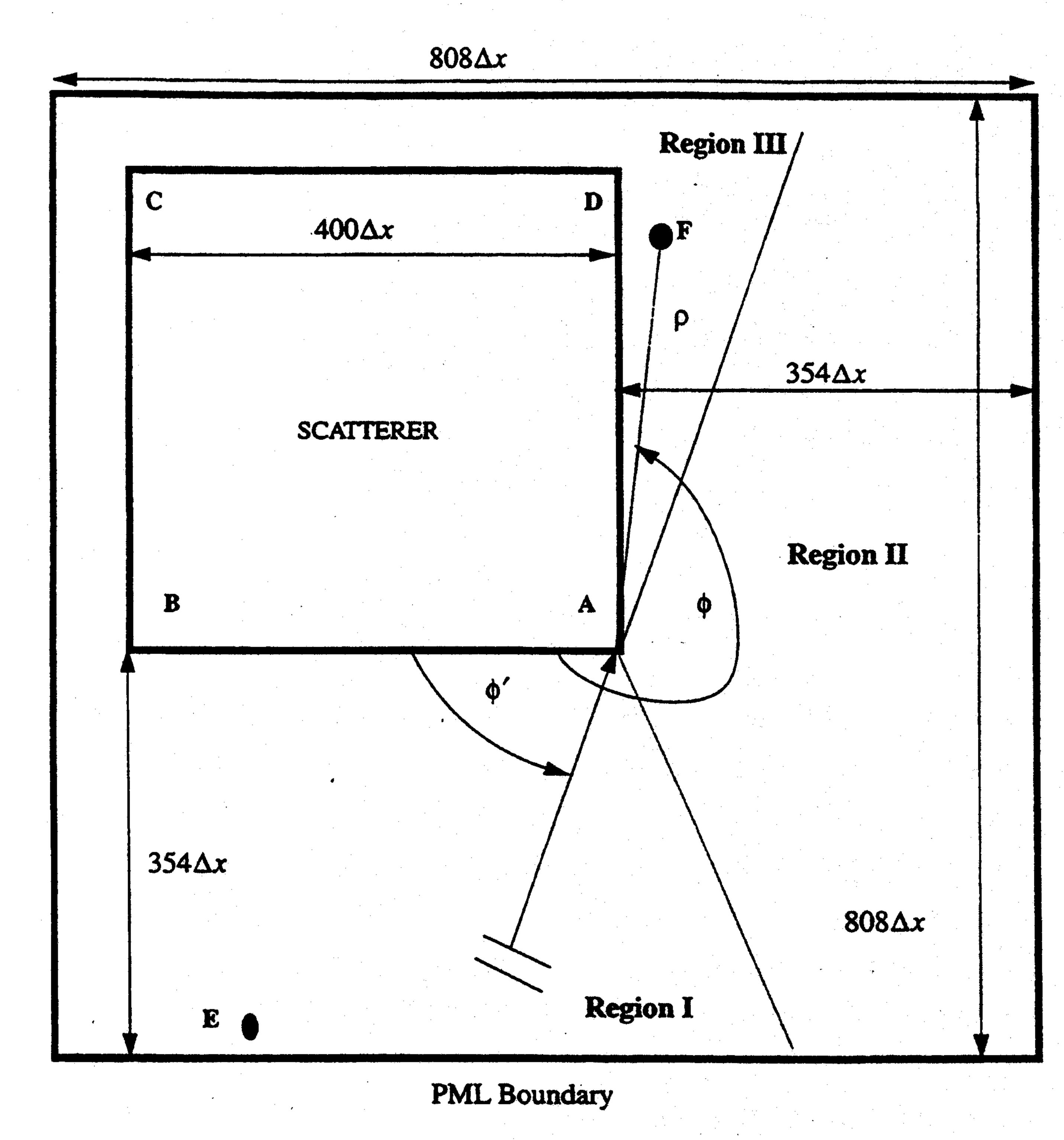
Fig. 1. Two-dimensional geometry of the grid and scatterer.
