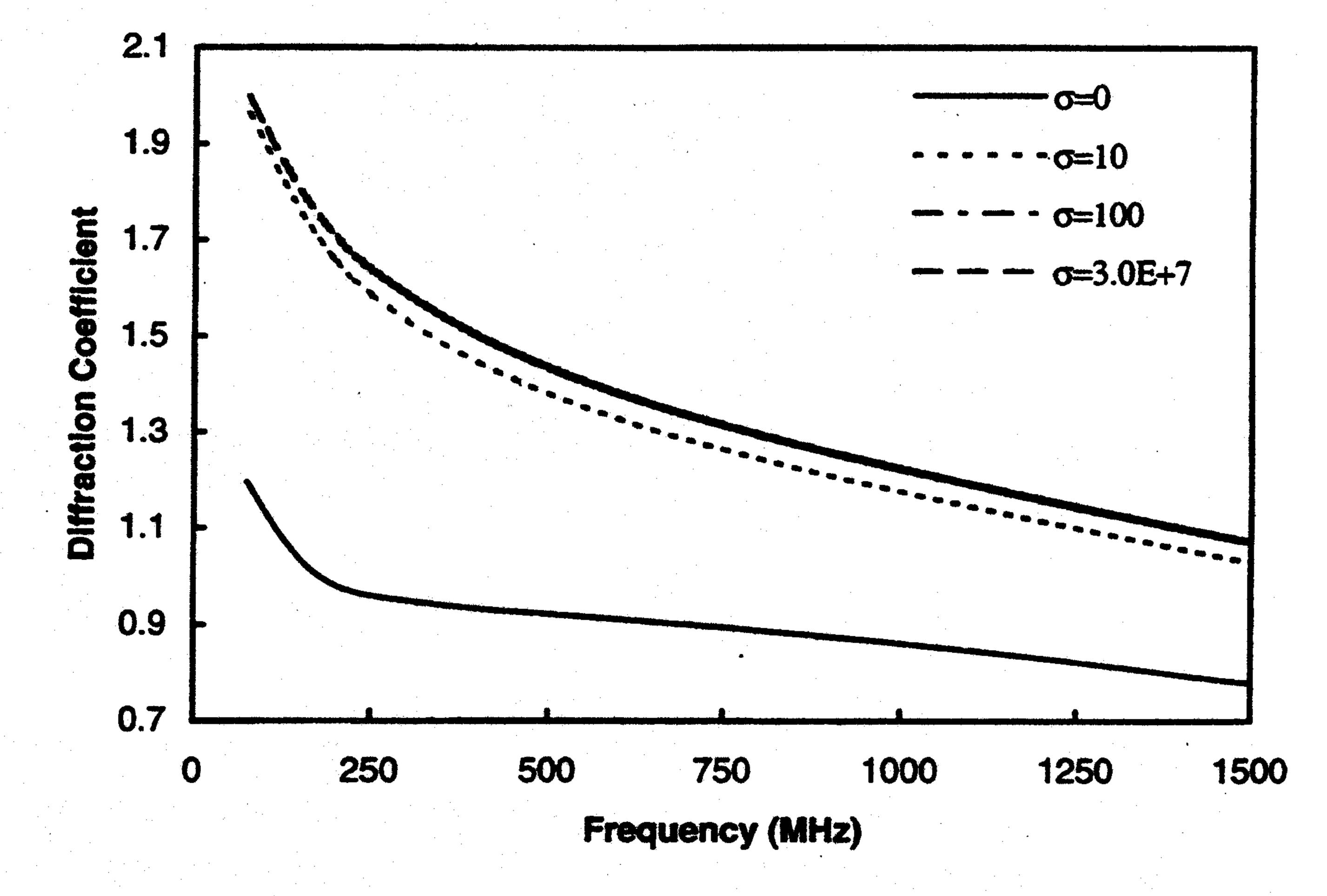
Fig. 9. FDTD computed diffraction coefficient for infinite dielectric wedge at observation point F ( $\rho = 6.30$  m,  $\phi = 262.37^{\circ}$ ) for the TE polarization case. Results are shown for fixed dielectric constant ( $\varepsilon = 7$ ) and varying conductivity for a fixed-grid resolution  $\lambda_0/20$ .
