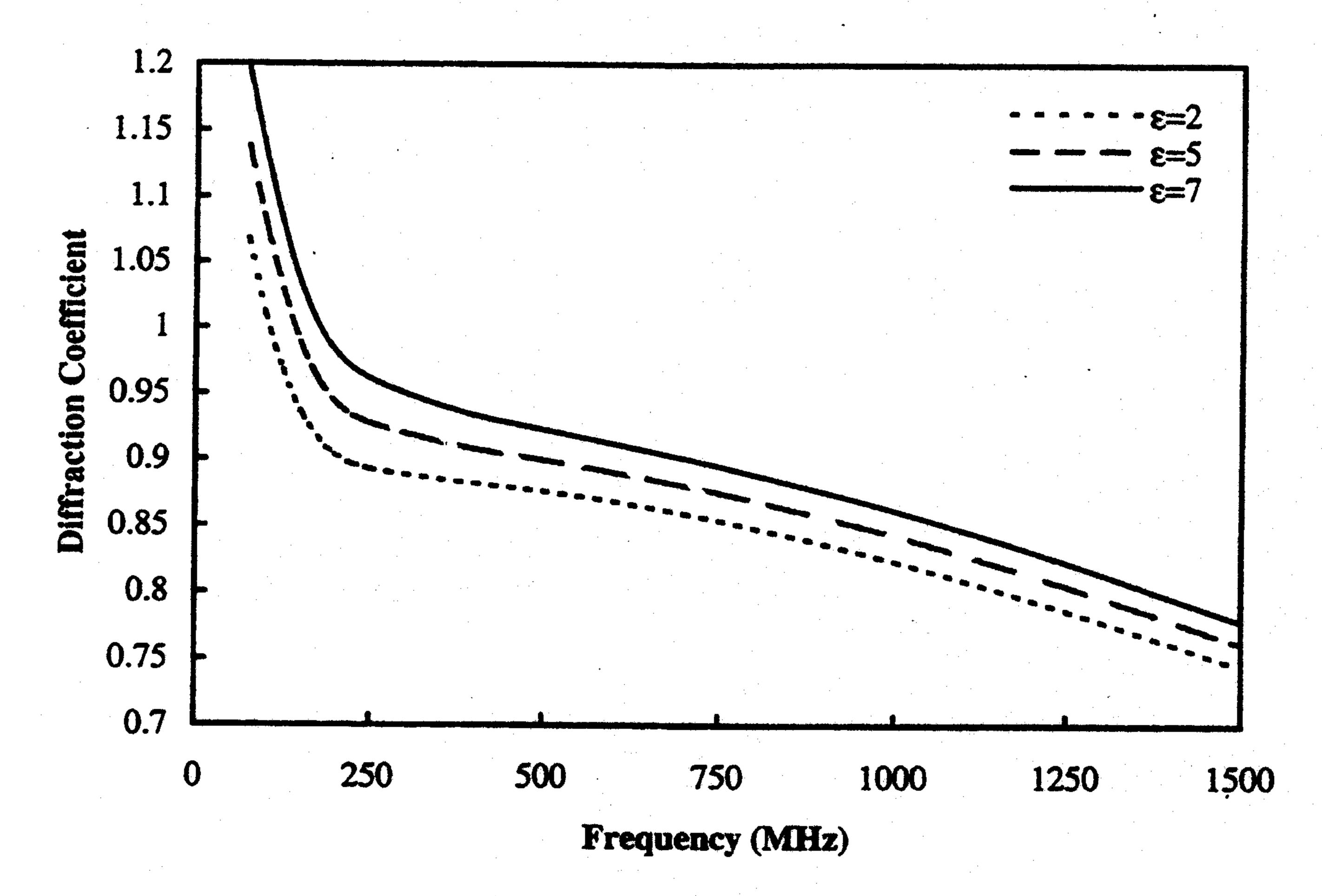
Fig. 7. FDTD computed diffraction coefficient for infinite lossless dielectric wedge at observation point F ( $\rho = 6.30$  m,  $\phi = 262.37^{\circ}$ ) for the TE polarization case. Results are shown for  $\varepsilon = 2$ ,  $\varepsilon = 5$ ,  $\varepsilon = 7$  for a fixed-grid resolution  $\lambda_0/20$ .
