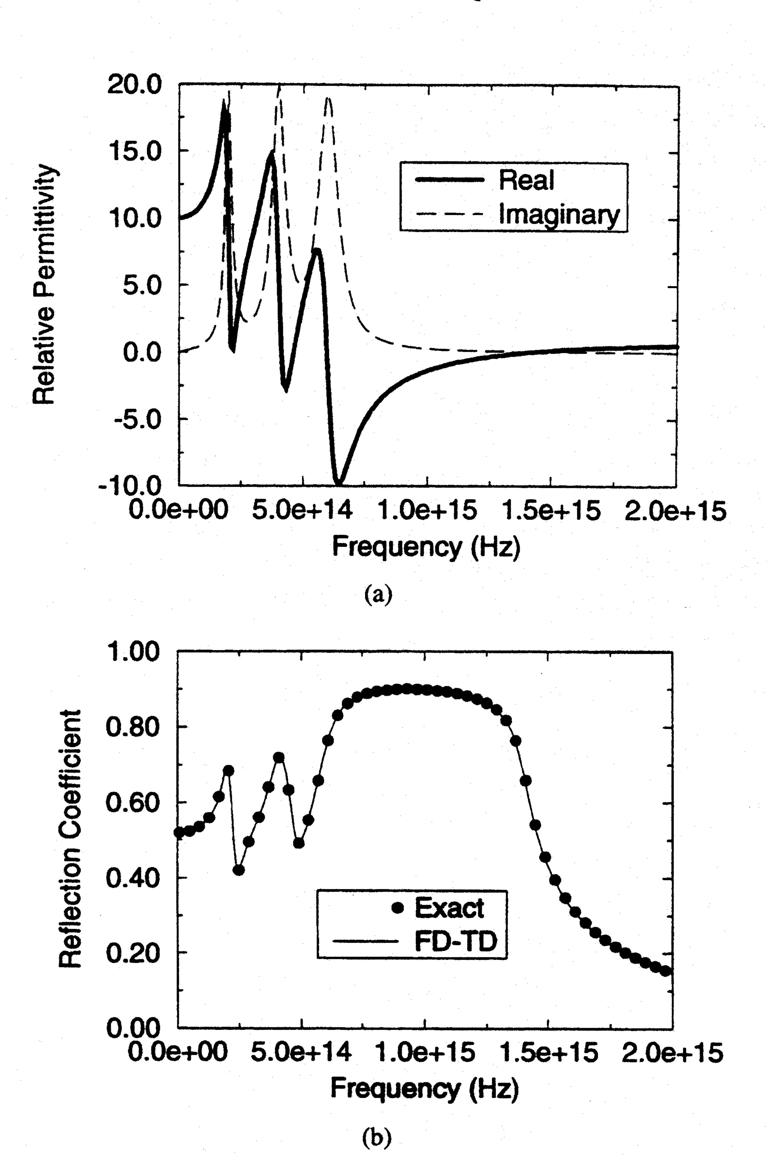
Fig. 1. (a) Real and imaginary parts of the permittivity of a Lorentz medium having three resonances in the optical range. (b) Comparison of FDTD and exact results from dc to  $2.0 \times 10^{15}$  Hz for the magnitude of the reflection coefficient of a half-space composed of the medium of (a).  $\Delta x = 2.65$  nm,  $\Delta t = 8.85$  as. Problem size: 20000 1-D cells, 20000 time steps. Computer resources: 0.92 MW; 1000 CPU s on a single processor of the Cray J90 [2].
