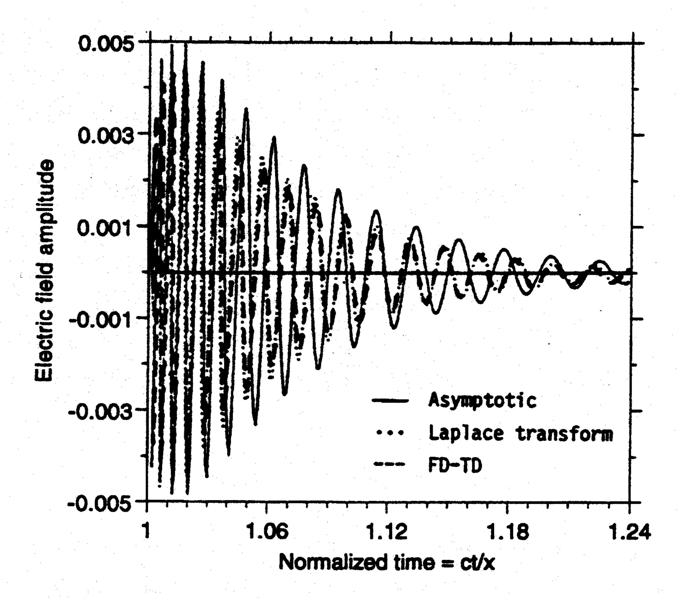
Fig. 2. Comparison of FDTD, asymptotic, and Laplace transform results for the Sommerfeld precursor observed at  $x=1\,\mu\mathrm{m}$  in a Lorentz-dispersive medium for a unit-step modulated sinusoidal excitation of  $\omega_c=1.0\times10^{16}$  at x=0.  $\Delta x=0.0157$  nm,  $\Delta t=0.0523$  as. Problem size: 80 000 1-D cells, 80 000 time steps. Computer resources: 1.4 MW; 965 CPU s on a single processor of the Cray J90 [2].
