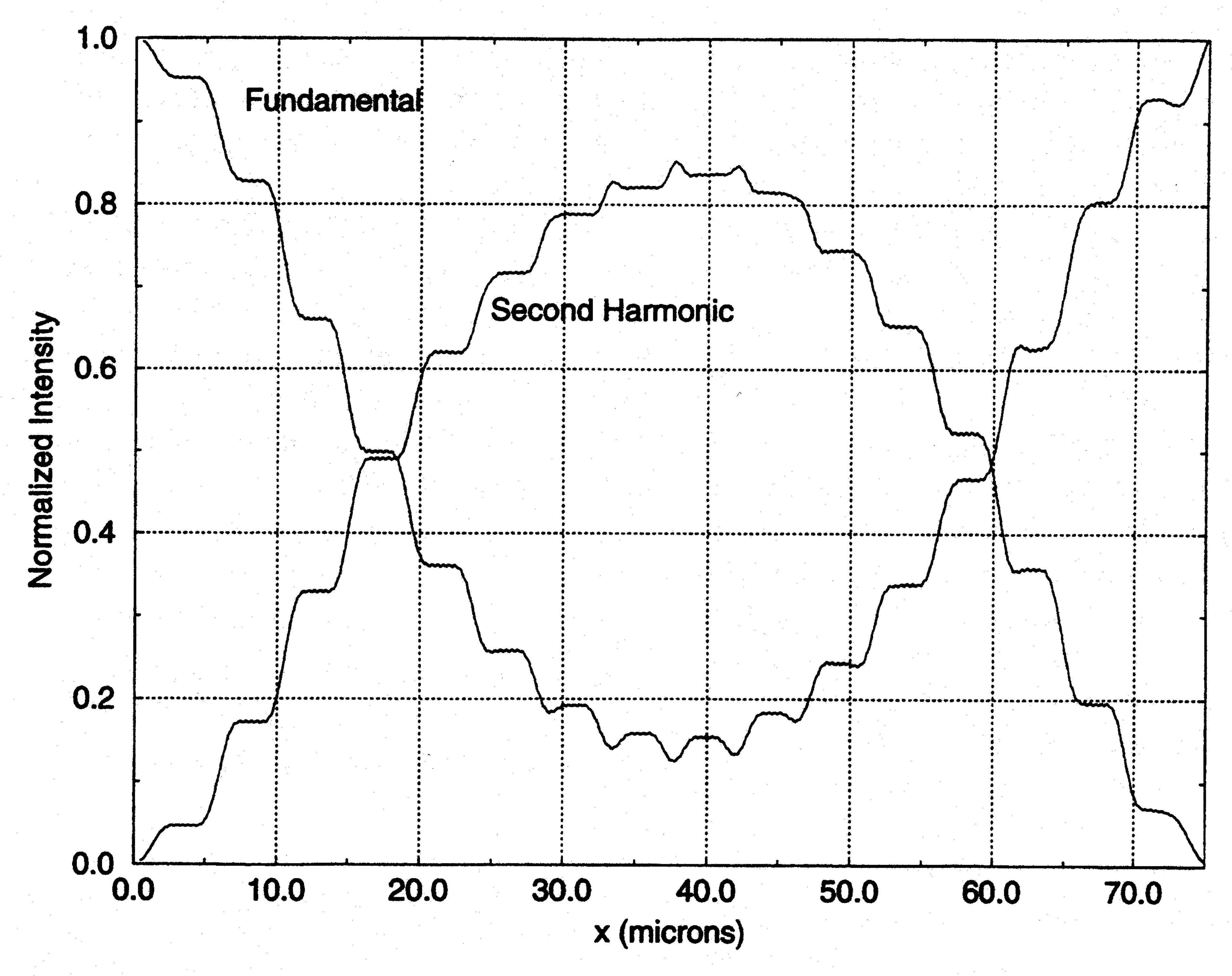
Fig. 6. FDTD-computed normalized intensities for both the fundamental ( $\lambda = 1.5 \,\mu\text{m}$ ) and the second-harmonic ( $\lambda = 0.75 \,\mu\text{m}$ ) fields along the length of a 2-D slab waveguide with a QPM grating of period 4.54  $\,\mu\text{m}$ .  $\Delta x = 20.83$  nm,  $\Delta t = 34.7$  as. 10000 time steps. Computer resources: 6.7 MW; 1300 CPU s on a single processor of the Cray J90.
