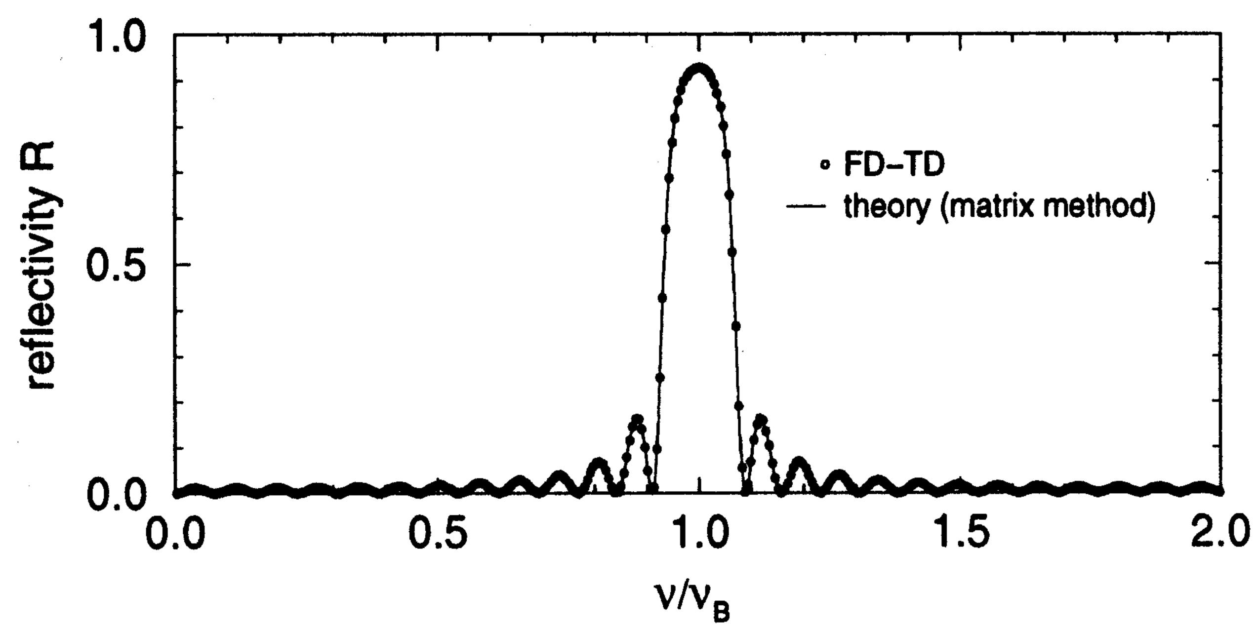
Figure 6. FD-TD computed reflectivity spectrum for the bottom mirror of the microcavity FP-SEL.
