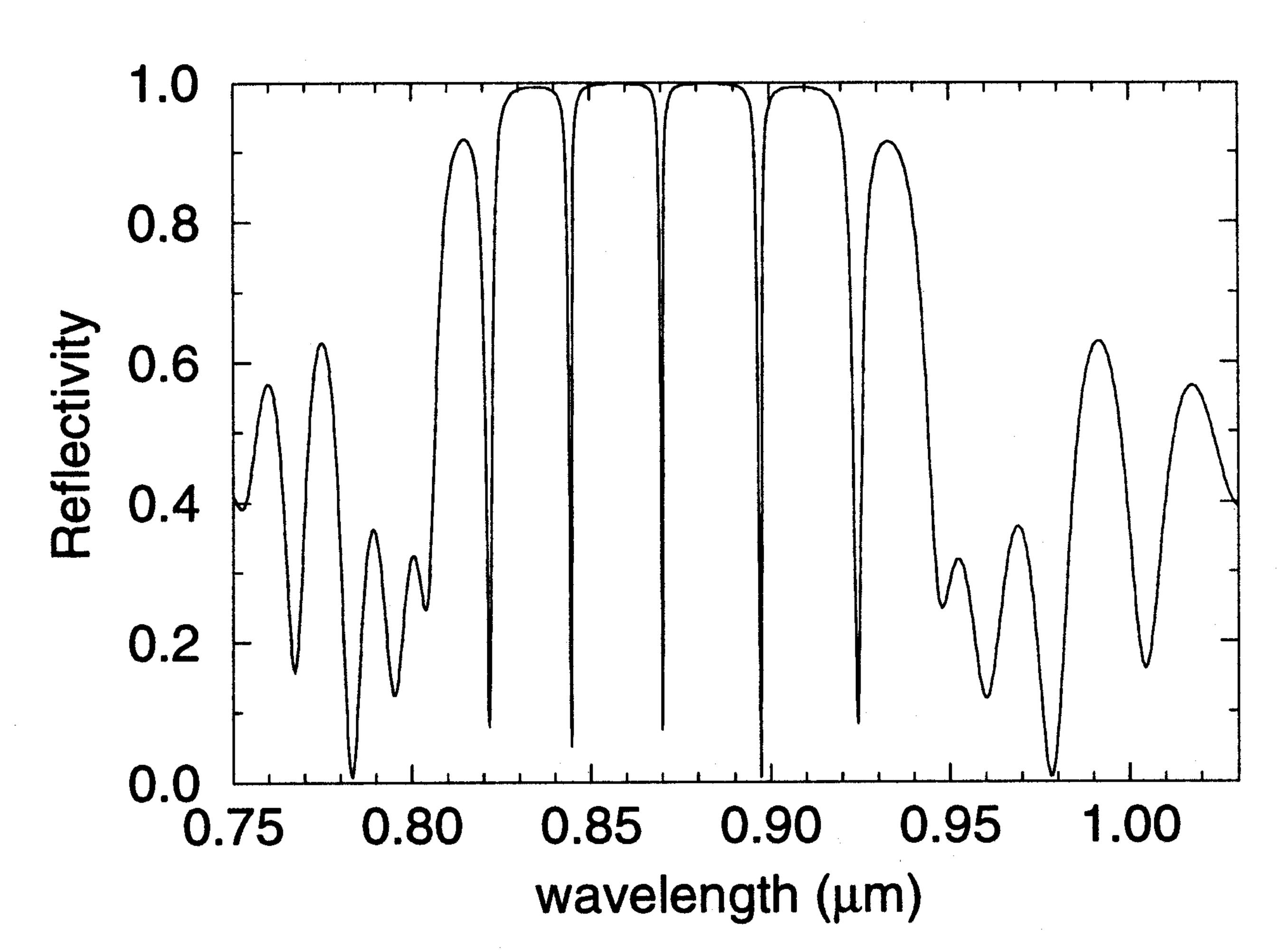
Figure 7. FD-TD computed reflectivity spectrum for the entire microcavity FP-SEL. The gain regions are inactive for this cold-cavity analysis.
