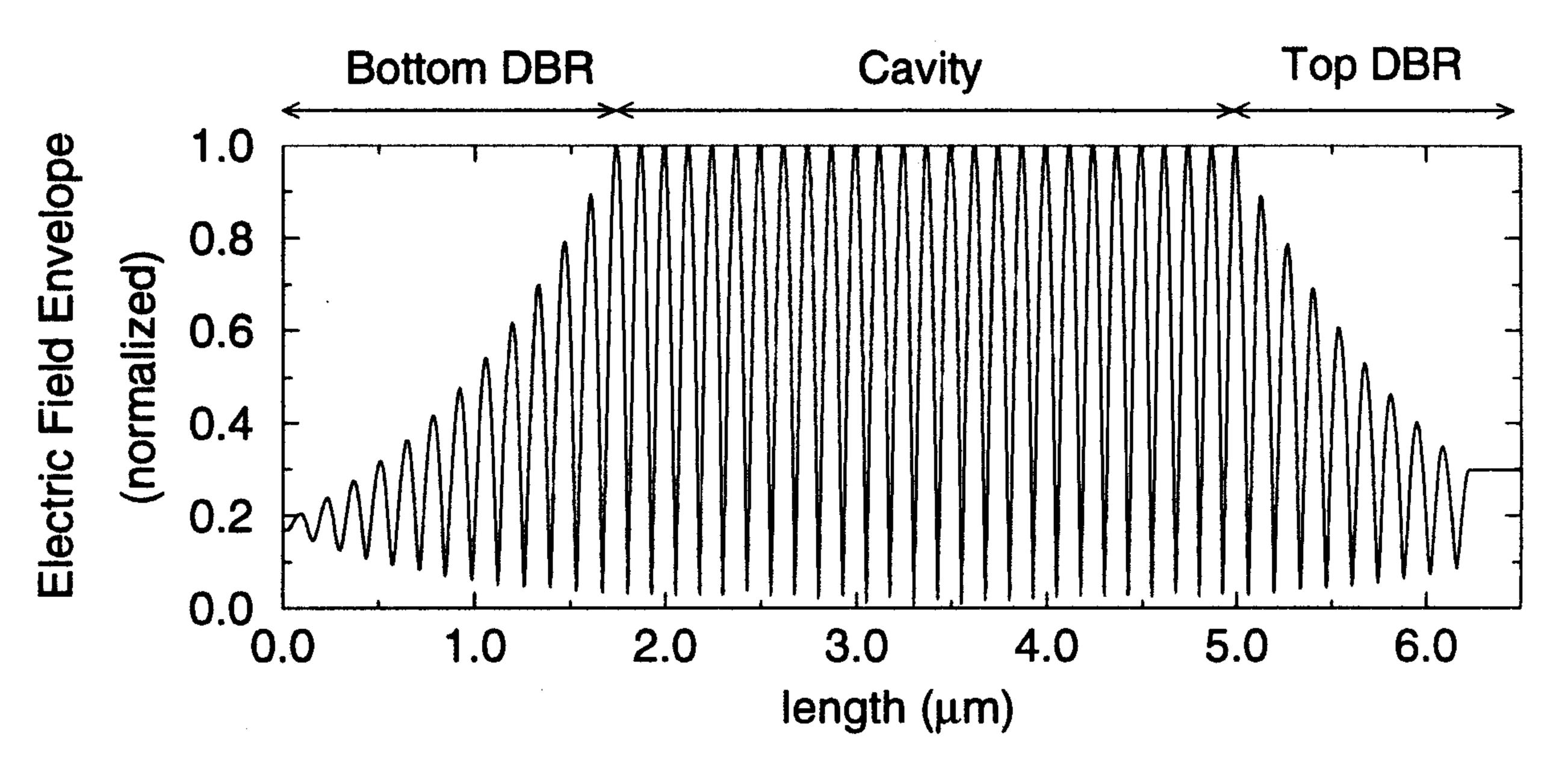
Figure 8. FD-TD results for the spatially varying steady state electric field pattern throughout the microcavity FP-SEL with a UGS.
