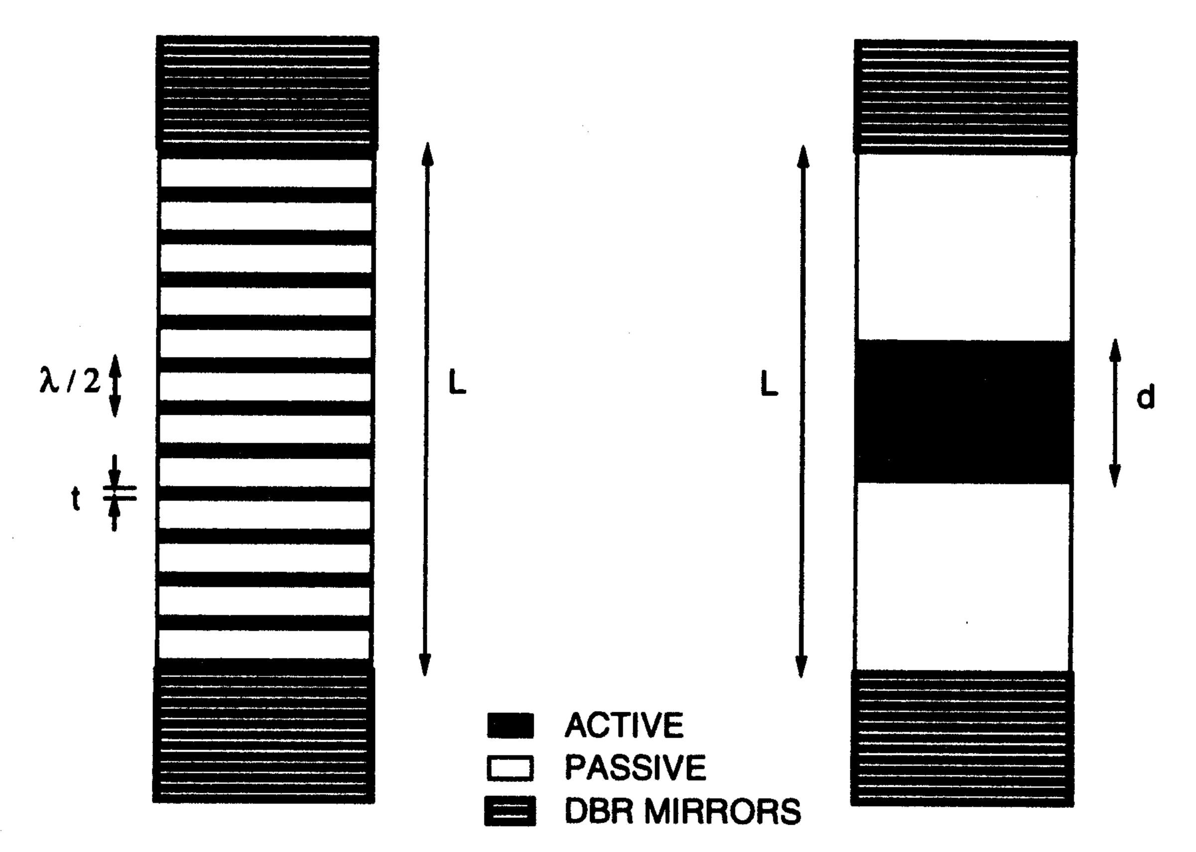
Figure 5. Schematic of microcavity Fabry-Perot surface-emitting lasers (FP-SELs) with vertical distributed Bragg reflectors (DBRs) and uniform (UGS) and periodic gain structures (PGS) within the cavity.
