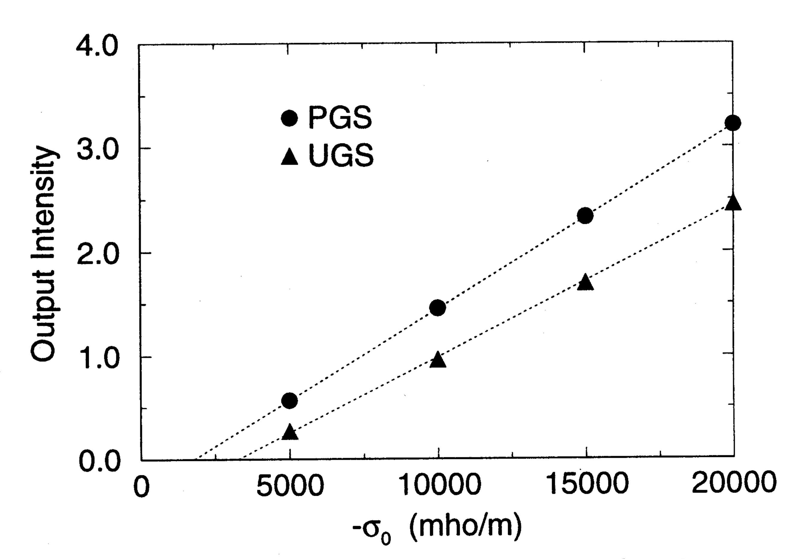
Figure 9. FD-TD computed L-I curve for the output intensity of the the microcavity FP-SEL. Comparison between the UGS and PGS reveals the following advantages of the PGS: a substantial reduction in gain threshold and a higher output intensity.
