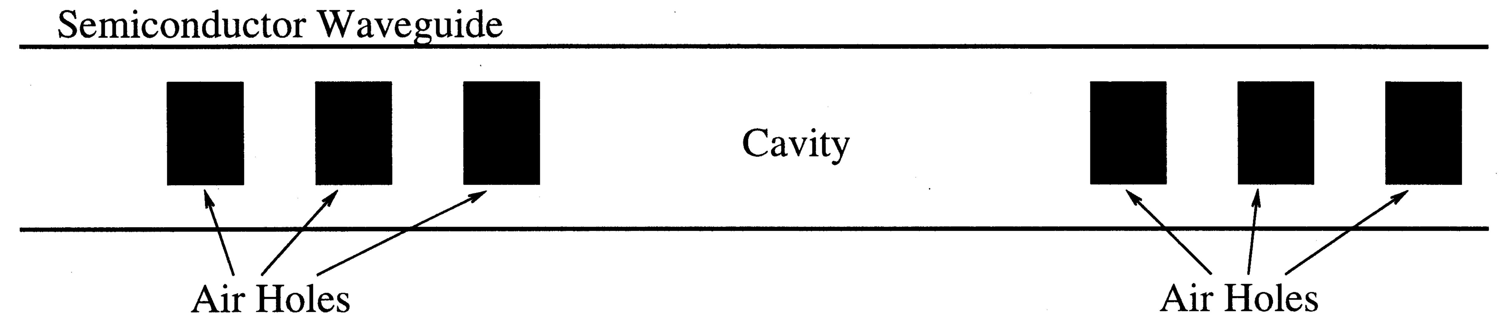
Figure 10. Schematic of a photonic-wire laser cavity defined by two photonic bandgap structures which act as broadband DBRs.
