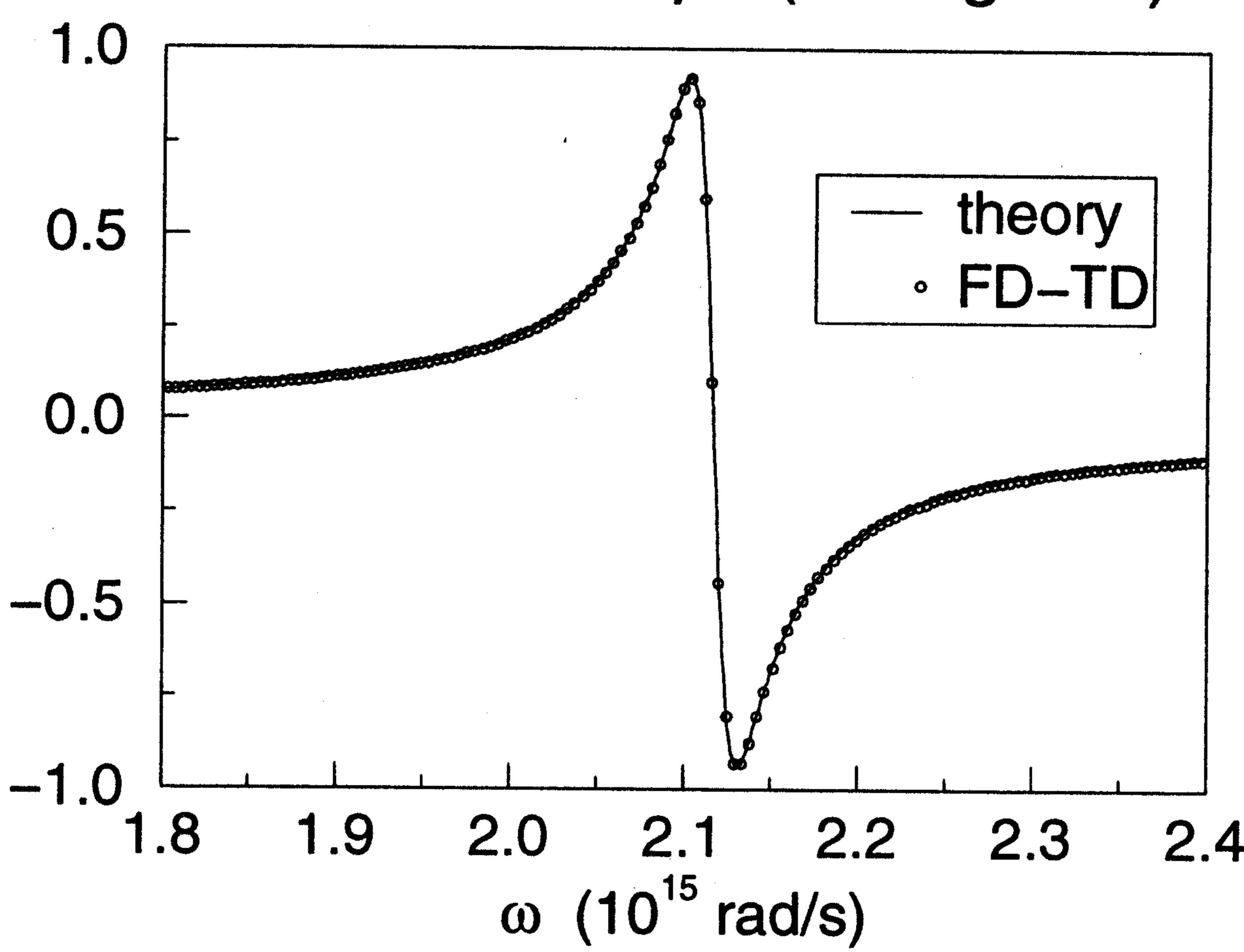
Figure 1. Comparison of finite difference time domain (FD-TD) results and theory for the amplification and phase factors of a pulse propagating a distance of one dielectric wavelength in a linear gain medium with  $\sigma_o = -5000$  mho/m.
