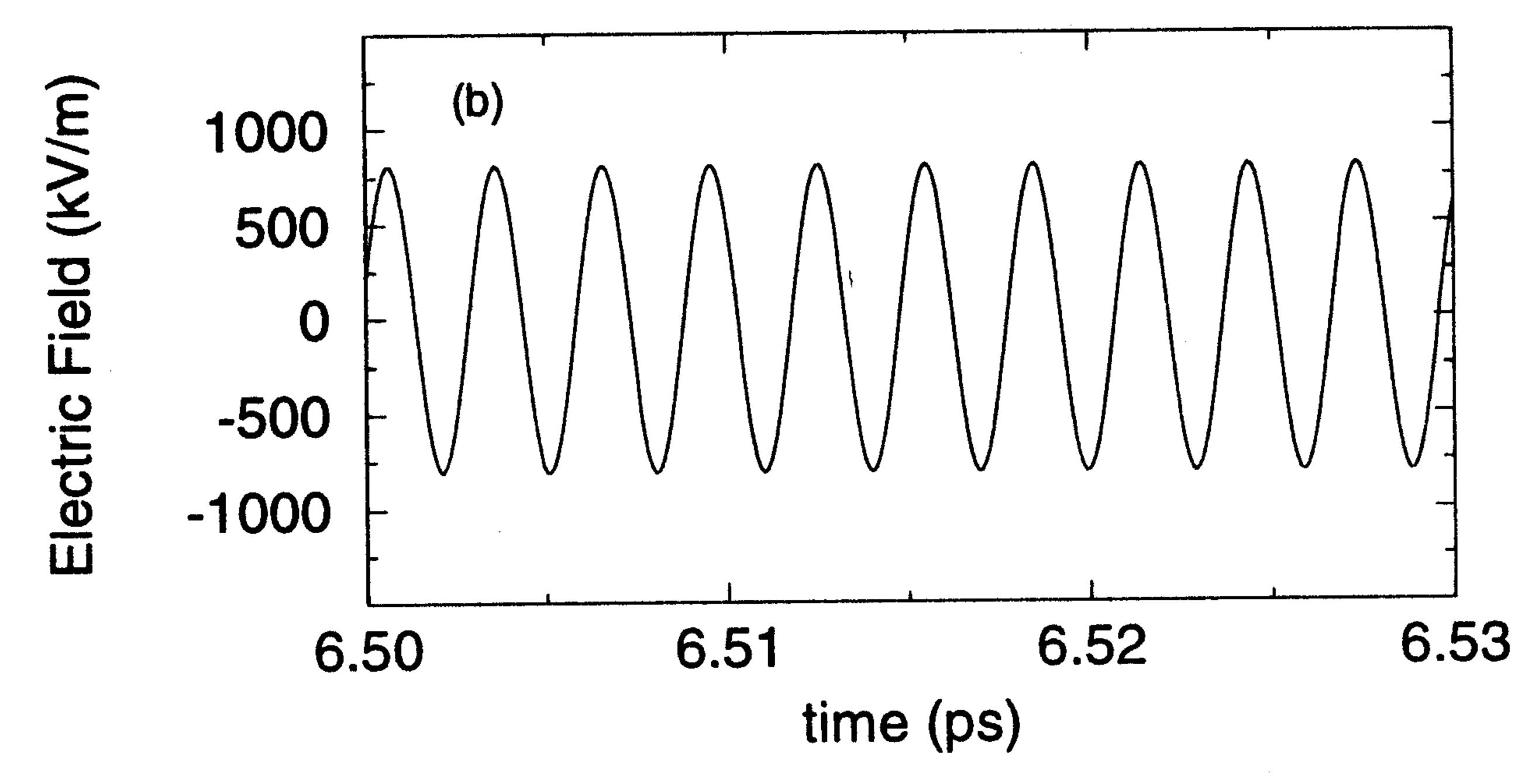
Figure 3. (a) FD-TD simulation of the time-varying electric field outside the Fabry-Perot laser cavity. (b) Expanded timescale of the steady state region showing single-mode oscillation at  $\omega_o$ .
