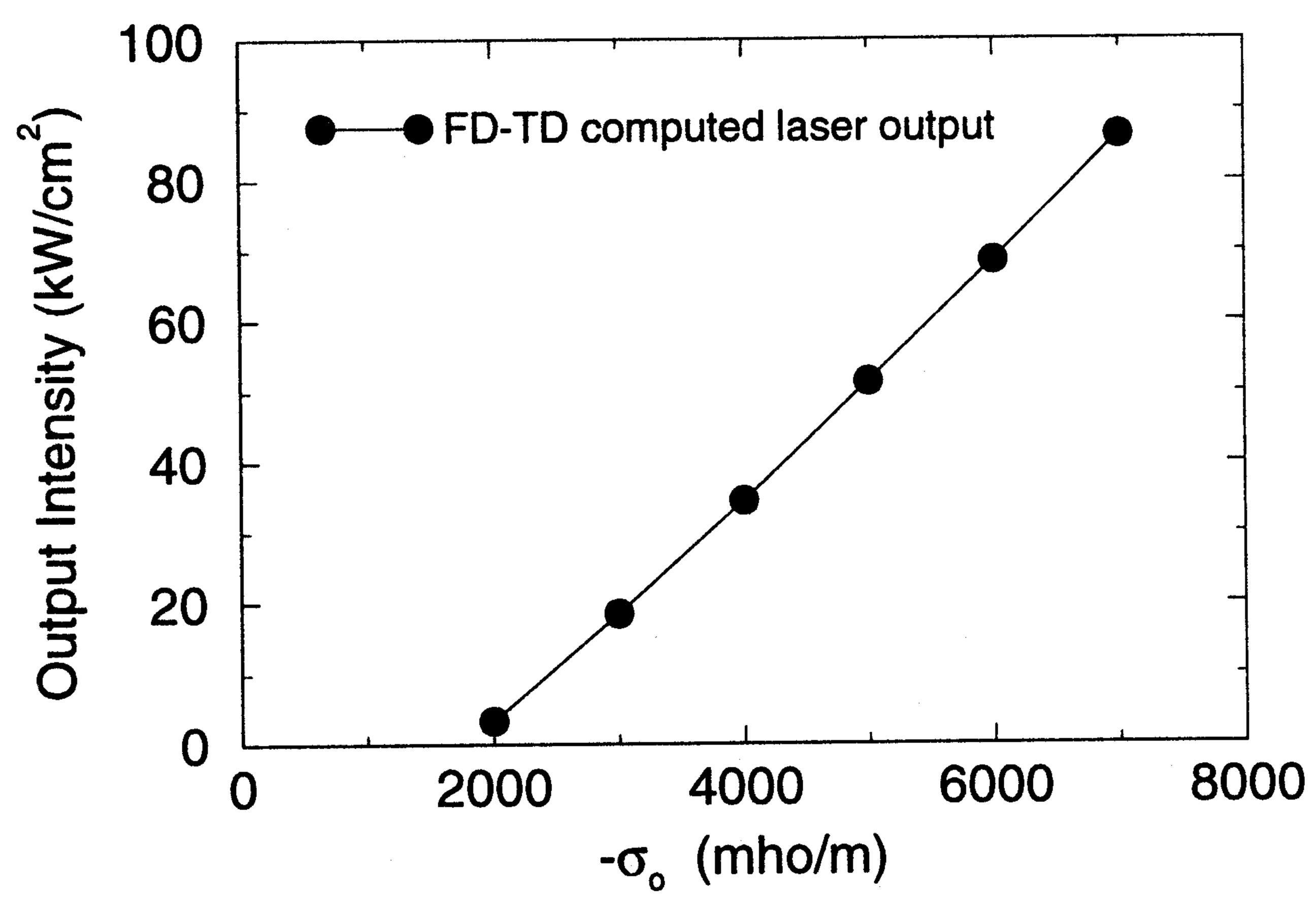
Figure 4. FD-TD computed light-current (L-I) curve for the output intensity of the Fabry-Perot laser.
