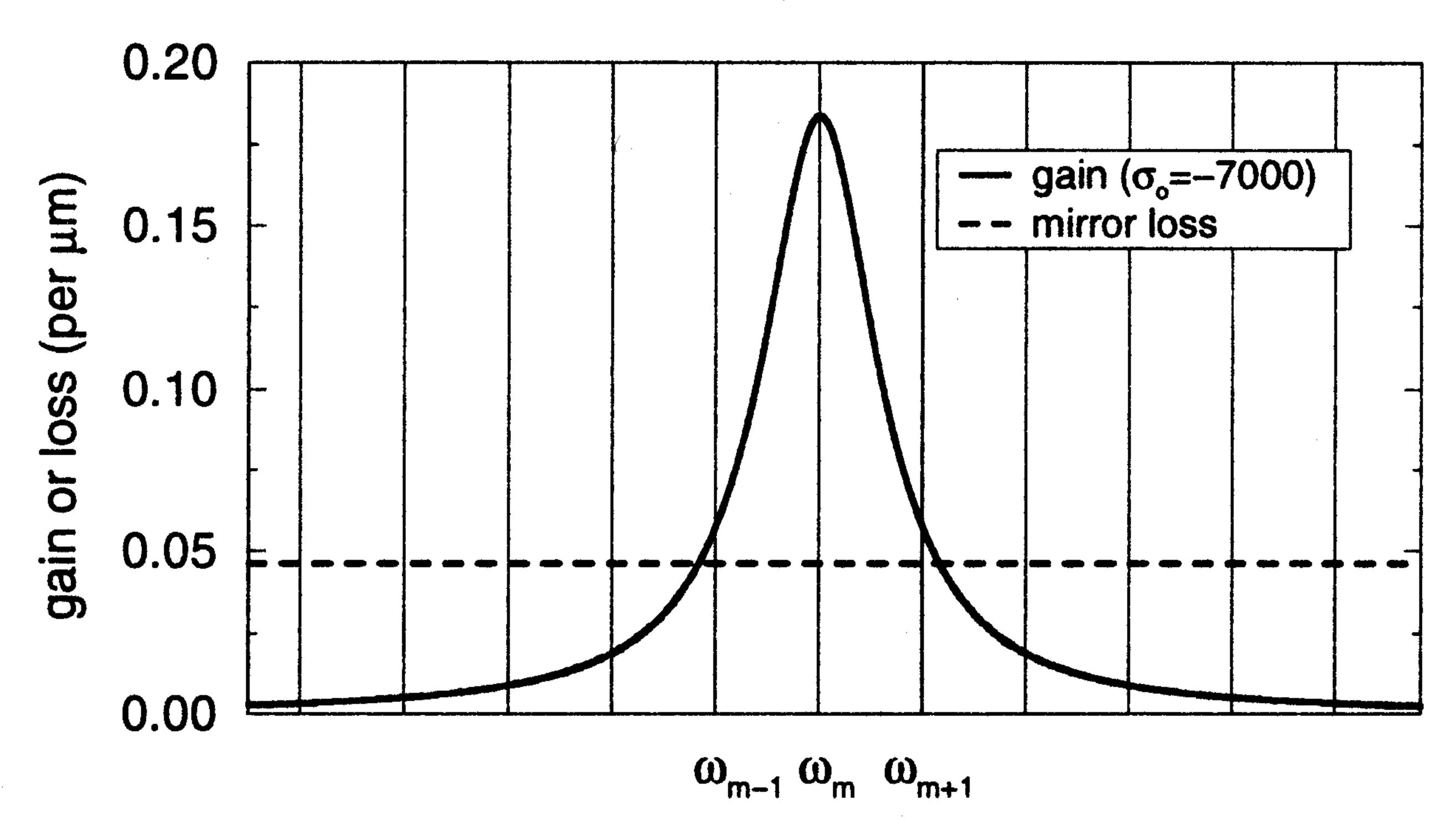
Figure 2. Unsaturated gain and loss spectra for a Fabry-Perot etalon with gain. The longitudinal modes of the Fabry-Perot cavity are shown as vertical lines.
