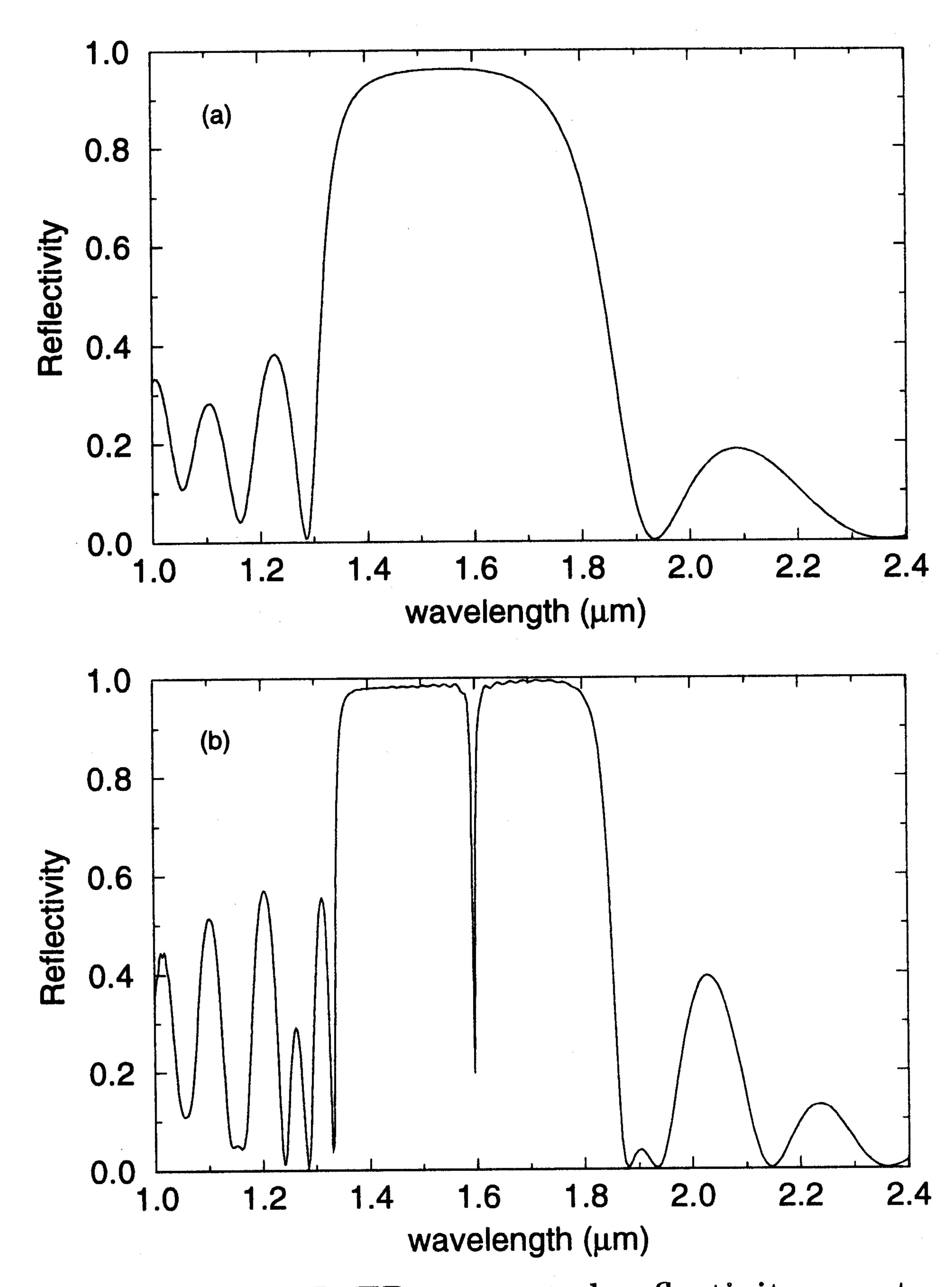
Figure 11. FD-TD computed reflectivity spectra for (a) a single photonic bandgap reflector composed of five periodically spaced air holes ( $\lambda_{\rm B} = 1.55~\mu{\rm m}$ ), and (b) a photonic-wire microcavity composed of two photonic bandgap reflectors separated by a length of  $0.525~\mu{\rm m}$ .
