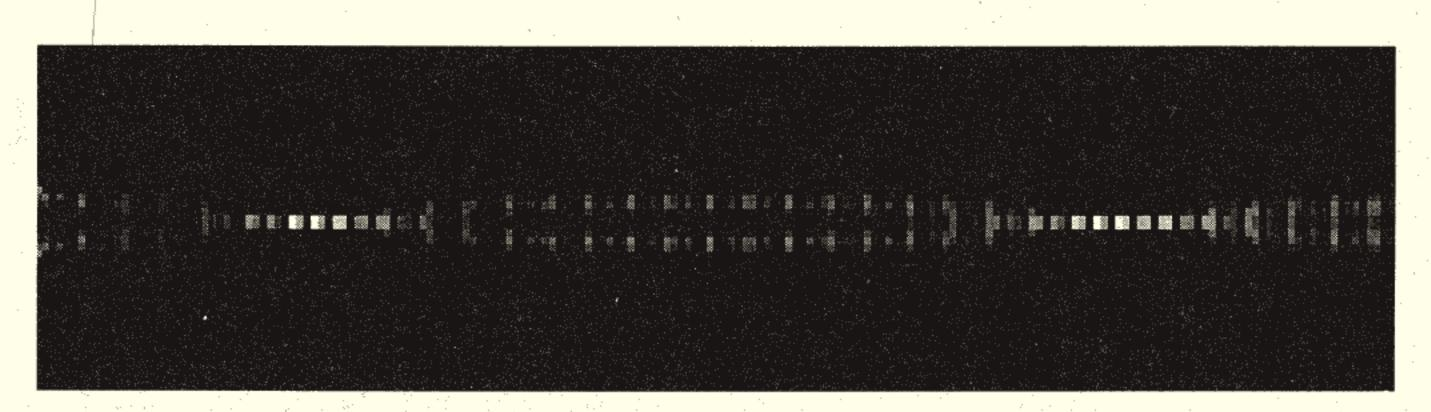
Fig. 2. FD-TD simulations showing restoration of the beam re-coalescence behavior after doubling the intensity beamwidth and separation parameters of the simulated beams, keeping the wavelength constant.
