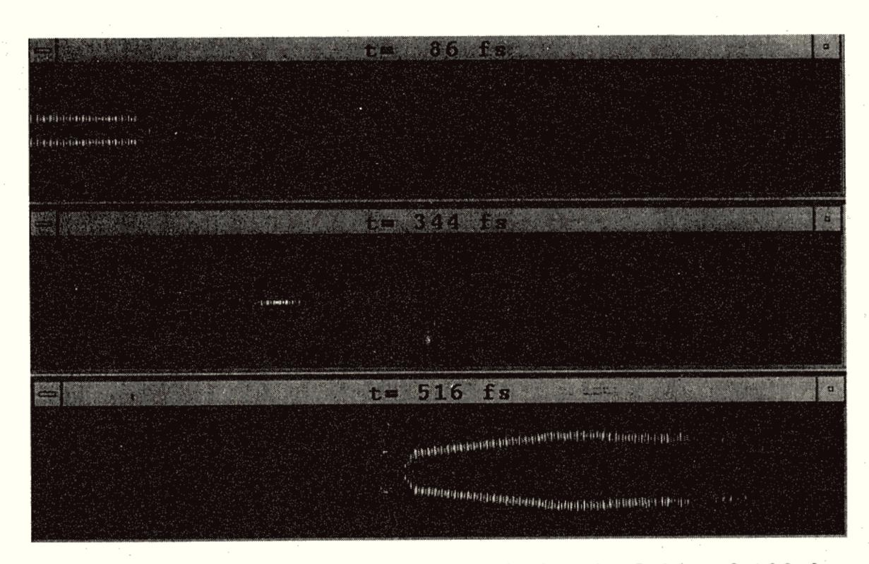
Fig. 4. Snapshots of the FD-TD-computed electric fields of 100-fs pulsed signal and control spatial solitons at the simulation times of 86 fs, 344 fs, and 516 fs for zero carrier phase between the pulses. Single-time spatial soliton coalescence behavior is indicated by FD-TD modeling for ultra-short pulses as well as continuous beams.
