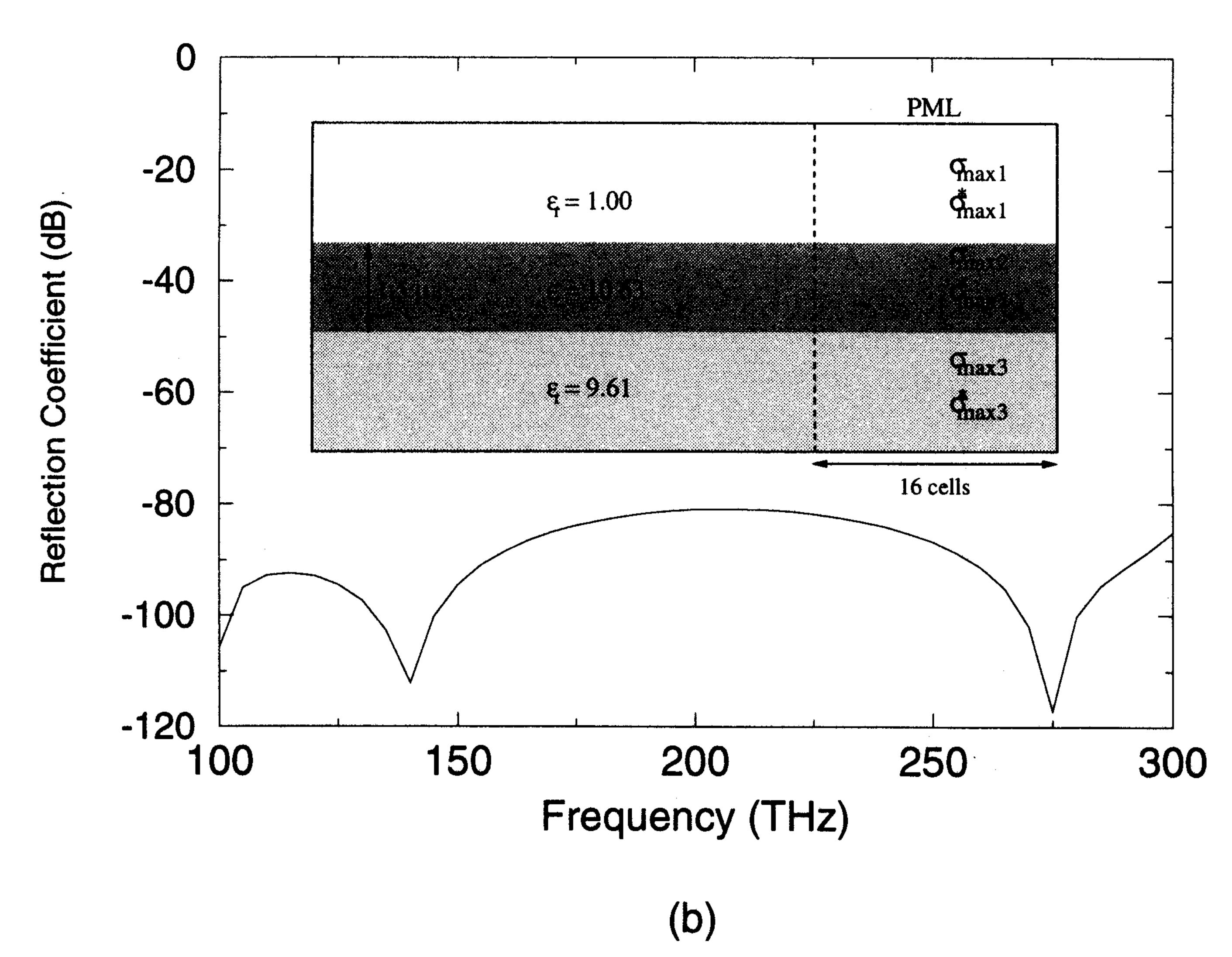
Fig. 2. Test of PML ABC for a 2-D asymmetric three-layer dielectric optical waveguide propagating three distinct modes: (a) Excitation spectrum superimposed upon the propagation factors for the three modes. (b) Waveguide/PML geometry and PML reflection coefficient versus frequency observed just outside the PML layer. Note that the substrate and air regions extend to infinity in the transverse direction, and that optical wave energy is present in all three regions.
