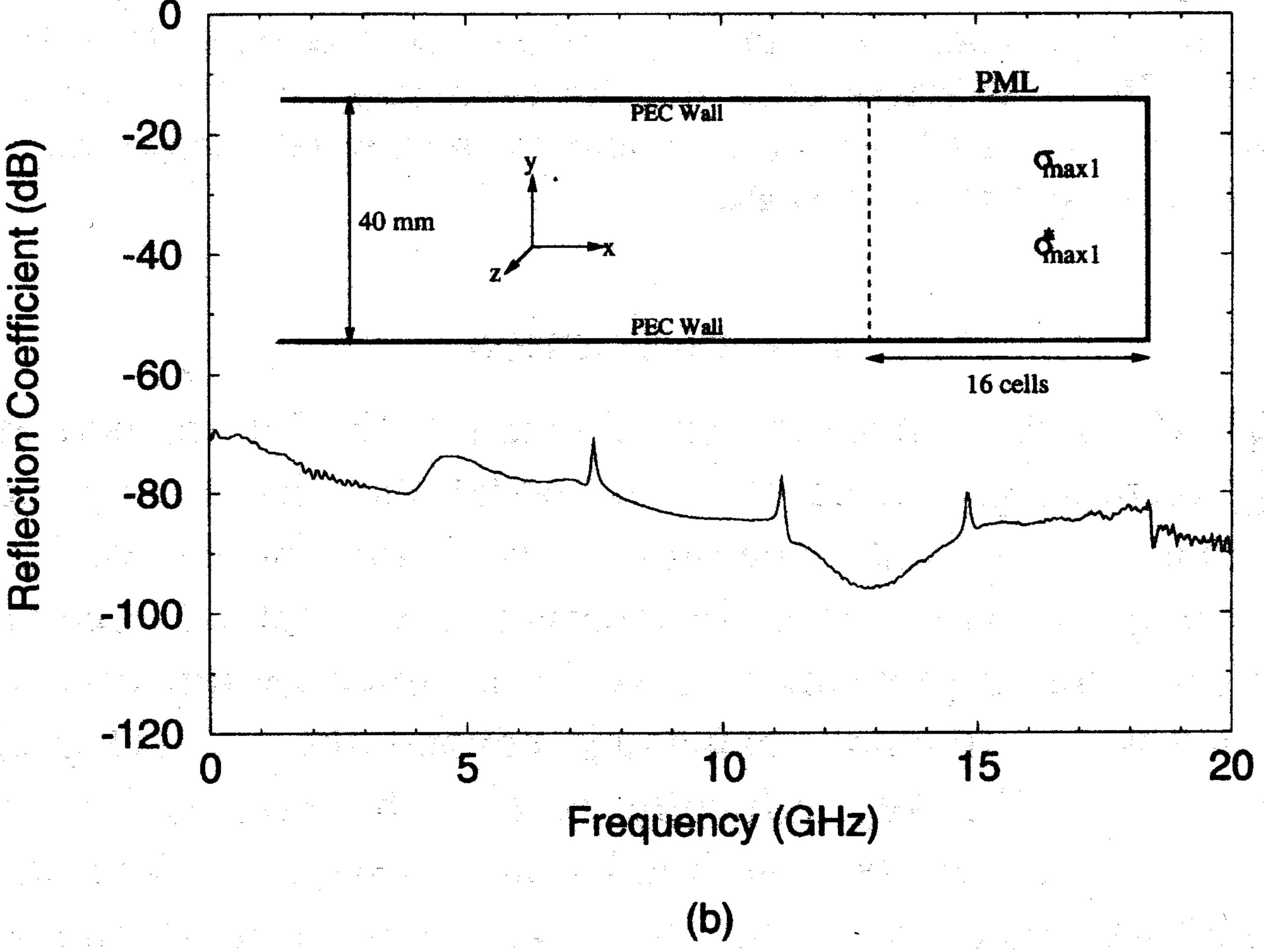
Fig. 1. Test of PML ABC for a 2-D PEC microwave waveguide propagating a pulsed  $TM_1$  mode: (a) Excitation spectrum superimposed upon the group velocity versus frequency function for the  $TM_1$  mode (cutoff frequency = 3.75 GHz). (b) Waveguide/PMLgeometry and PML reflection coefficient versus frequency observed just outside the PML layer.
