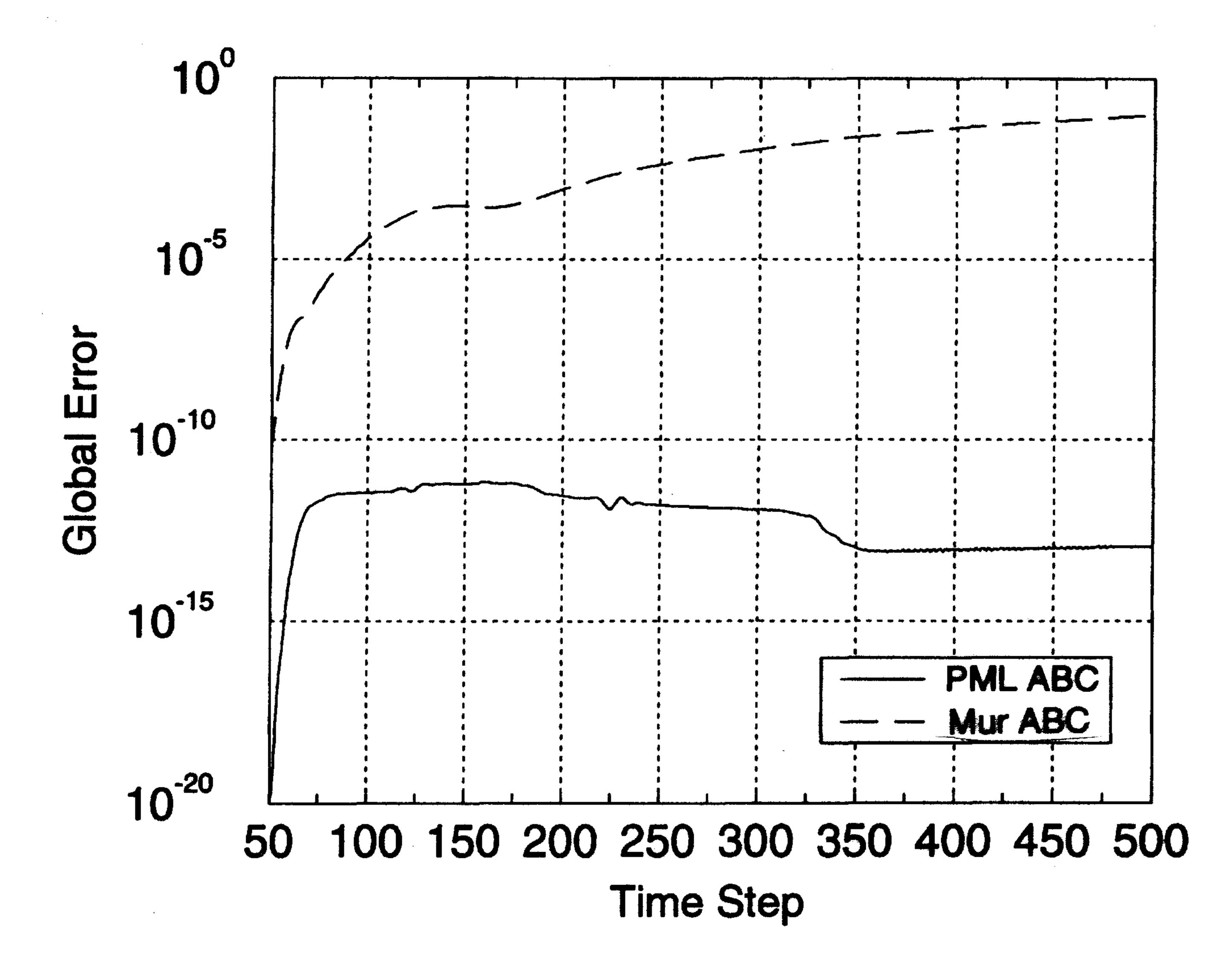
Fig. 1. Global error energy (square of the electric field error at each grid cell summed throughout the entire grid) within the  $100 \times 50$  cell 2-D TE FD-TD grid for both the second-order Mur ABC and the 16-cell-thick PML, plotted as a function of time step number on a logarithmic vertical scale.
