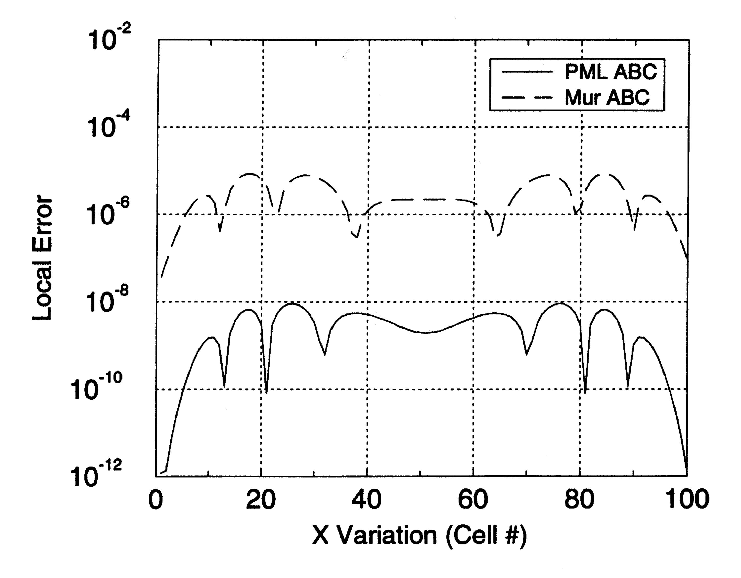
Fig. 2. Local electric field error along the x axis at the outer boundary of the  $100 \times 100 \times 50$  cell 3-D FD-TD grid for both the second-order Mur ABC and the 16-cell-thick PML, plotted on a logarithmic vertical scale (time step = 100).
