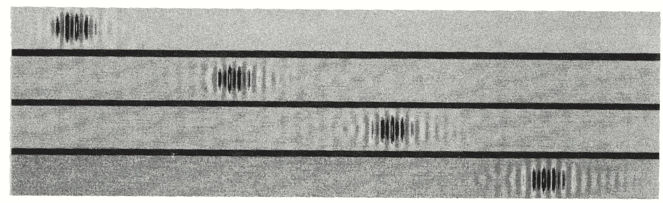
Fig. 2. Electric field of an optical soliton carrier pulse corresponding to that in Fig. 1, including quantum effects such as the Kerr and Raman interactions.
