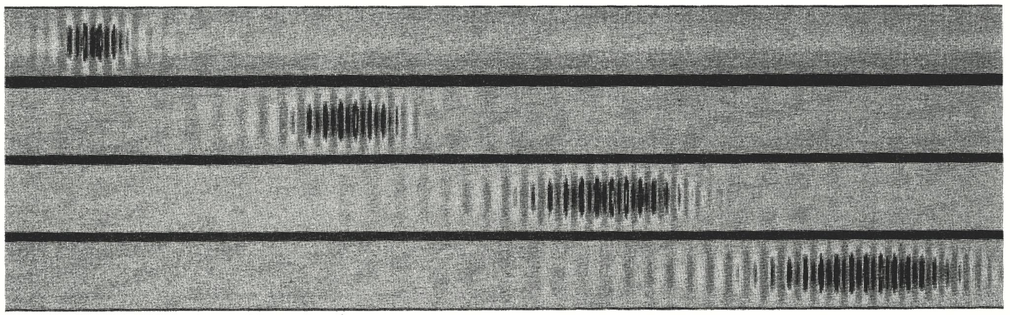
Fig. 1. Electric field of a propagating optical carrier pulse with initial hyperbolic-secant envelope ( $\lambda = 2.19 \ \mu m$ ,  $\tau = 14.6 \ fs$ ) in a 1- $\mu m$ -thick linear Lorentz-medium dielectric waveguide.
