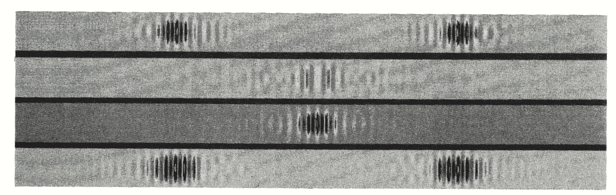
Fig. 3. Electric field of colliding counterpropagating solitons corresponding to that in Fig. 2 (approaching, destructively interfering, constructively interfering, separating).
