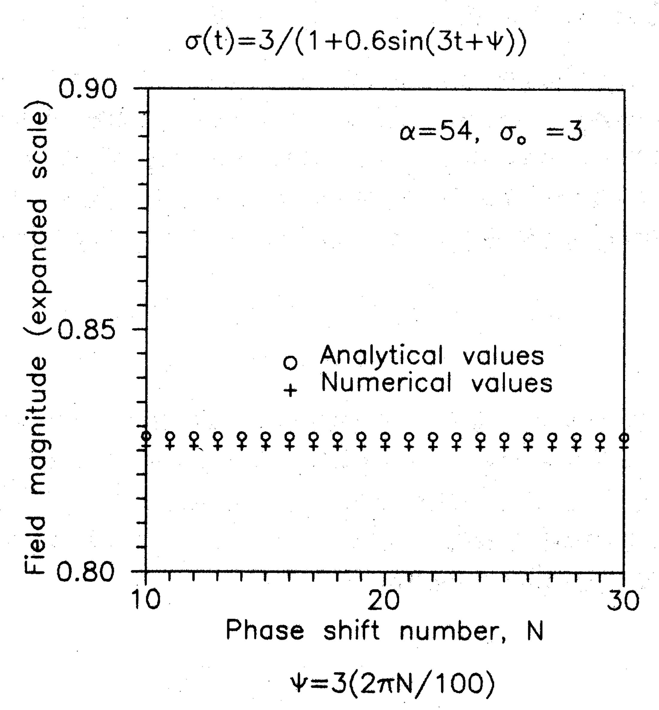
Fig. 4. Reflected field amplitude at illumination frequency versus initial phase as obtained both asymptotically and by FDTD for  $\nu = 3$ ,  $\sigma_0 = 3$ , and  $\alpha = 54$ .
