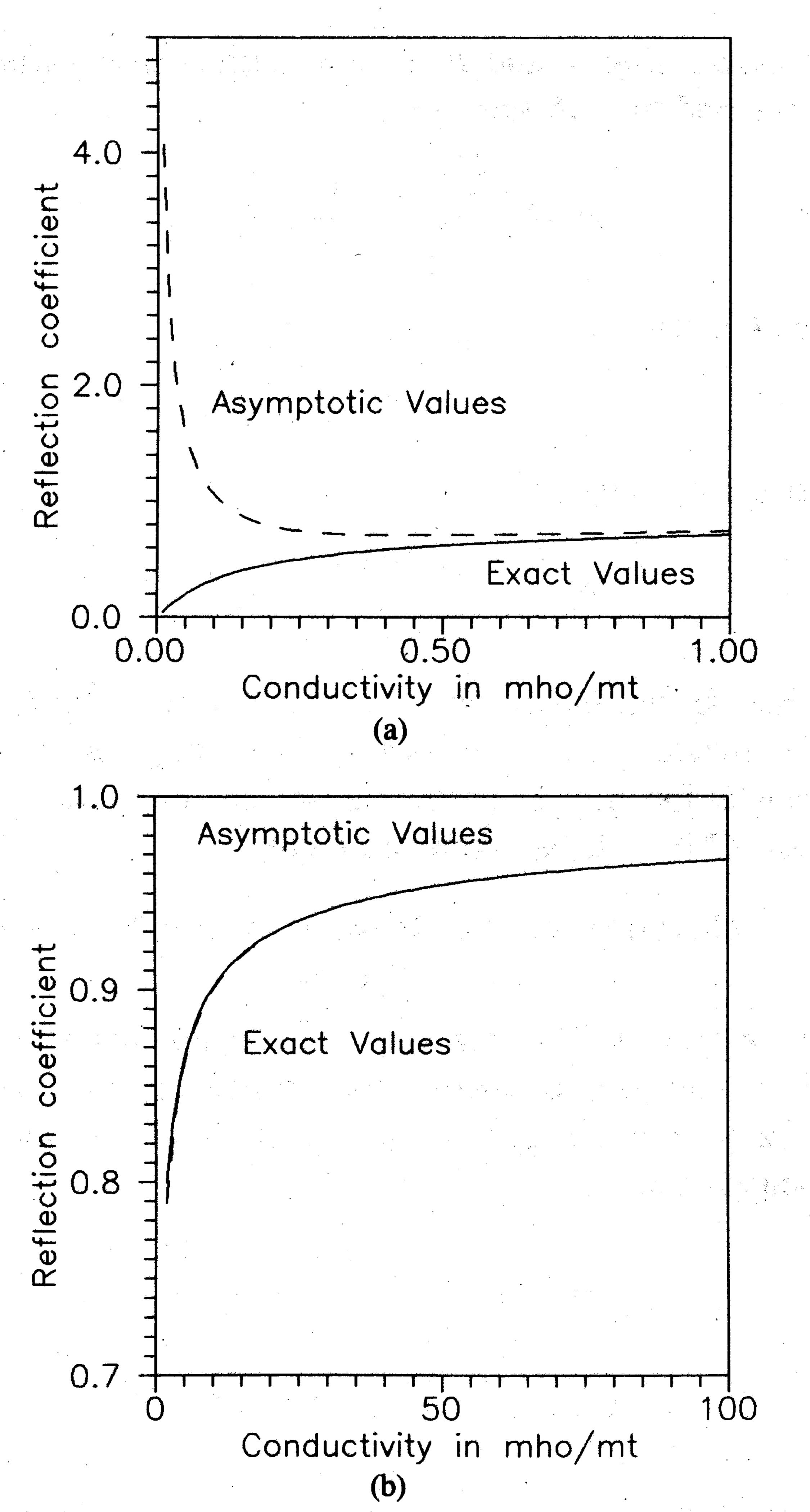
Fig. 9. Variations of the reflected field amplitude versus fixed conductivity  $\sigma_0$  as obtained both exactly and asymptotically.
