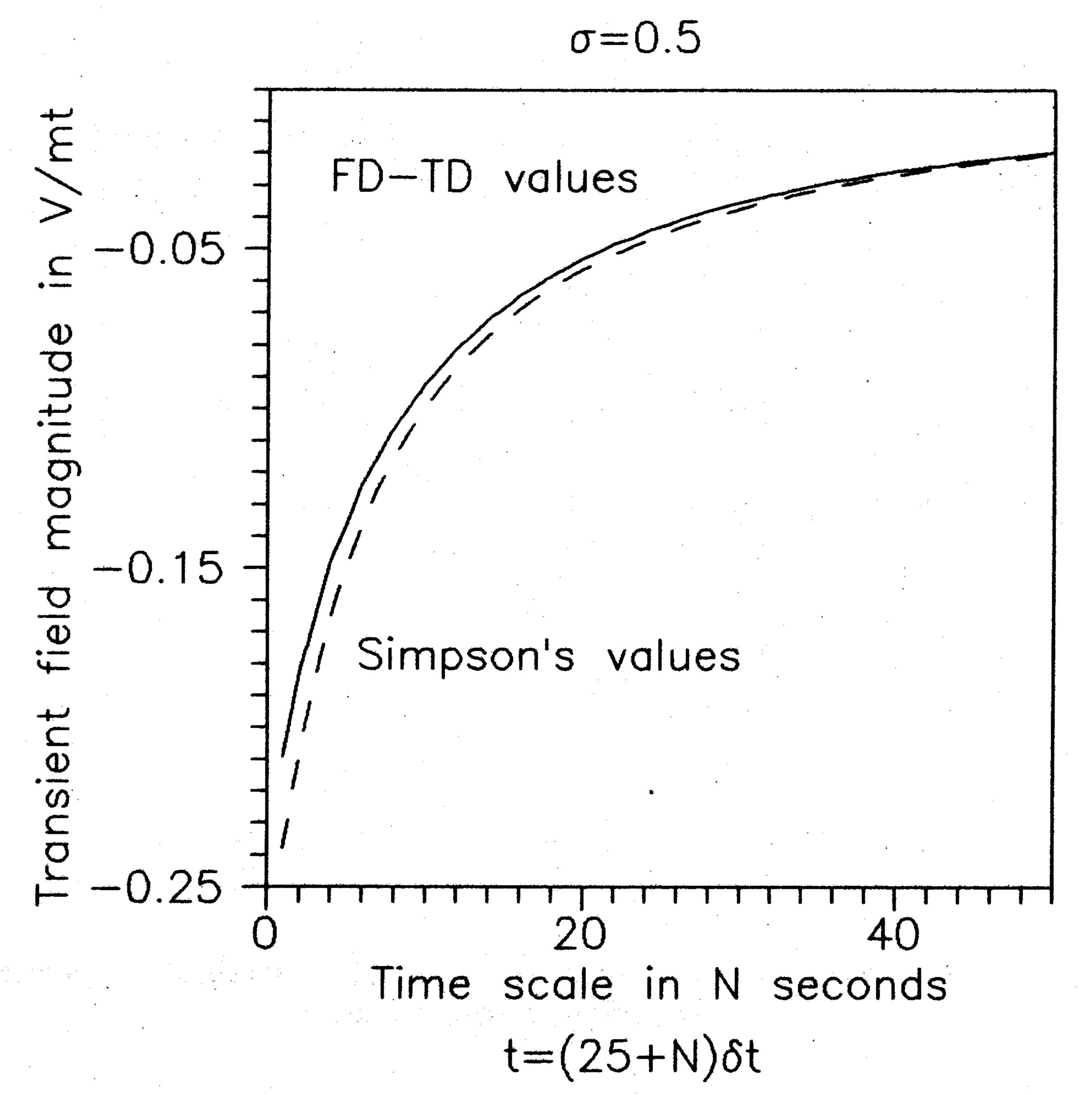
Fig. 10. Transient response in the reflected field from a material with a constant conductivity  $\sigma_0$  as obtained by numerical integration and FDTD.
