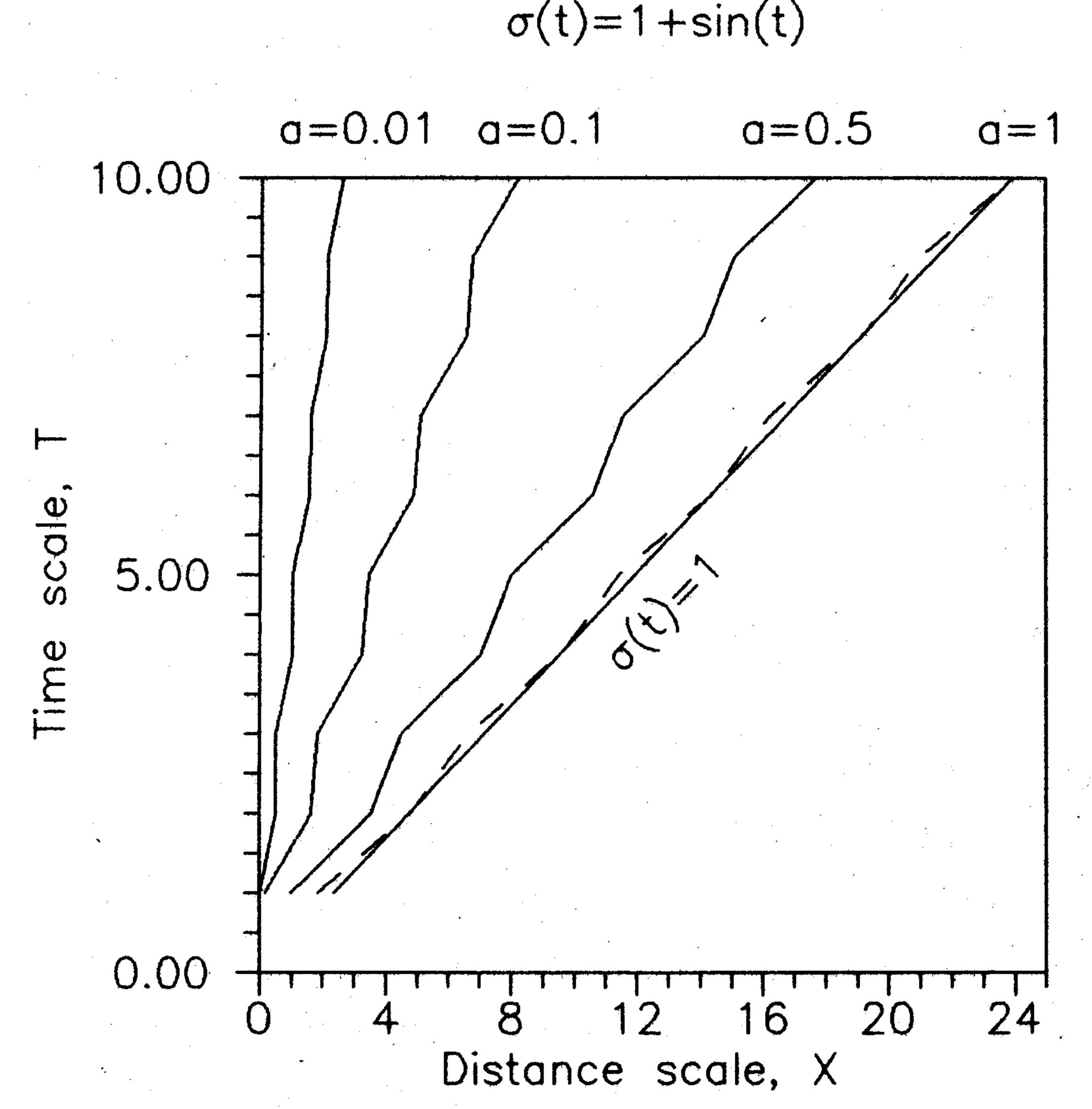
Fig. 8. Rays tracing in (x, t) space for a given time-modulated conductivity and different firing angles.
