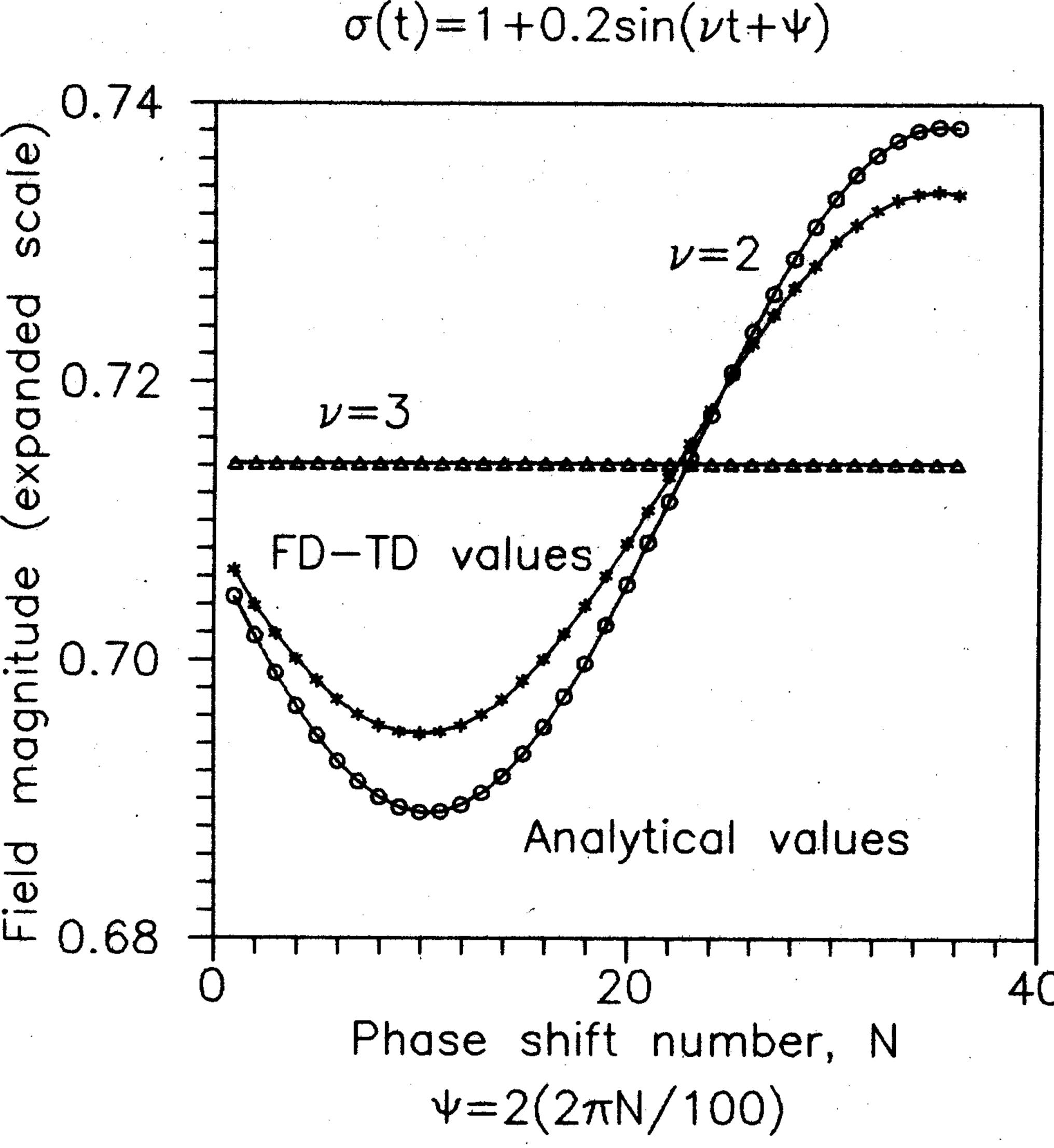
Fig. 2. Reflected field amplitude at the illumination frequency versus the initial phase shift  $\phi$  as obtained both by FDTD and the first-order perturbation analysis.
