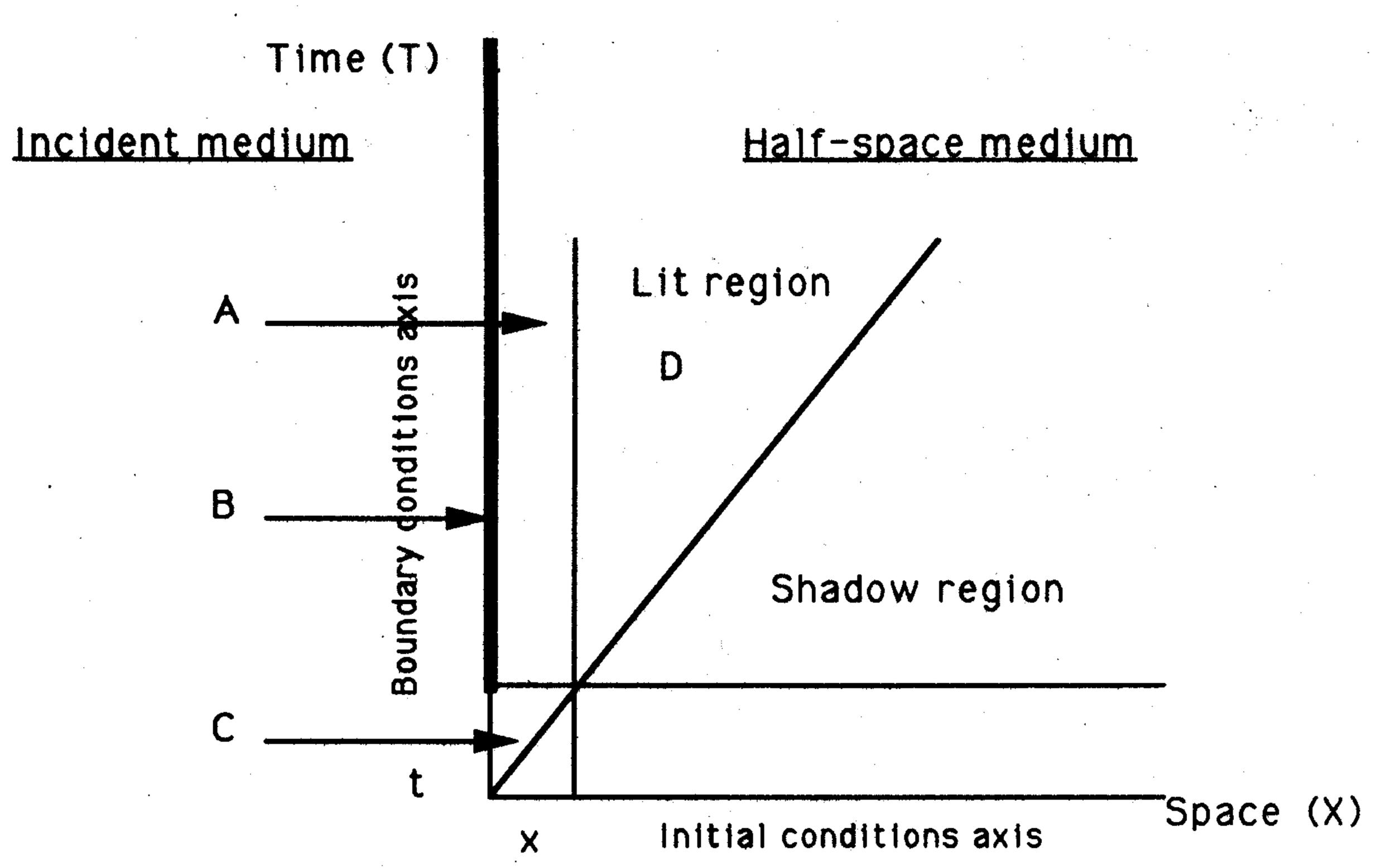
Fig. 7. Boundary-layers in a media with a time-varying conductivity. A: Diffusion solution, B: oscillating solution, C: propagating solution, D: large parameter solution.
